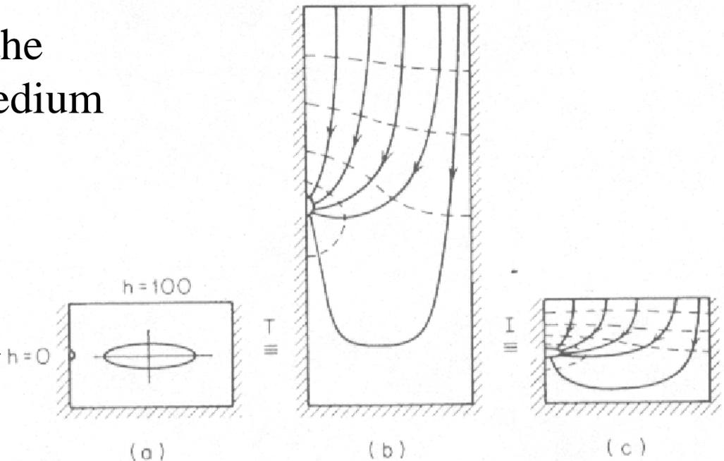
Figure 5.8 (a) Flow problem in a homogeneous anisotropic region with  $\sqrt{K_x}/\sqrt{K_z} = 4$ . (b) Flow net in the transformed isotropic section. (c) Flow net in the actual anisotropic section.  $T$ , transformation;  $I$ , inversion.
