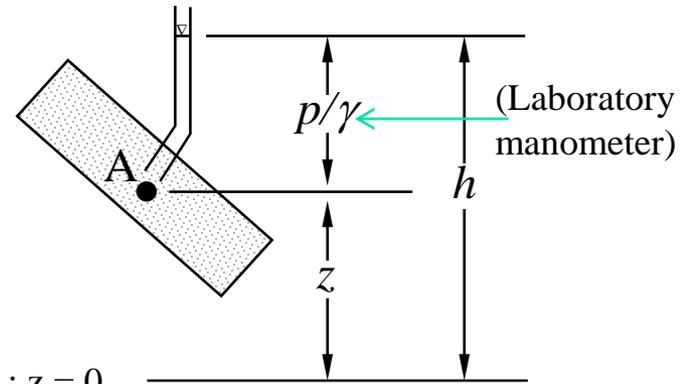
Schematic of hydraulic head, pressure head, and elevation (potential) head
