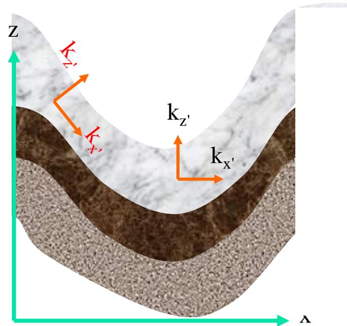
A global coordinate system (x-z) is defined. Local coordinates (x'-z') are aligned with the principal directions of the local hydraulic conductivity tensor.
