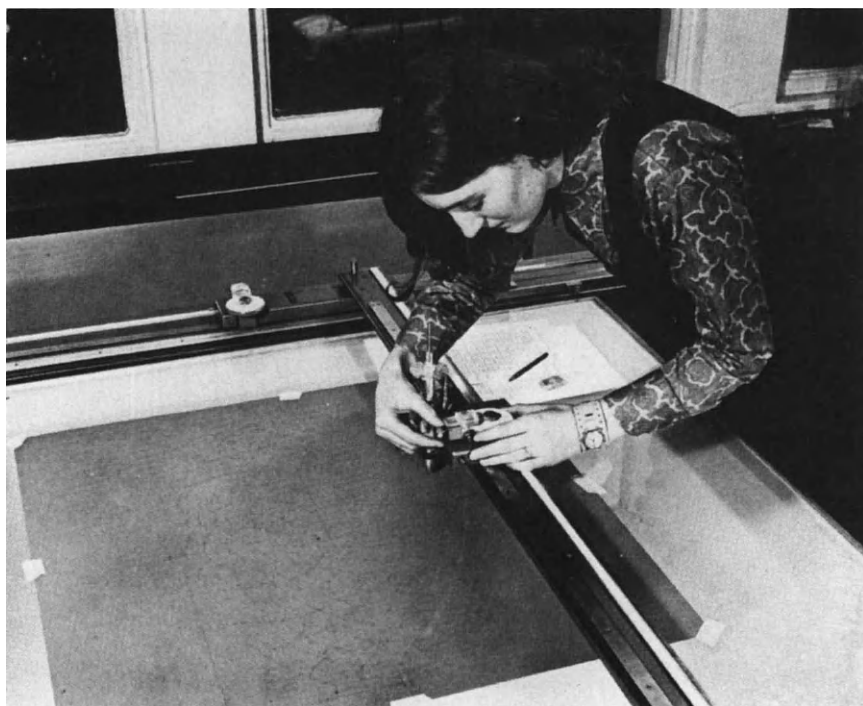
Plate 1 Coradi coordinatograph with effective plotting dimensions 1000 mm. in both x and y.
