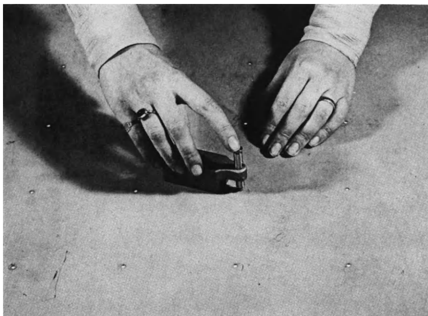
Plate 2 Haag-Streit Master Grid Template with effective plotting dimensions 1000 \times 700 mm. and holes at 100 mm. intervals.
