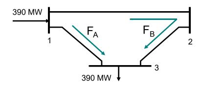
$F_A$  = 2 x  $F_B$  because the path 1-2-3 has twice the reactance of the path 1-3
