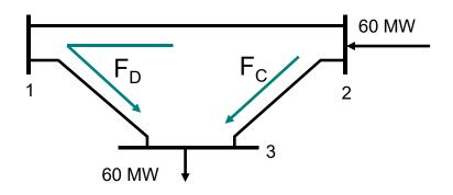
$F_C$  = 2 x  $F_D$  because the path 2-1-3 has twice the reactance of the path 2-3
