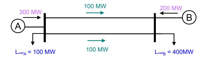
In this simple case, the solution of the economic dispatch can be modified easily to produce acceptable flows.
