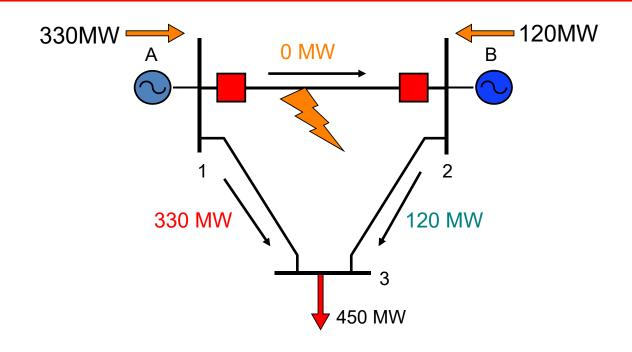
Unacceptable because overload of line 1-3 could lead to a cascade trip and a system collapse
