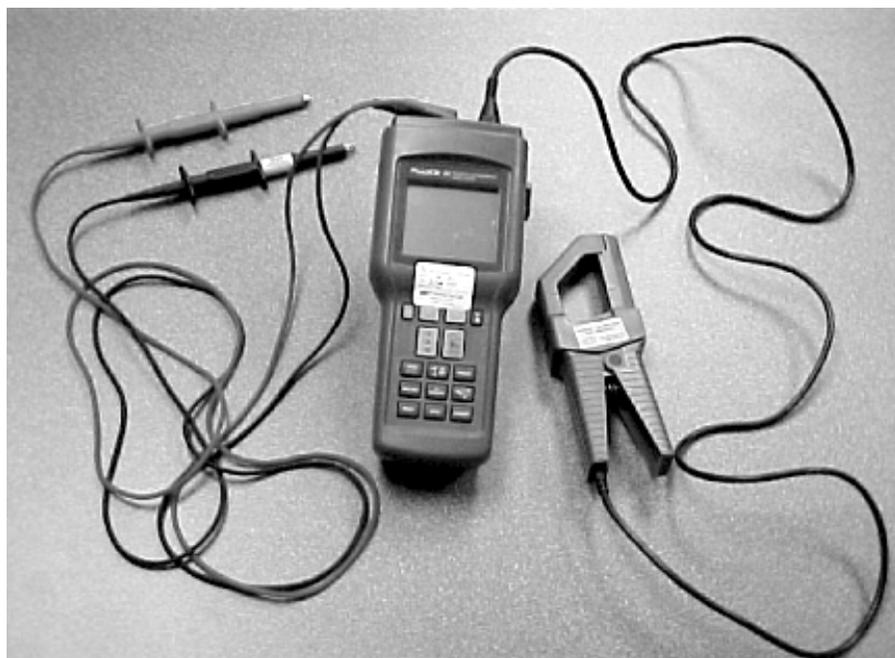
**FIGURE 9.2** Handheld harmonic analyzer showing voltage leads and current probe for voltage and current harmonic measurements. (Photograph courtesy of Fluke.)
