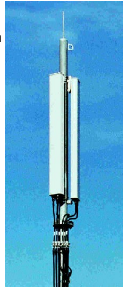
X-polarization diversity, 2RX, 1 TX per sector, duplexer
