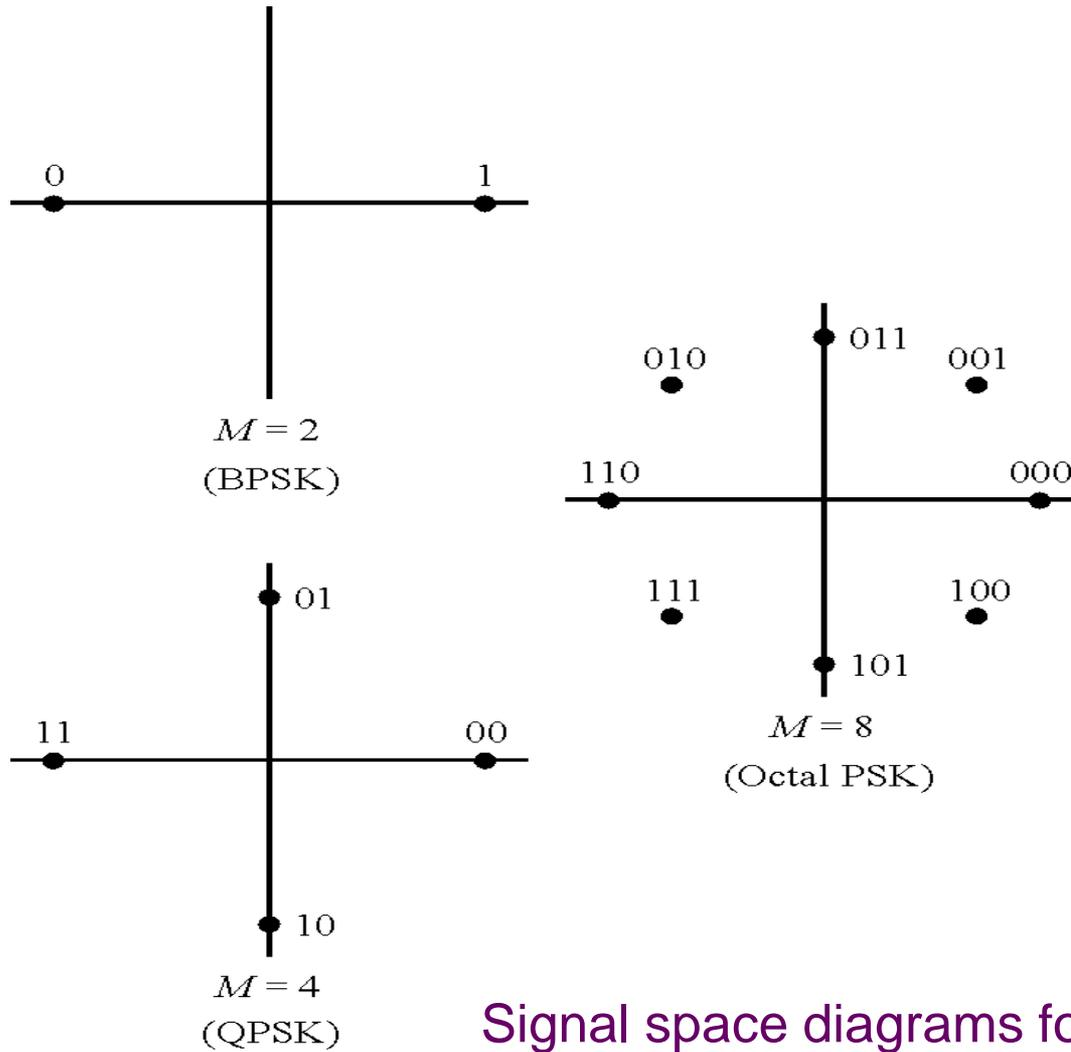
Signal space diagrams for PSK signals
