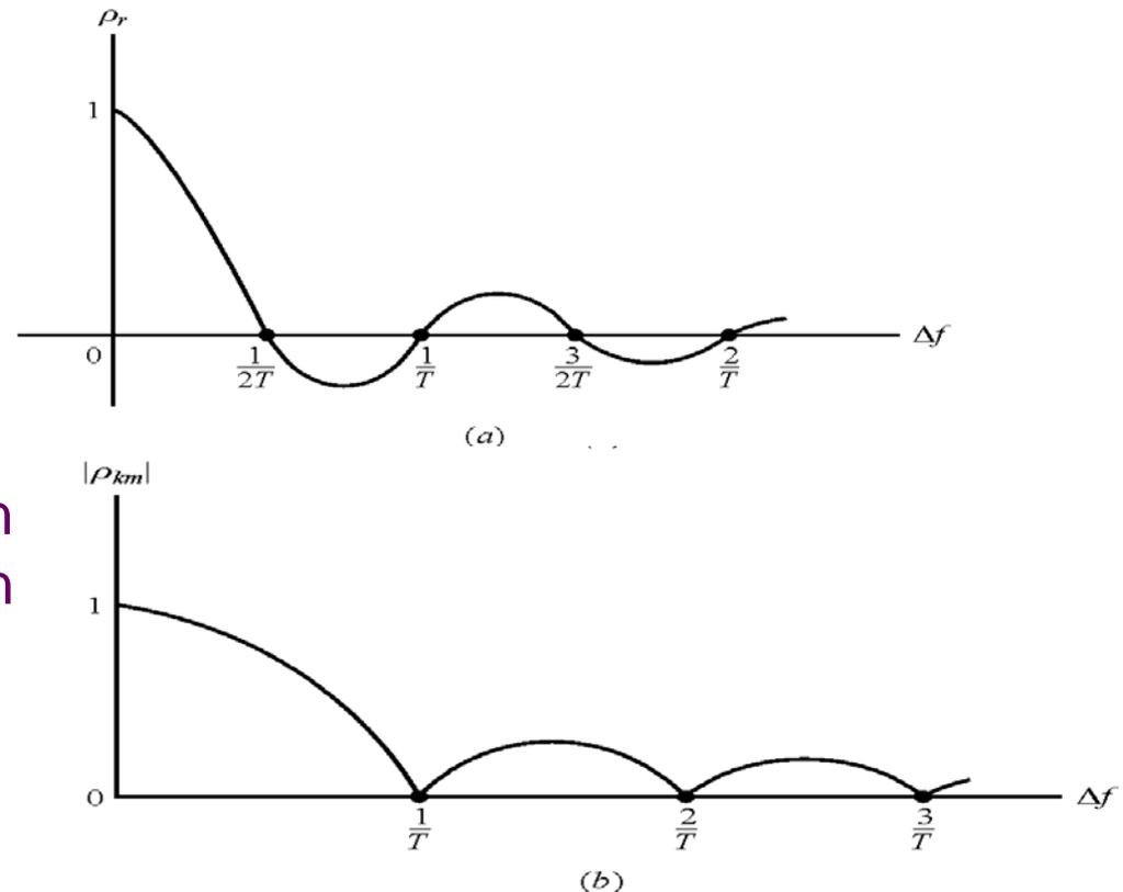
Cross-correlation coefficient as a function of frequency separation for FSK signals
