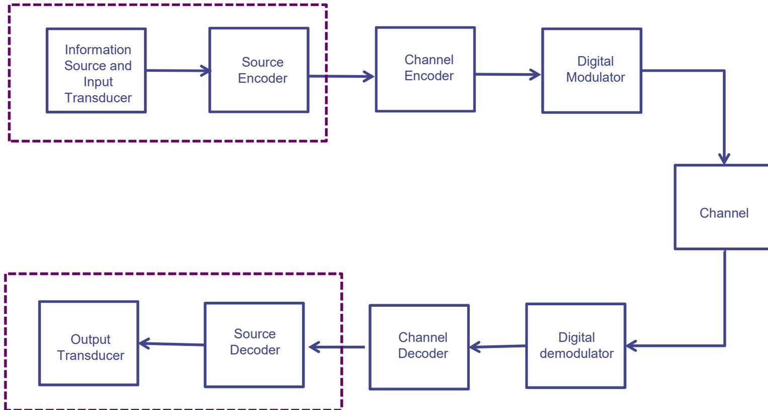
Functional block diagram of a typical digital communication system
