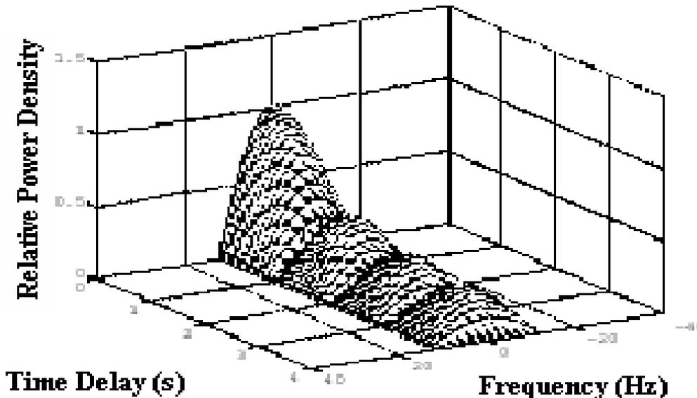
Example of Scattering function of Time Varying Channel
