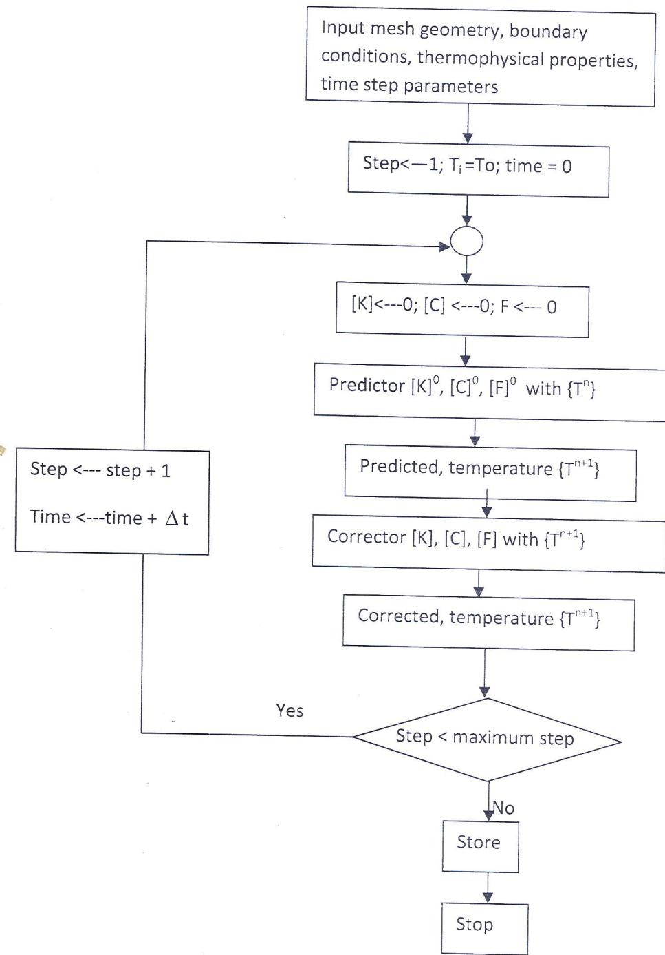
Fig.2 Flow chart for solutions of non linear transient heat conduction problem with predictor correction algorithm
