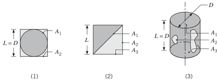
1. Sphere of diameter  $D$  inside a cubical box of length  $L = D$ .
