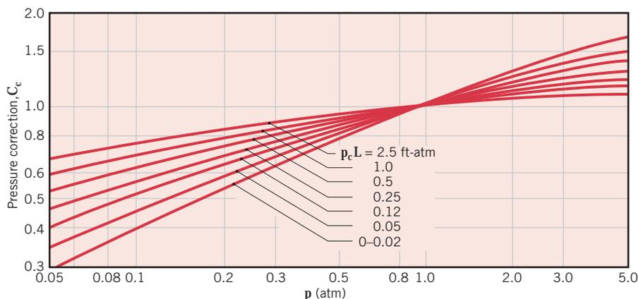
**FIGURE 13.18** Correction factor for obtaining carbon dioxide emissivities at pressures other than 1 atm ( $\epsilon_{c,p \neq 1 \text{ atm}} = C_c \epsilon_{c,p=1 \text{ atm}}$ ) [13]. Used with permission.
