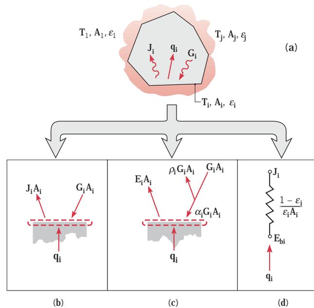
**FIGURE 13.8** Radiation exchange in an enclosure of diffuse, gray surfaces with a nonparticipating medium. (a) Schematic of the enclosure. (b) Radiative balance according to Equation 13.9. (c) Radiative balance according to Equation 13.11. (d) Network element representing the net radiation transfer from a surface.
