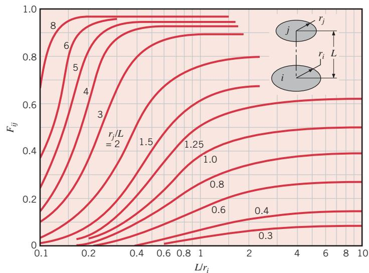
**FIGURE 13.5** View factor for coaxial parallel disks.
