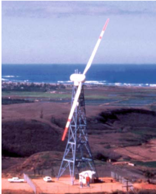
1.3. The MOD OA wind turbine (Courtesy of Hawaiian Electric Company, Inc., http://heco.com )
