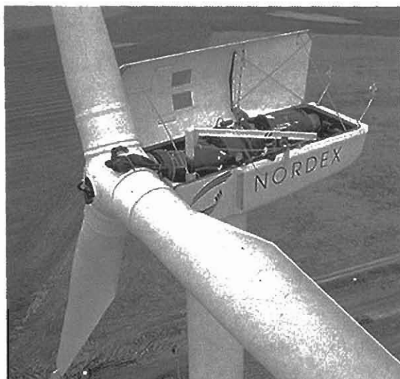
Figure 6.38 Typical nacelle cover. Reproduced by permission of Nordex AG
