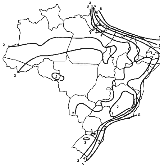
Figure 2.32 Annual average wind speeds for Brazil (m/s) (Rohatgi and Nelson, 1994). Reproduced by permission of Alternative Energy Institute
