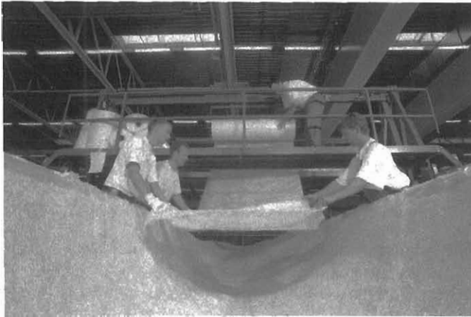
Figure 6.17 Laying fiberglass cloth into blade molds. Reproduced by permission of LM Glasfibre
