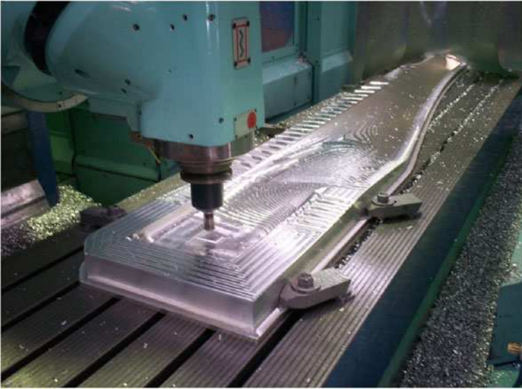
Fig. 7.10 Machining the mould for the lower surface of the 2.5 m long blade in Fig. 7.6
