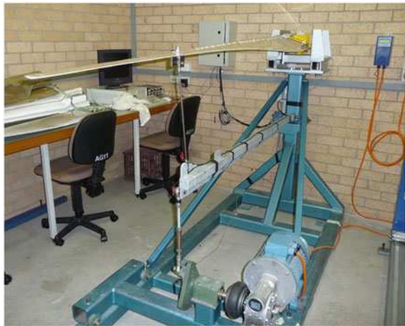
Fig. 7.14 The 2.5 m long blade from Fig. 7.6 in the fatigue test rig at the University of Newcastle
