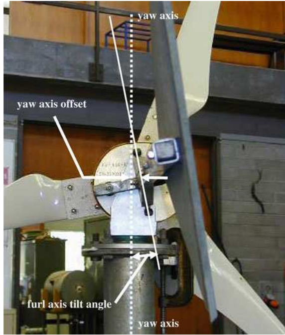
Fig. 8.14 Close up of 500 W turbine furling mechanism. Photo from Wright [21]
