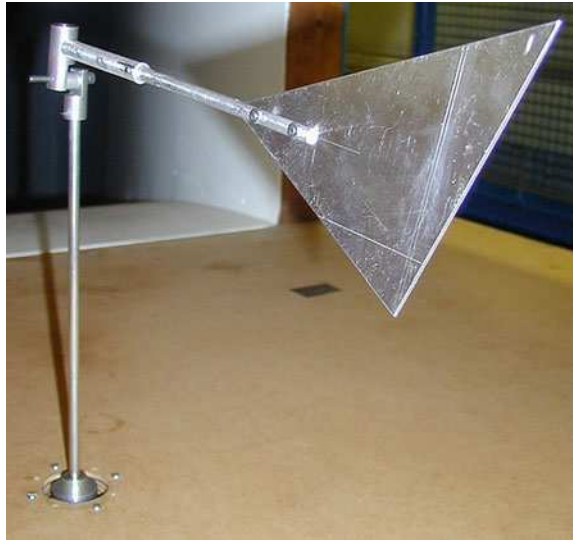
Fig. 8.5 Wind tunnel testing of a 1/4 scale model of the tail fin in Fig. 6.1. The vertical shaft has an encoder to measure angle. From Wright [21]
