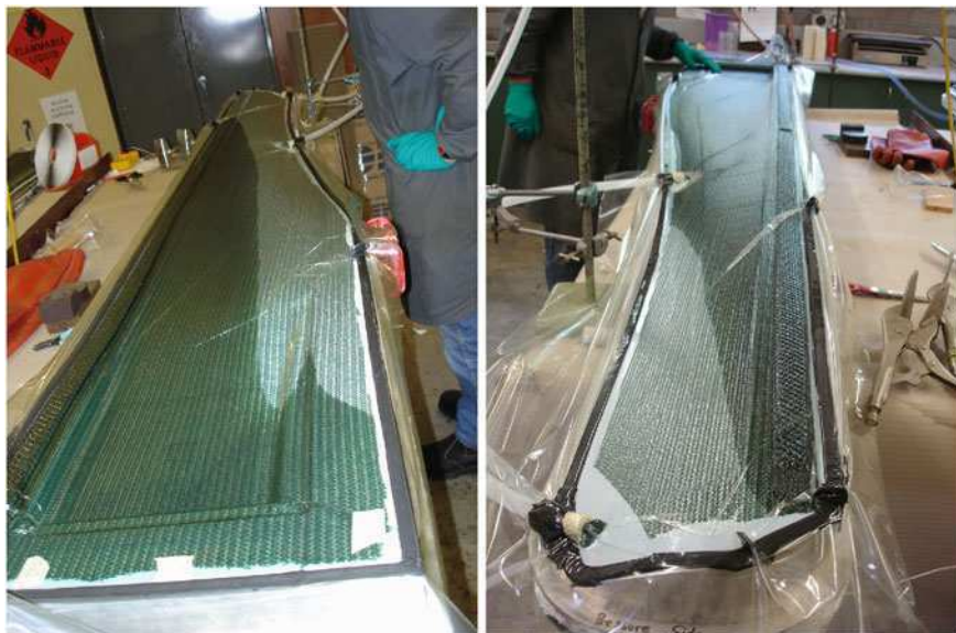
Fig. 7.11 Vacuum infusion of the lower half of a 2.5 m long blade. Left side view from hub end, right side from the tip
