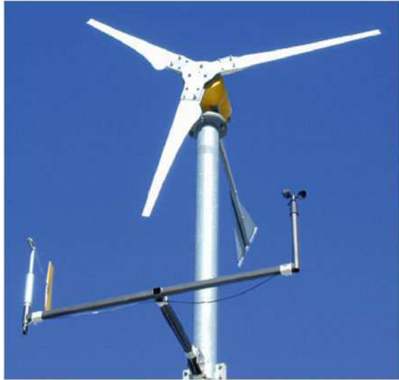
Fig. 6.1 500 W 1.94 m diameter turbine with cup anemometer and wind vane
