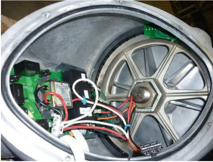
Fig. 1.10 Inside the nacelle of the Skystream 2.4 kW wind turbine
