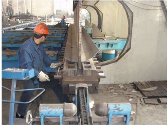
Fig. 10.1 Bending half an octagonal tower section at a factory in China
