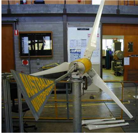
Fig. 8.13 Rear view of the 500 W turbine showing tail fin. Photo from Wright [21]
