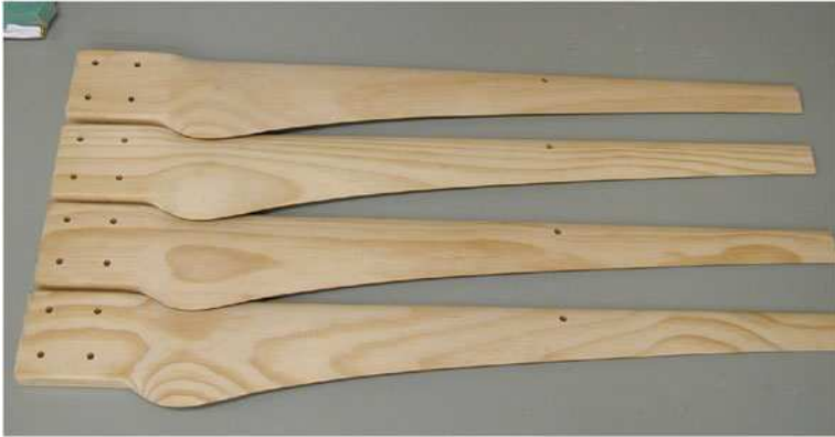
Fig. 7.7 Machined 0.87 m long timber blades for the turbine in Fig. 6.1. These blades have holes at the 2/3 radius point for static and fatigue testing
