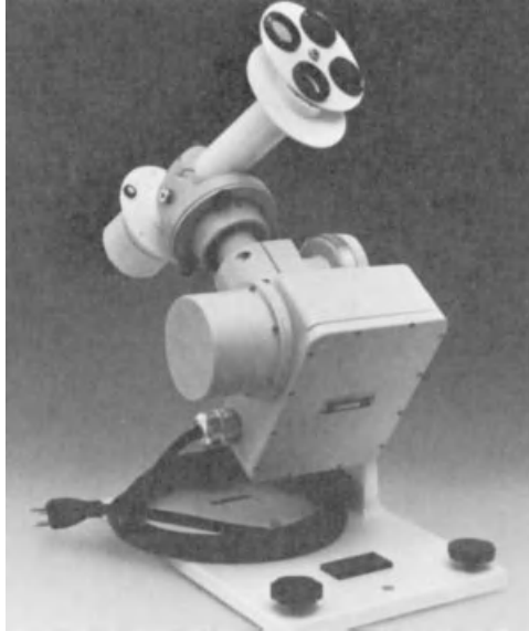
Figure 2.2.3 An Eppley NIP on an altazimuth tracking mount. Courtesy of The Eppley Laboratory.
