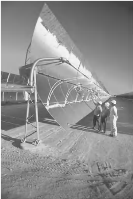
Figure 17.3.3 (b) Individual collector.
