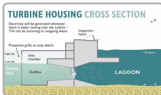
Fig. 18.9. Diagram of the tidal lagoon.
