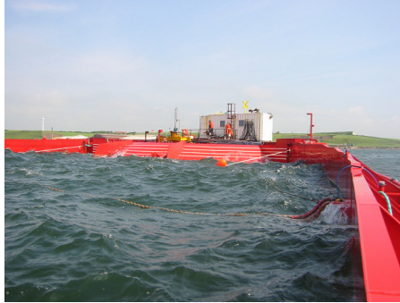
Fig. 18.4. Wave Dragon seen from reflector, prototype 1:4½.
