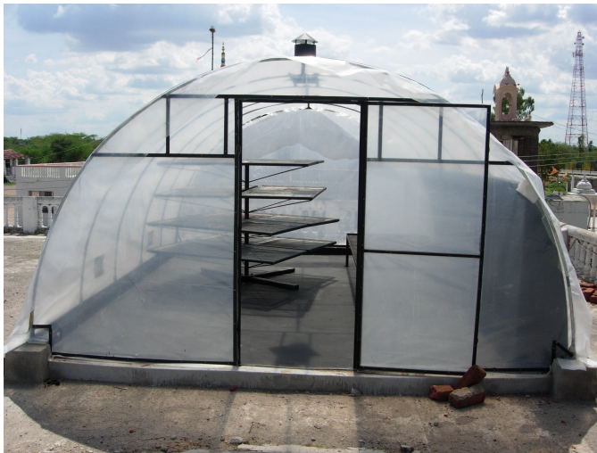
Fig. 13.6. Closed view of solar tunnel dryer installed at M/s Shrinath Aonla's Farm.
