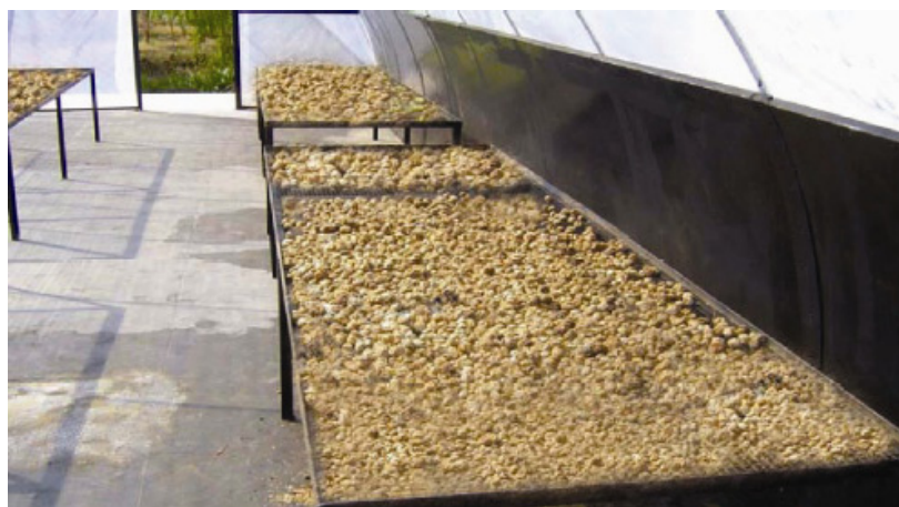
Fig. 13.7. Inside view of solar tunnel dryer for drying foremblica officinalis pulp.
