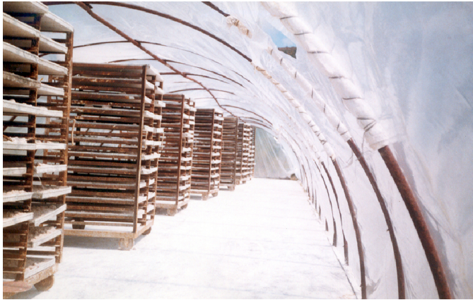
Fig. 13.17. Inside view of solar tunnel dryer under full load condition for drying of di-basic calcium phosphate.
