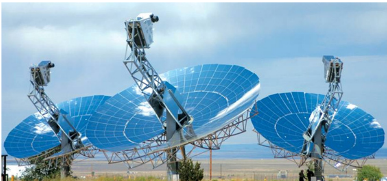
Fig. 10.19. Solar dish Stirling system (courtesy of Stirling Energy Systems, Inc.).
