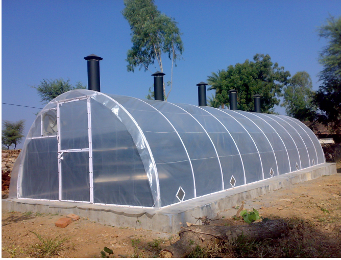
Fig. 13.16. Closed view of the solar tunnel dryer installed at the factory site for drying of di-basic calcium phosphate.
