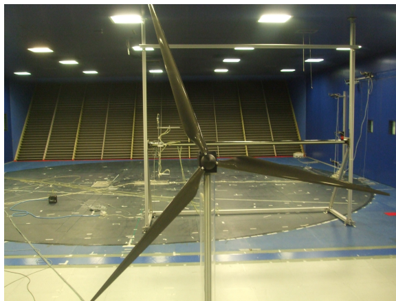
Fig. 7.19. The Milan Polytechnic wind tunnel and the model turbine.
