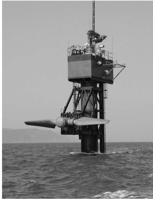
Figure 16.7 Prototype of a tidal turbine installed off the Coast of Devon, England. The rotor/turbine assembly is shown in the raised position for maintenance. Source: Marine Current Turbine, Ltd.
