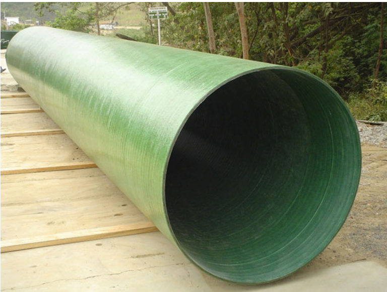
Fig. 5.24 A filament wound pipe (diameter = 2 m) made for irrigation purposes in Ecuador. (courtesy of Odebrecht Co.)
