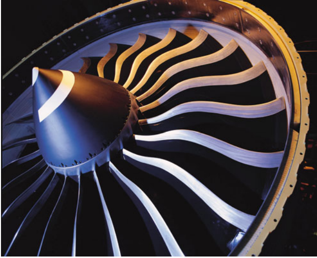
Fig. 5.25 Blades of GEnx engine are made of carbon fiber/epoxy composites (courtesy of General Electric Co.)
