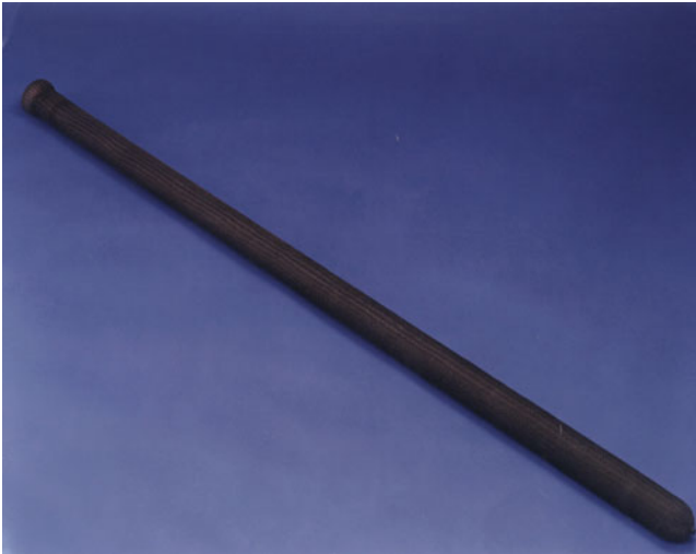
Fig. 7.28 A candle-type filter consisting of Nextel™ 312 ceramic fibers in a silicon carbide matrix. The filter is 1.3 m long. Such filters are used to remove particulate matter from high-temperature gas streams up to 1,000 °C (courtesy of 3M Co.)
