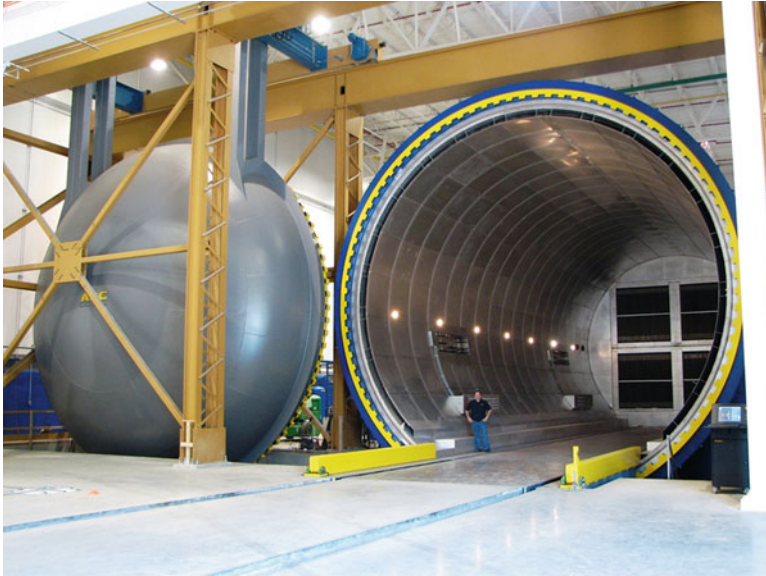
Fig. 5.6 A large autoclave that is used to make the wings of Boeing 787. An idea of the size of the autoclave can be had from the height of the person standing inside the autoclave (courtesy of ASC Process Systems Inc., Sylmar, California)
