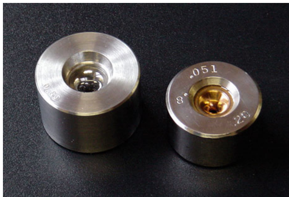
Fig. 5.3 Two wire drawing dies where a hard material occupies the conical inner configuration
