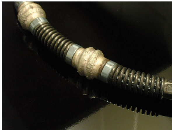
Fig. 9.7 A wire saw for cutting hard stones, such as marble or granite tiles. The bead consists of a diamond composite with tungsten and tungsten carbide shaped by injection molding and infiltrated during sintering [courtesy N. Williams]
