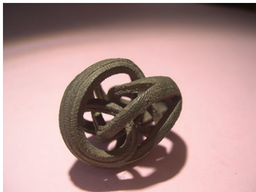
Fig. 7.41 One means to build limited production components is with additive or freeform fabrication. Illustrated here is a computer controlled laser scanner coupled with layered particles. Laser scribing on the top surface the particles induces sintering. By coordination of the repeated layering and the computer image, three-dimensional objects are created by layer-wise sinter builds
