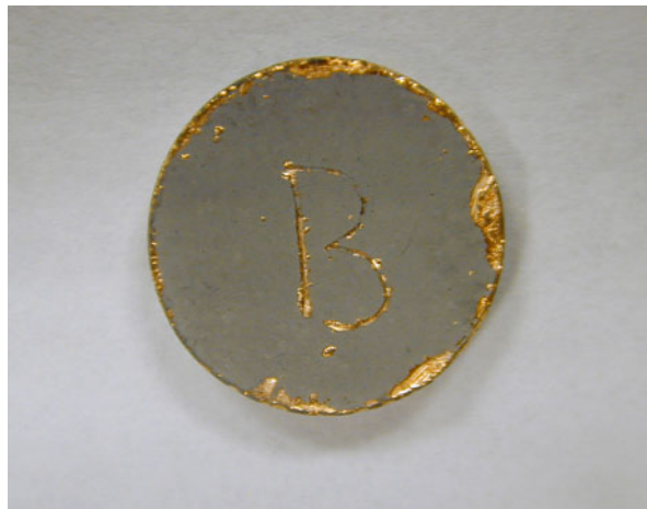
Fig. 11.37 A picture of copper bleeding from the surface of a W-20Cu composite as the result of excess copper used during infiltration
