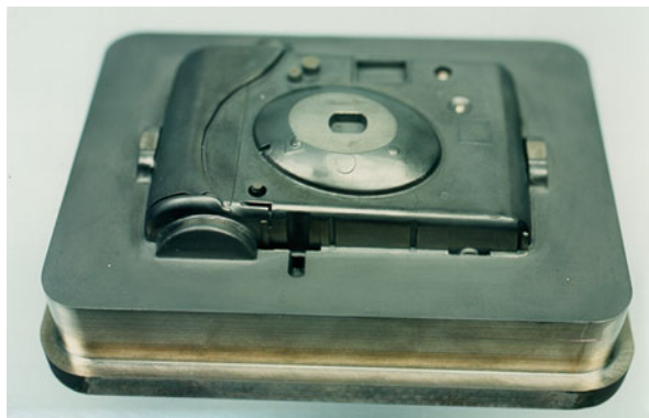
Fig. 9.20 A mold formed by slurry casting tool steel powder with subsequent bronze infiltration to form a composite structure that is then used for plastic injection molding
