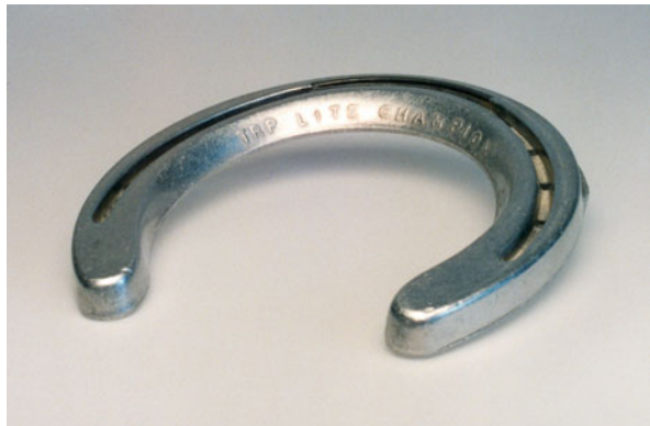
Fig. 11.3 This Al-SiC horseshoe is intended for endurance races, where the low density aluminum is favorably combined with the high wear resistance of silicon carbide
