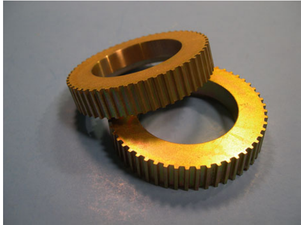
Fig. 9.12 Magnetic rotational sensors called tone wheels, formed by die compaction of a mixture of iron and iron phosphide particles. These illustrate the flat, squat character of ideal die compaction shapes
