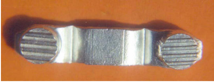
Fig. 11.18 An arc erosion resistant high voltage switching electrical contact that is a composite of tungsten and silver, in this case with excess silver on the exterior
