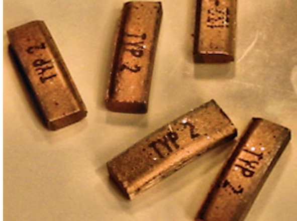
Fig. 9.18 Diamond segments formed by hot pressing, illustrating the relative shape simplicity dictated by the compaction conditions and weak graphite tooling
