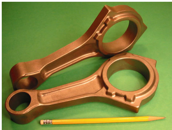
Fig. 9.19 A truck engine connecting rod formed by forging a mixture of iron, copper, and graphite powders to form a full density steel-copper structure. Note the rounded corners associated with forged shapes
