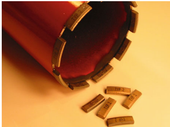
Fig. 11.15 An example of a cement coring tool that consists of a steel tube with diamond composites laser bonded to the steel tube to form the cutting surface. Some segments are shown with the tool
