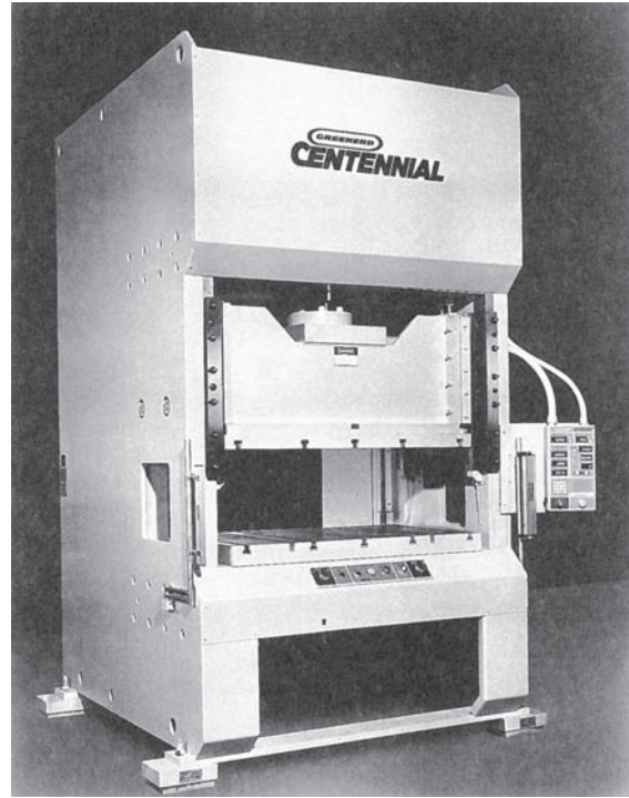
FIGURE 20.37 Straight-sided frame press. (Photo courtesy Greenerd Press & Machine Company, Inc., Nashua, New Hampshire.)
