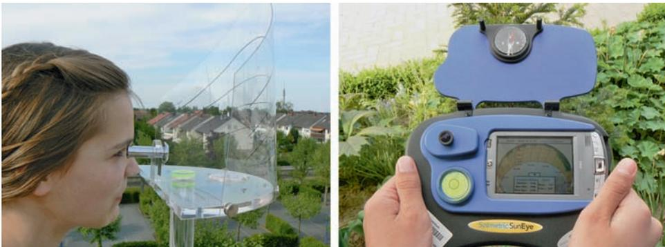
**Figure 9.2** Two variants of the shading analysis: The left picture shows the manually operated Sun path indicator and the right picture shows the SunEye device that permits automatic acquisition of the shading horizon
