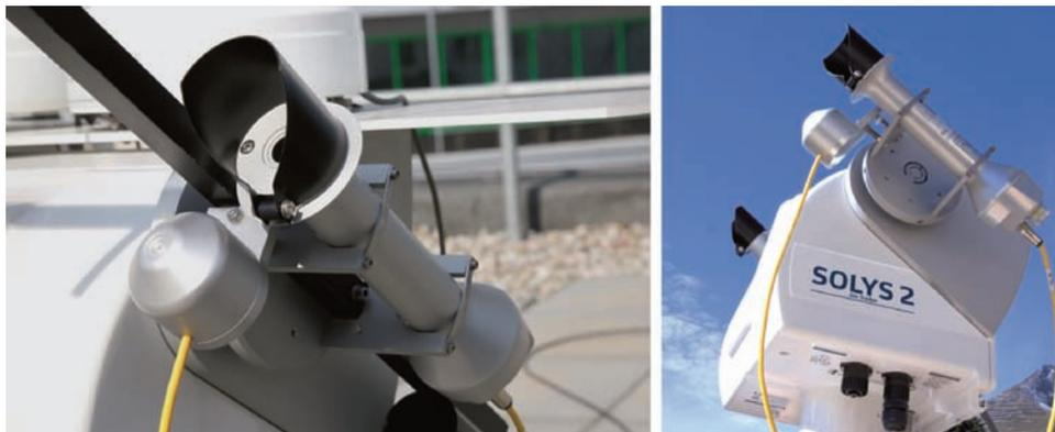
**Figure 8.4** Pyrhelimeter for measuring direct radiation: The instrument must continuously track the Sun (photos: Kipp and Zonen)
