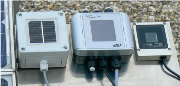
**Figure 8.3** Various reference sensors of c-Si solar cells at the experimental rig of the Münster University of Applied Sciences: The modules are installed at module level in order to measure the incident radiation on the solar module
