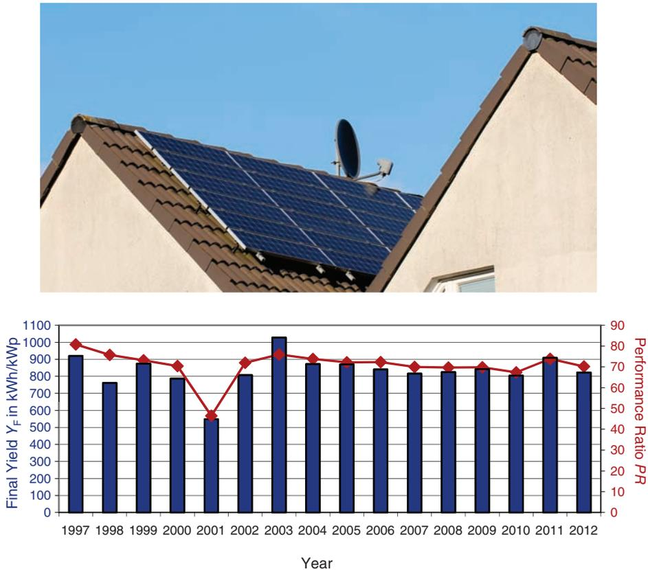
**Figure 9.11** View and operating results of a 2 kW installation in Aachen: The poor yield in 2001 can be clearly seen and was caused by a burned-through fuse (photo: M. Pankert)
