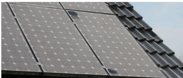
**Figure 8.12** “Thermography for the poor” on a cold November day: The two cells of the modules from Figure 8.10 can be clearly seen as free from hoarfrost (photo: T. Stegmann, Münster UAS)
