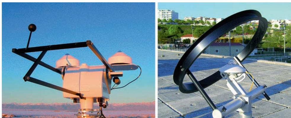
**Figure 8.5** Sensors for measuring diffuse radiation: Whereas the shade ball variant must continuously track the Sun, the shade ring is satisfied with an occasional adjustment of the tilt angle (photos: Kipp and Zonen)
