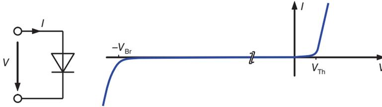
**Figure 3.18** Symbol and  $I/V$  characteristic curve of a p-n diode: in the forward direction the diode only conducts from the threshold voltage  $V_{Th}$ , in reverse direction, there are high currents in the case of exceeding the breakthrough voltage  $V_{Br}$
