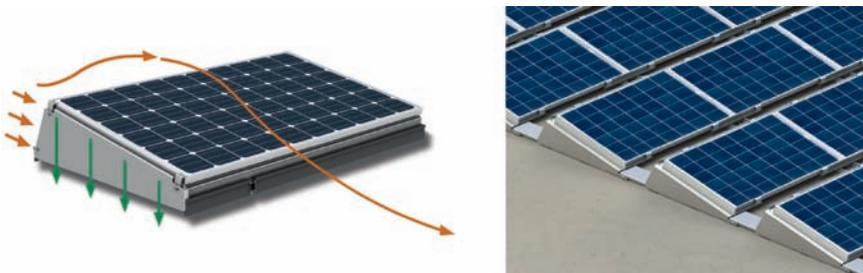
**Figure 6.31** Solution for roofs with low bearing capacity: Because of the low closed form the system offers hardly any resistance to the wind; instead the elements are pressed down by the wind (source: LORENZ-Montagesysteme GmbH)
