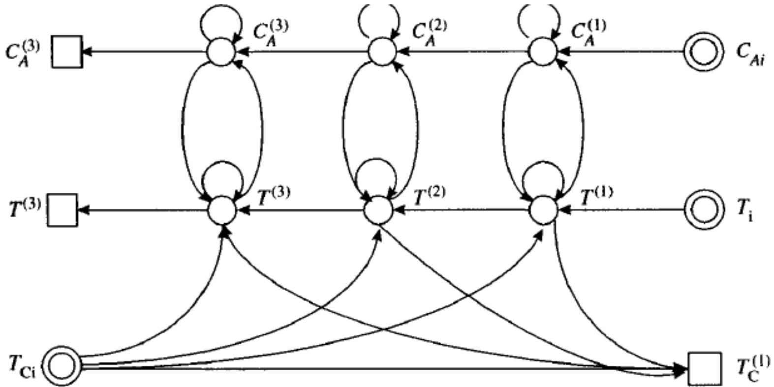
Simplified structure graph of three jacketted CSTRs by variable removal
