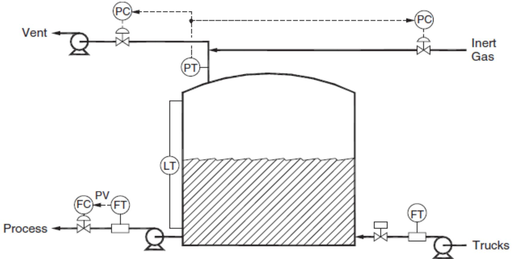
Figure 2.12 Oil storage tank with two feedback controllers
