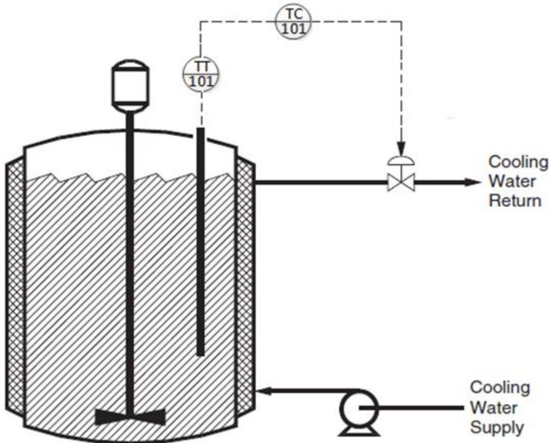
Normal Operation: Maintain reactor temperature at desired value.
