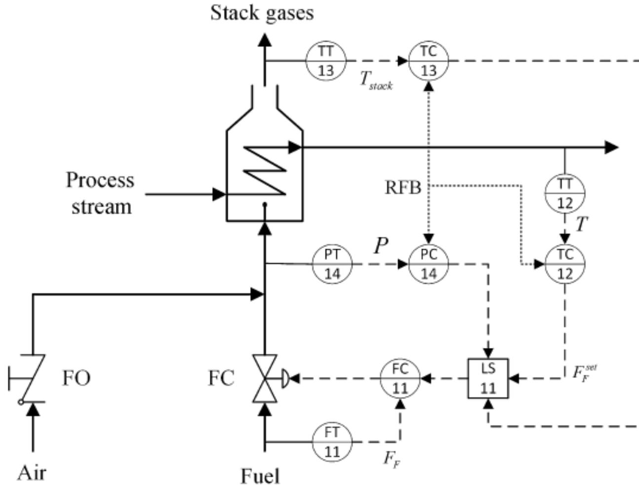
Figure 2.7 Furnace override control
