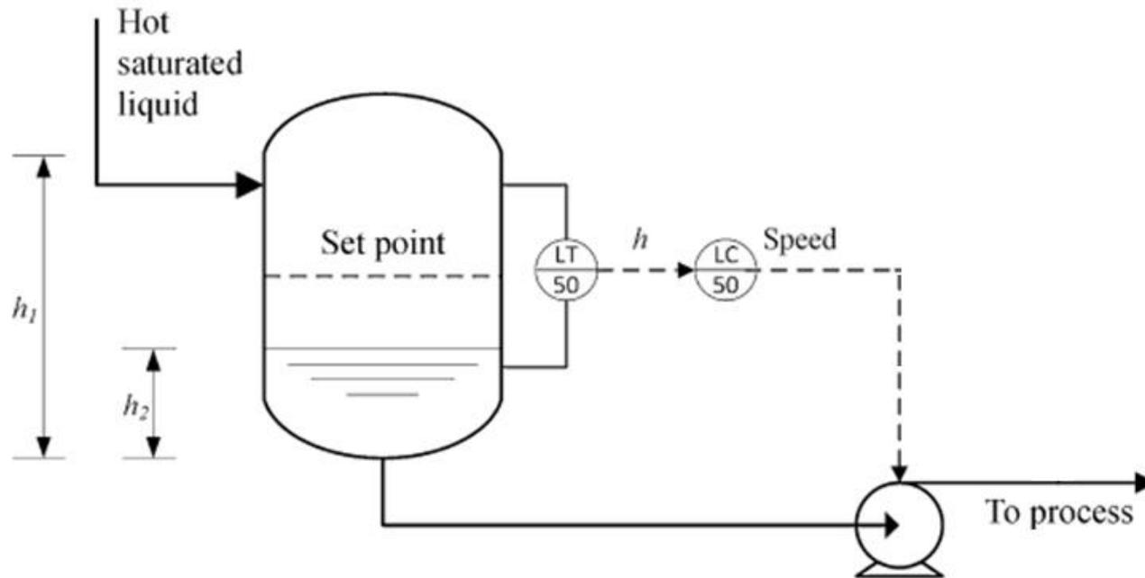
**Figure 2.2 Level Control- Feedback**
