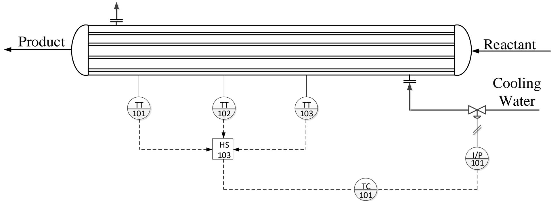
Figure 2.1 A fixed-bed catalytic tubular reactor with an exothermic reaction.
