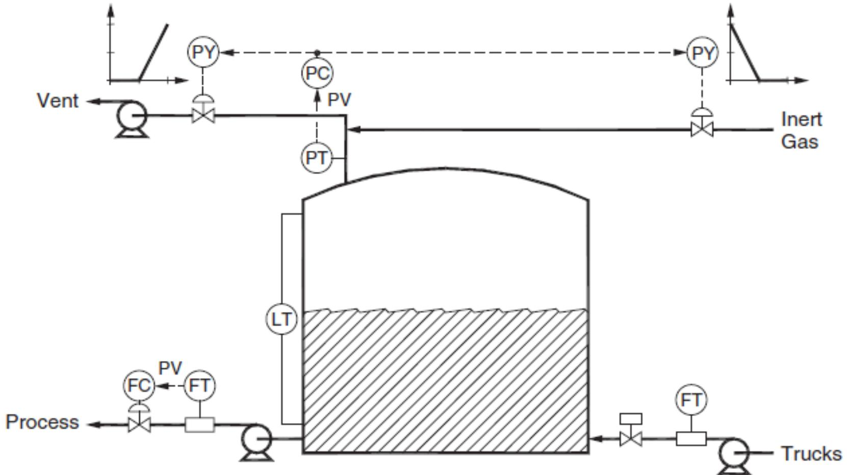
Figure 2.13 Oil storage tank with two feedback controllers
