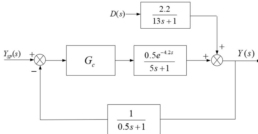
Figure Q4. Feedback control system
