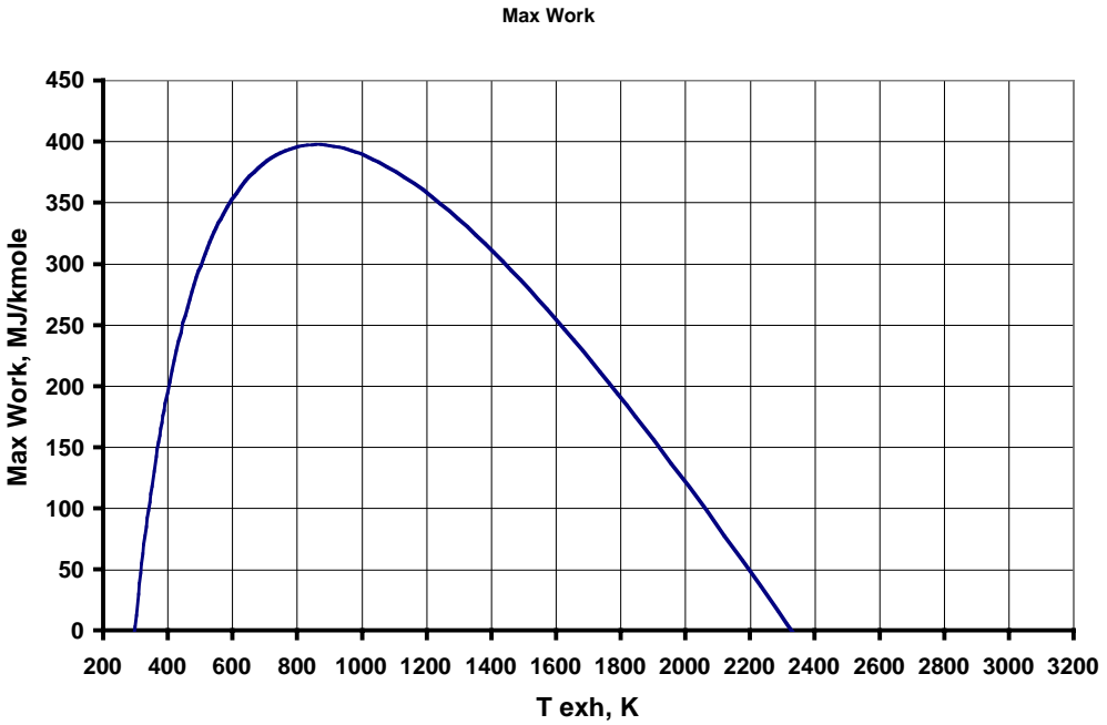
Figure 3: Work output with respect to T_{HE} . for stoichiometric methane–air combustion considering variable specific heat c_{po}(T) .
