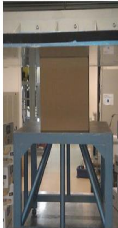
Box compression test (ISO 12048, ASTM D 642)
