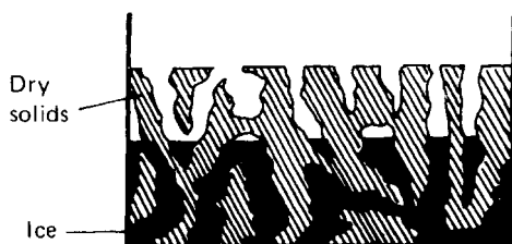
Fig. 22.4 Porous structure of freeze-dried food.
