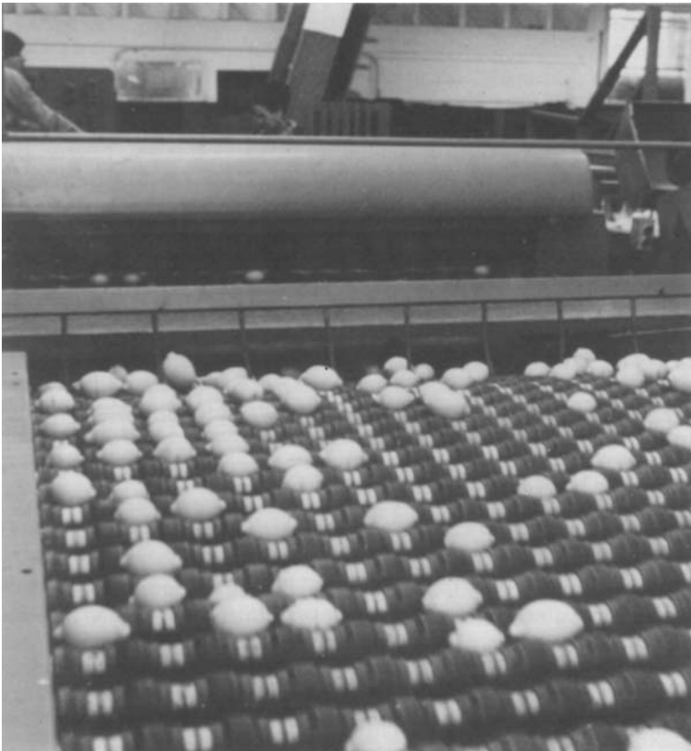
Fig. 3.7 Sorting lemons on a roller sorter. (Courtesy of Sunkist Growers.)
