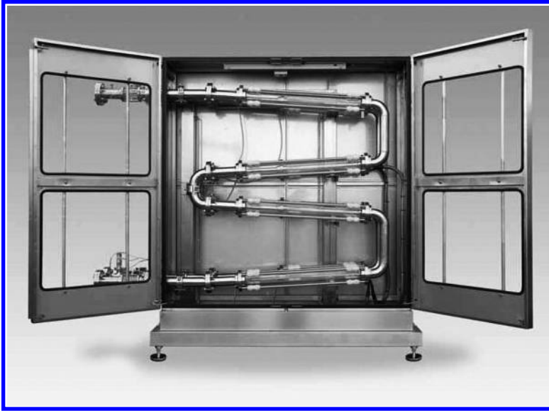
FIGURE 10.3 Ohmic heater of 240 kW for soup processing. (Courtesy of Emmepiemme, Piacenza, Italy; From Municino, F., Industrial applications of Ohmic heating of foods, in: Workshop on Ohmic Heating , Abrantes, Portugal, December 19, 2012.)
