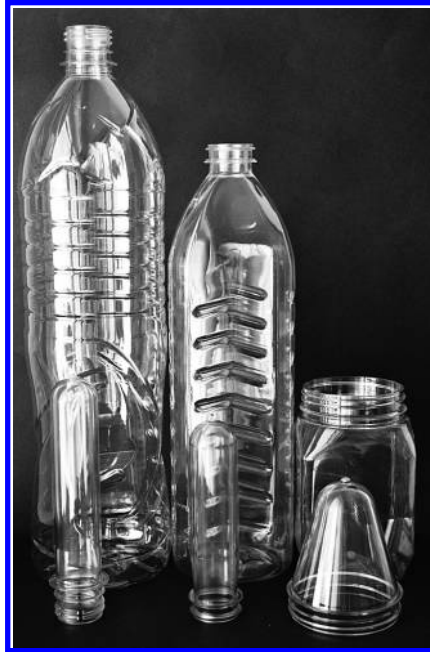
FIGURE 17.8 PET bottles and jar and respective preforms.
