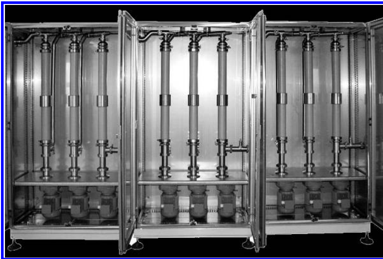
FIGURE 10.4 Example of Ohmic heating unit with heating tubes in series. (From Agro-Process, Technologie chauffage direct , ZIP Technologique Cintech Agroalimentaire , 27th edn., April 8, 2010, Saint-Hyacinthe, Quebec, Canada, 2010, also available at Internet: www.agro-process.com . Accessed on October 10, 2013.)
