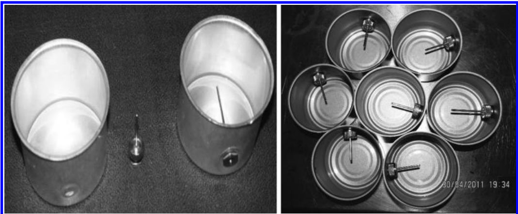
FIGURE 3.9 Aluminum and TFS cans fitted with thermocouple.
