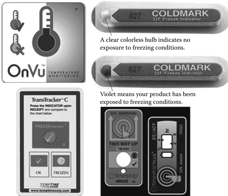
FIGURE 7.12 Examples of time temperature indicators used in the current cold chain to monitor the real time temperature history of frozen and chilled products.
