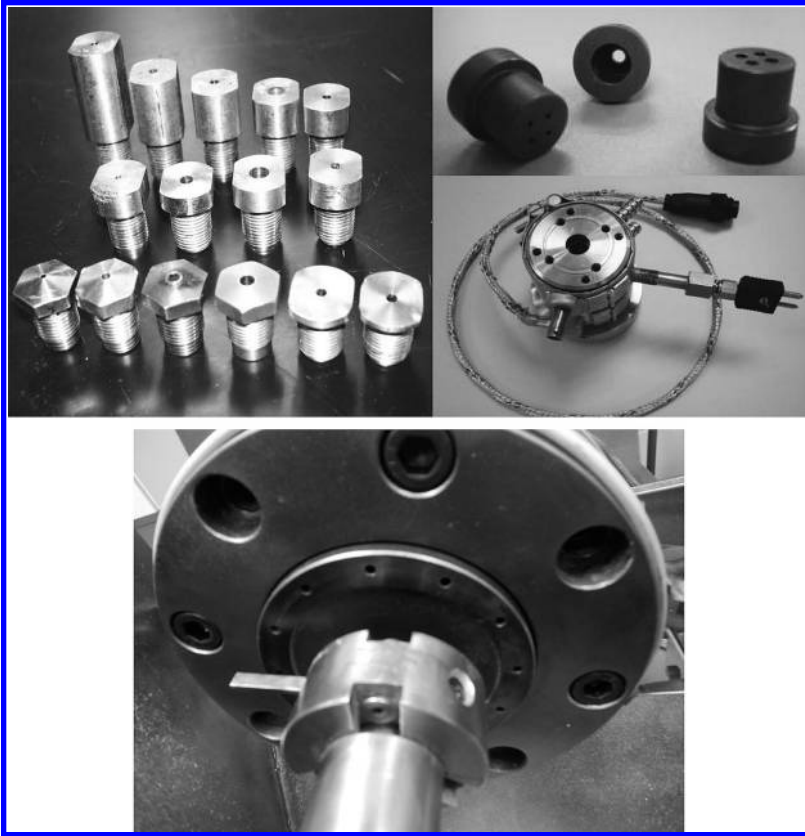
FIGURE 4.2 Die inserts (with single and multiple openings) and die assembly. (Courtesy of C.W. Brabender, Germany.)
