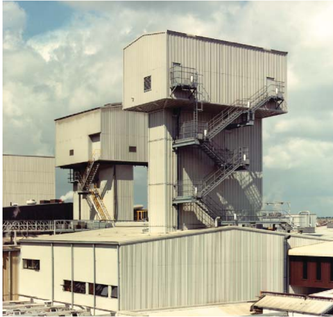
Figure 6.6 Exterior view of a continuous hydrostatic sterilizer (source: Photo courtesy of JBT FoodTech, formerly FMC FoodTech, Madera, CA). See plate section for colour version
