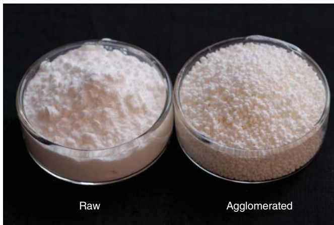
Figure 13.7 Unprocessed (raw) and agglomerated corn starch samples. The latter sample is obtained by moistening, steaming and granulation followed by final drying
