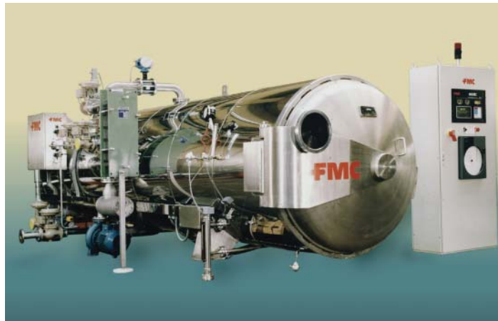
Figure 6.3 Modern-day horizontal batch retort (source: Photo courtesy of JBT FoodTech, formerly FMC FoodTech, Madera, CA)
