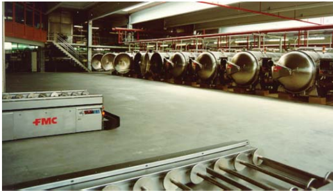
Figure 6.4 Batch retort system showing battery of retorts in a large cook room operation (source: Photo courtesy of JBT FoodTech, formerly FMC FoodTech, Madera, CA)
