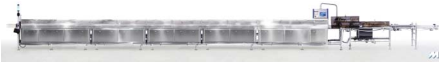
Figure 18.3 Microwave pasteurization tunnel for production of ready-to-heat meals (source: http://www.micvac.com/food-technology/equipment by Hanna Rüdél. Reproduced with permission of MicVac.)
