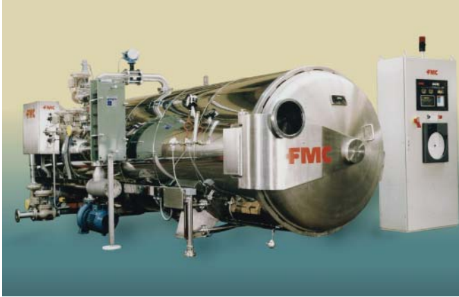
Figure 6.3 Modern-day horizontal batch retort (source: Photo courtesy of JBT FoodTech, formerly FMC FoodTech, Madera, CA). See plate section for colour version
