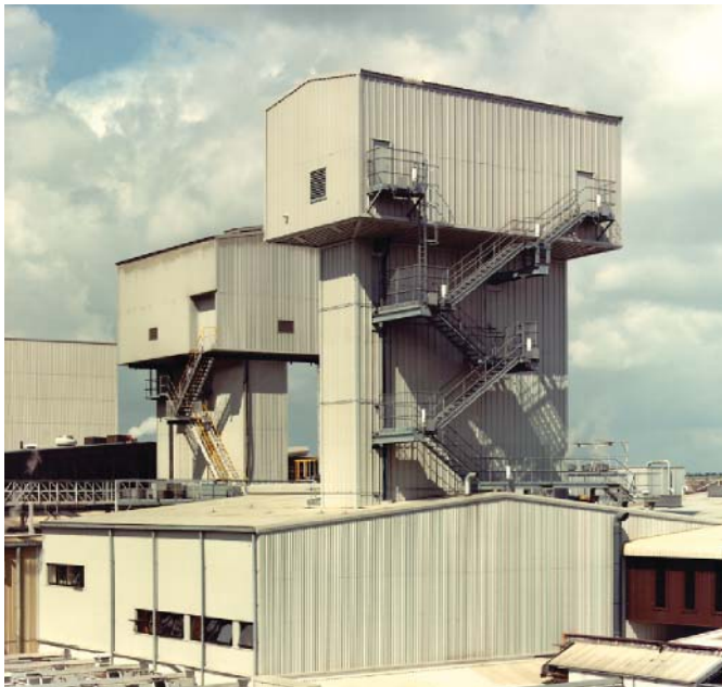
Figure 6.6 Exterior view of a continuous hydrostatic sterilizer (source: Photo courtesy of JBT FoodTech, formerly FMC FoodTech, Madera, CA)
