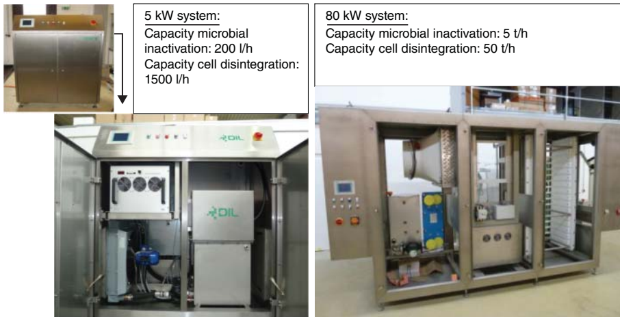
Figure 26.5 PEF units developed by DIL and the related maximum capacities; left side: pulse transformer setup; right side: semiconductor-based Marx generator equipment (source: DIL e.V., Quakenbrueck, Germany)
