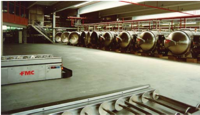
Figure 6.4 Batch retort system showing battery of retorts in a large cook room operation (source: Photo courtesy of JBT FoodTech, formerly FMC FoodTech, Madera, CA). See plate section for colour version
