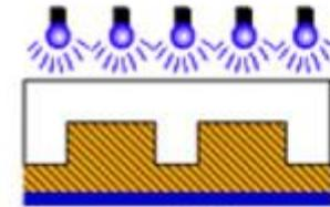
Transparent stamp allows UV light to polymerize resist, causing solidification
