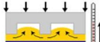
Heat thermoplastic polymer to decrease viscosity, then imprint malleable resist
