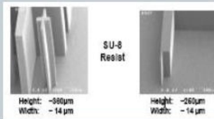
Figure1: 3-D microstructure
