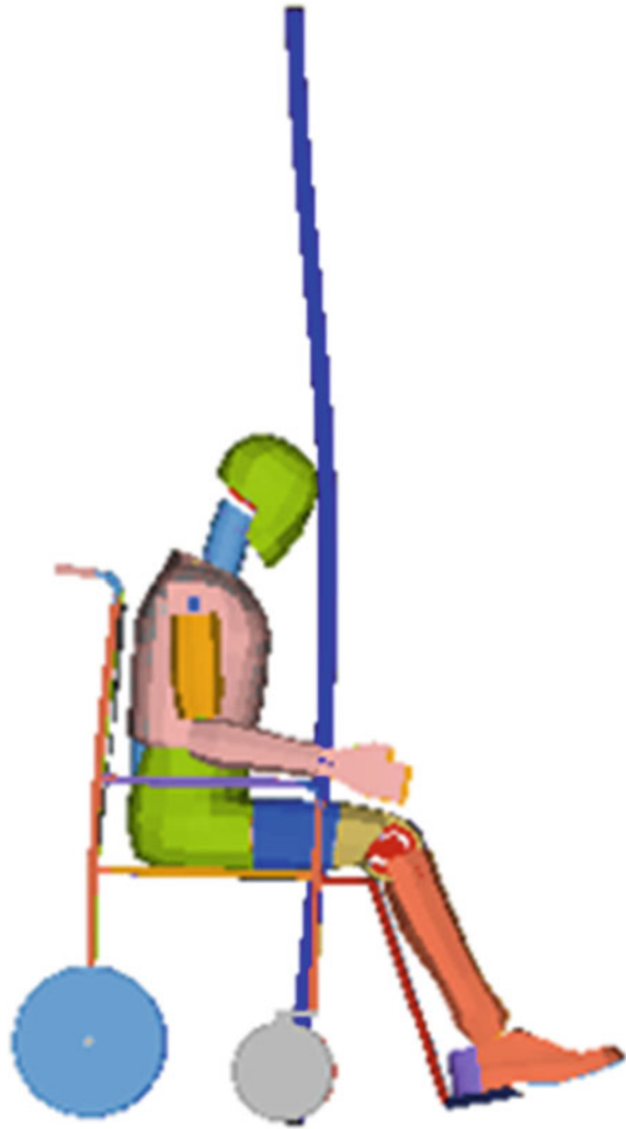
Fig. 5.12 Wheelchair occupant secondary collision with a grab pole
