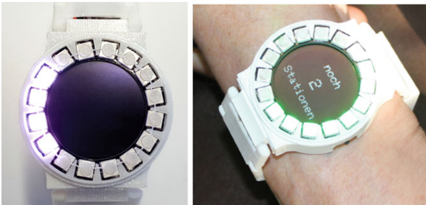
Fig. 9.7 Left LED ring providing directional information about where to go next; right OLED display showed the number of stops left until departure
