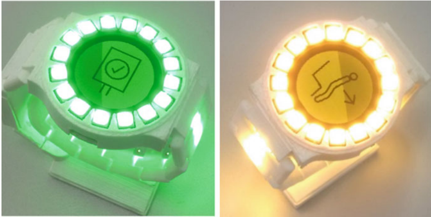
Fig. 9.6 LED rings and LED ribbon as well as OLED display providing simple information ( left “right bus stop”; right “leave car at next bus stop”)
