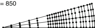
Fig. 5.4 Finite element idealisation of Dungeness B vessel ( Note: For clarity certain nodes are not shown)
