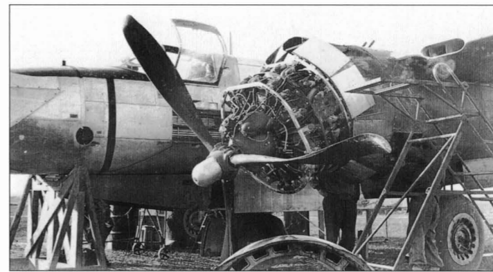
Yet another landing gear collapse inflicted this damage to a clamshell canopy A-26 in early 1945. Note the wooden trestle beneath the bomber's nose
