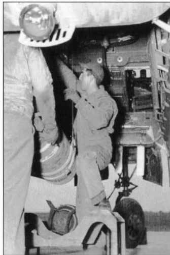
Armourers carefully winch a 500-lb (GP) bomb into the bomb-bay of a Project Squadron Invader at Great Dunmow
