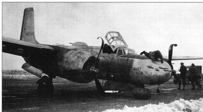
Fitted with underwing gun pods, this A-26B suffered a nose gear failure whilst taxiing at Laon/Athies in early 1945. Both propellers have been badly damaged and the engines wrenched. The aircraft is also equipped with a large, heavily-framed hatch on the right-hand side of the canopy, which provided cockpit access. This early style hatch severely restricted pilot visibility
