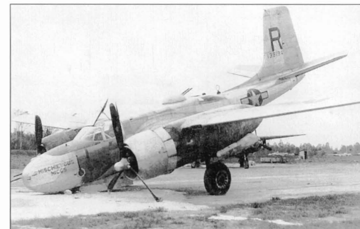
A-26B-15-DL Invader 41-29194 MISCHIEVOUS MICCS suffered a nose gear failure on landing at Coulommiers in late 1944. Note the olive drab A-20s parked behind the aircraft
