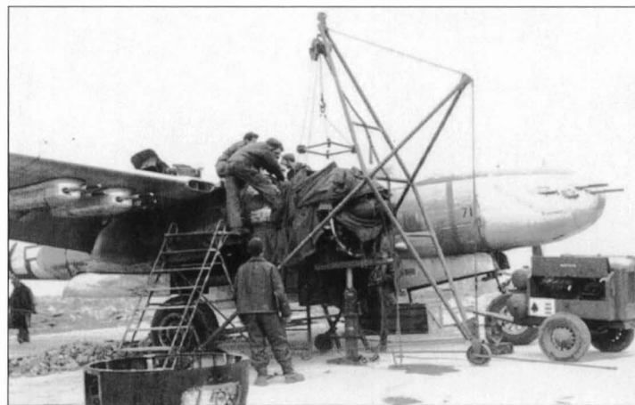
Various airfield support equipment can be seen in this photograph of a 416th BG A-26B undergoing an engine change in the open
