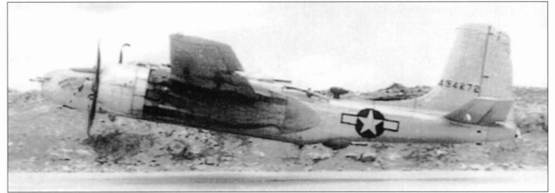
The pilot of A-26B-50-DL 44-34272 PRINCESS PUD carries out a forced landing at Machinato on 10 August 1945 following a mid-air collision with another 319th BG aircraft during a mission to Kyushu. Note bent right propeller, which the pilot had to feather after the collision
