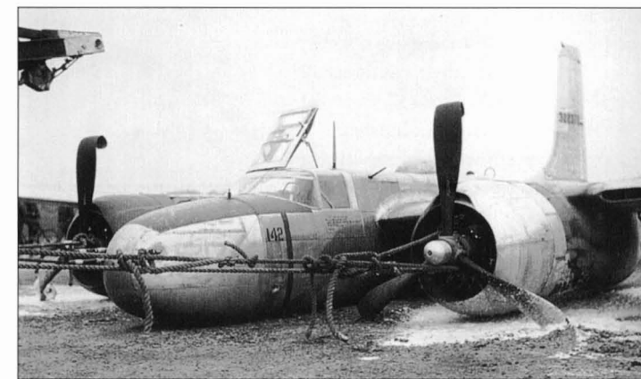
In an effort to improve cockpit visibility, a revised canopy style was quickly introduced by Douglas. As this damaged machine from the 416th BG clearly shows, two framed panels on the left hand side of the canopy were replaced by a single large frameless panel
