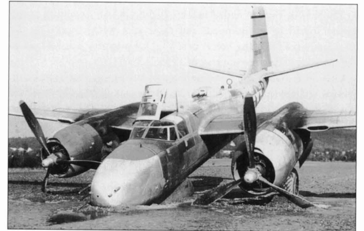
Below and bottom The nose gear of this A-26B collapsed on landing after a training mission at Wethersfield on 18 October 1944. This is one of at least three landing gear failures known to have occurred on the same day and at the same location
