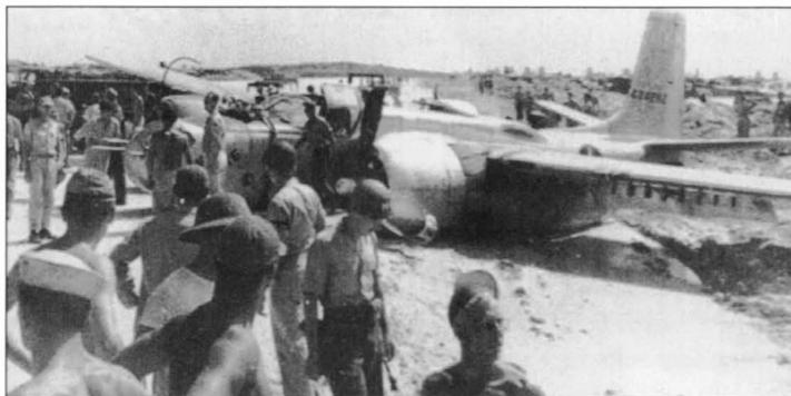
This 319th BG aircraft made a belly landing at Machinato after its gear malfunctioned upon returning from a mission. Note the rocket mounting pylons under the left wing
