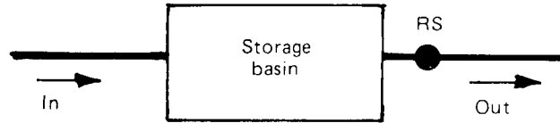
FIGURE 18.3 Location of a flow regulating structure in an in-line connected storage. (From Stahre and Urbonas, 1990)
