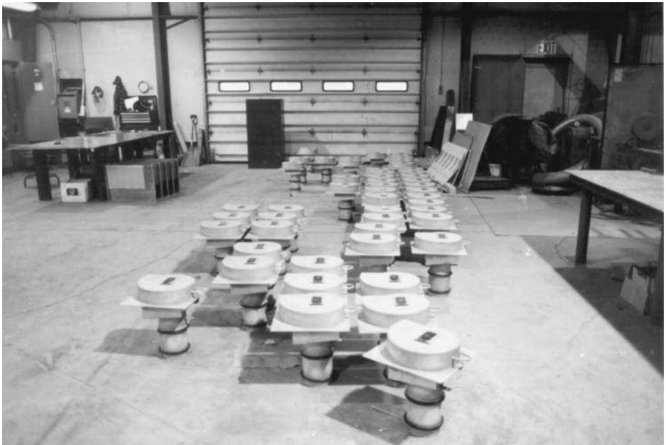
FIGURE 18.32 3-Inch Catchbasin Control Units. The valve assembly comprises 2 parts: one which is pushed into the outlet pipe; and the valve itself which seats on the slide mount. The valve may be removed from its seating to facilitate maintenance. Many hundreds of controls such as these have been supplied. Stormwater attenuation techniques utilizing the vortex valve in this way have been shown to be extremely cost effective. (From HydroInternational, PLC)
