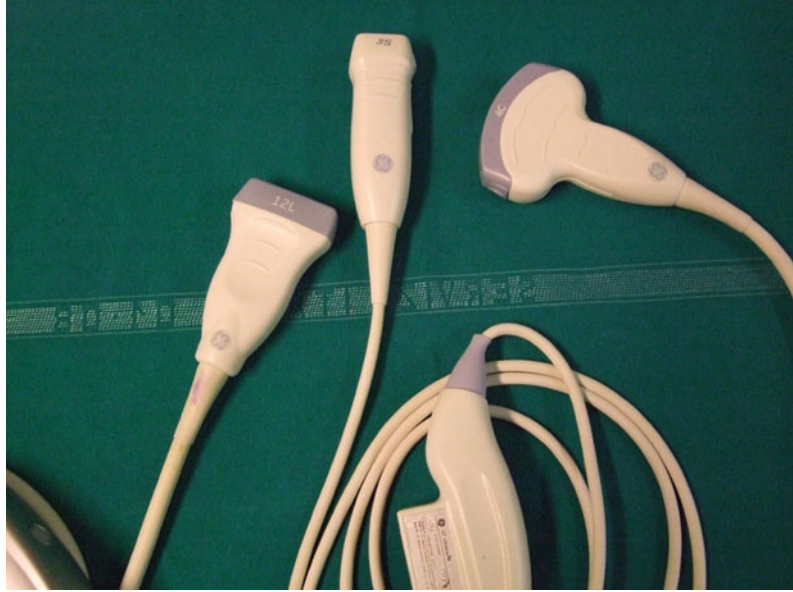
Fig. 1.23 Ultrasound probes. From left to right : vascular and soft tissue linear probe, cardiac phased-array probe, abdominal convex probe
