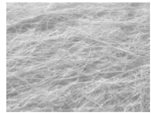
Fig. 3 Filter membrane of less clogging PVD
