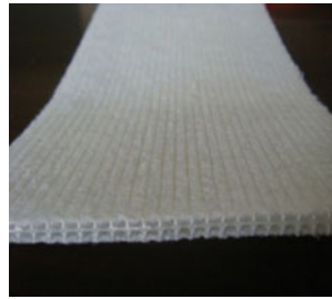
Fig. 3 Filter membrane of less clogging PVD
