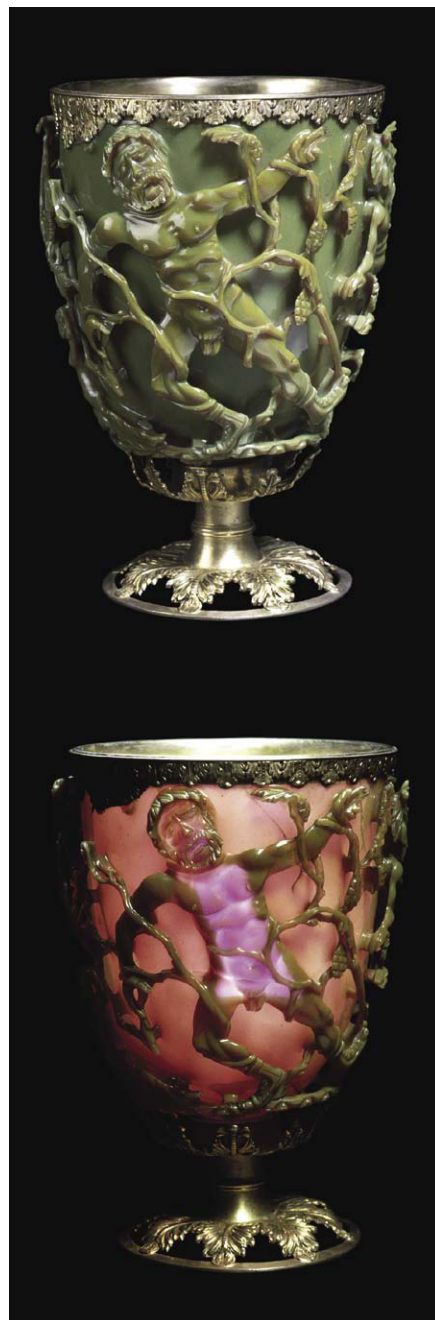
FIGURE 2.17 The Lycurgus cup looks green when light shines on it but red when a light shines inside it. The cup contains gold nanoparticles. (Courtesy of the British Museum.)
