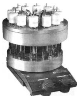
Figure 3. The Radleys reaction block (left) mounts on a standard stirplate. Reaction blocks by STEM (center) and H+P (right) are available in numerous sizes and can provide heating/cooling as well as magnetic stirring in each position. A reflux option is also available.
