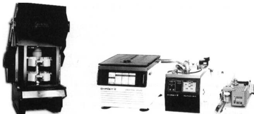
Figure 14. Vacuum centrifuges: Genevac's Mega Series and CHRIST's Beta RVC. Both have been integrated with robotic systems.
