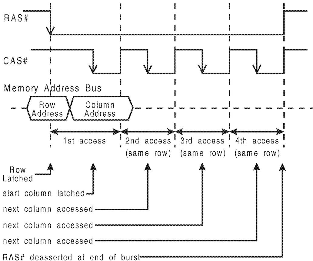
Figure 13-14. Burst Mode Access Timing
