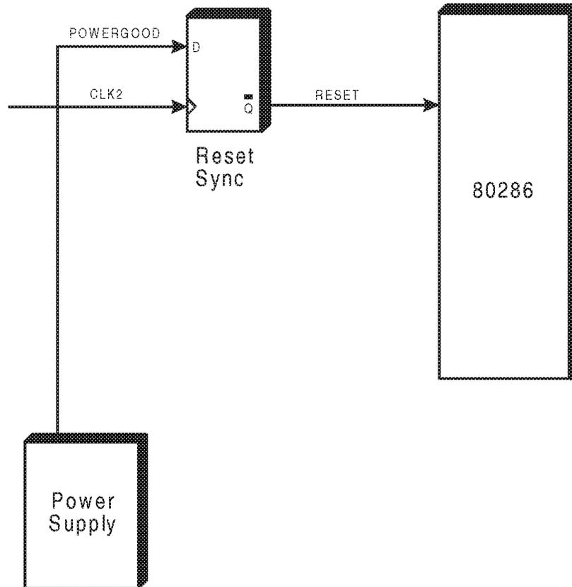
*Figure 5-18. The Reset Logic*
