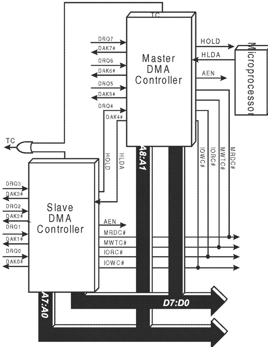
Figure 20-1. DMA and Bus Mastering
