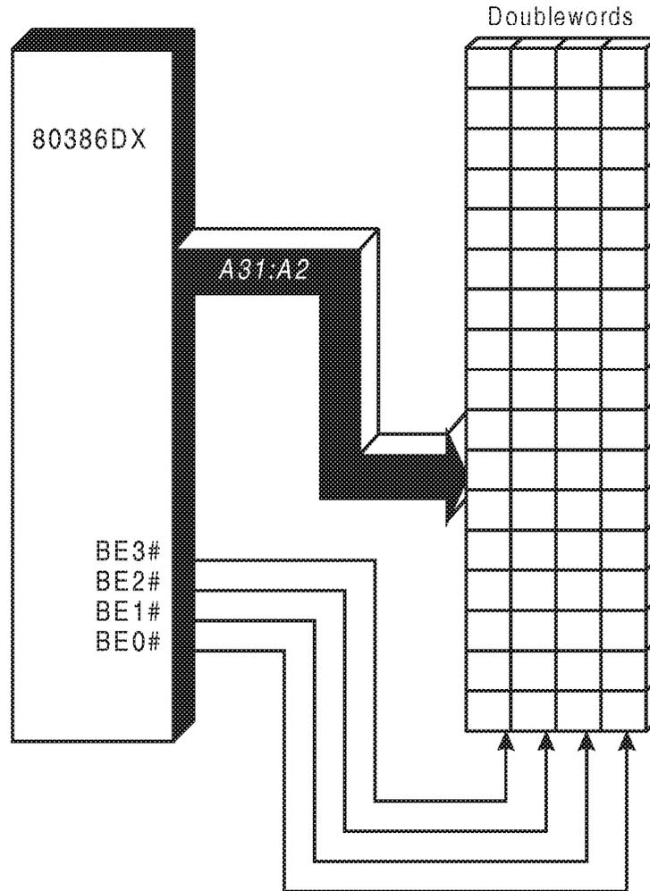
*Figure 10-13. 80386DX Address/Byte Enable Relationship*
