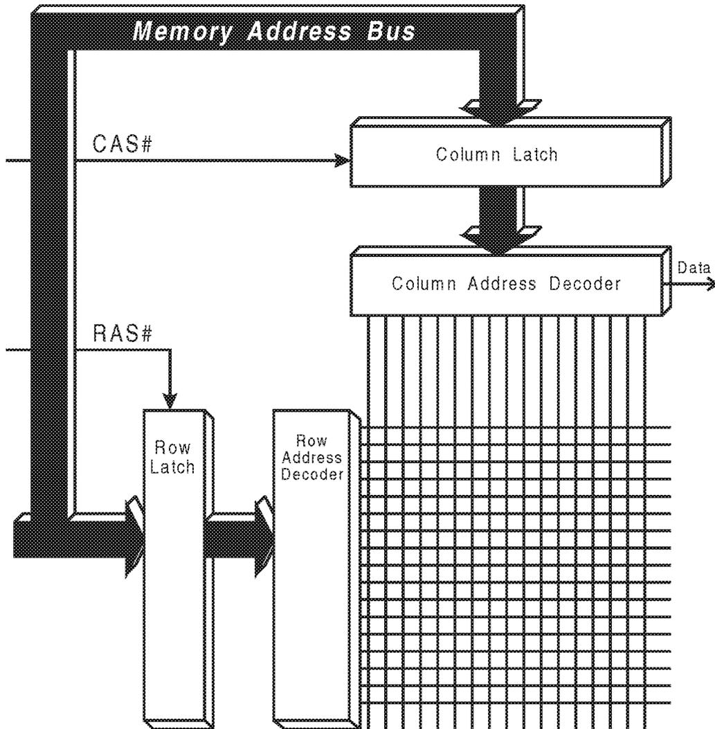
Figure 13-1. Block Diagram of a DRAM Memory Chip
