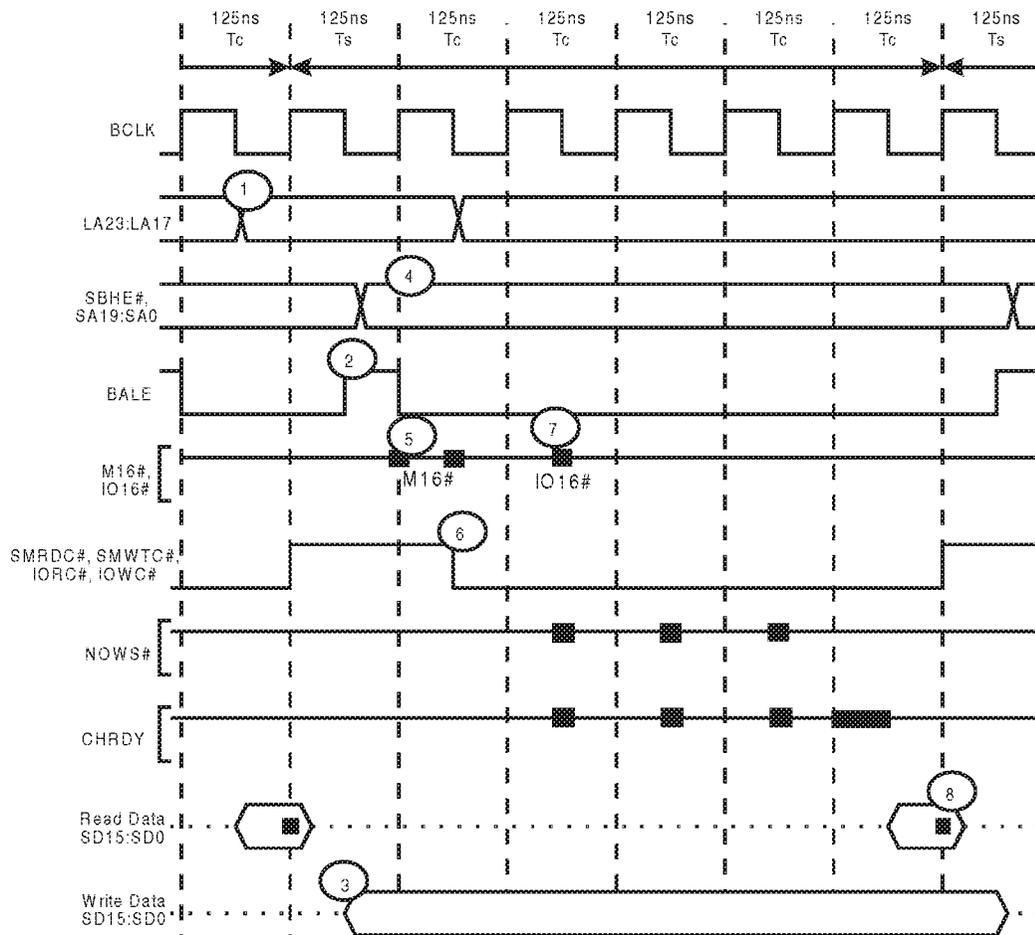
*Figure 17-1. Standard Access to an 8-bit ISA Device*
