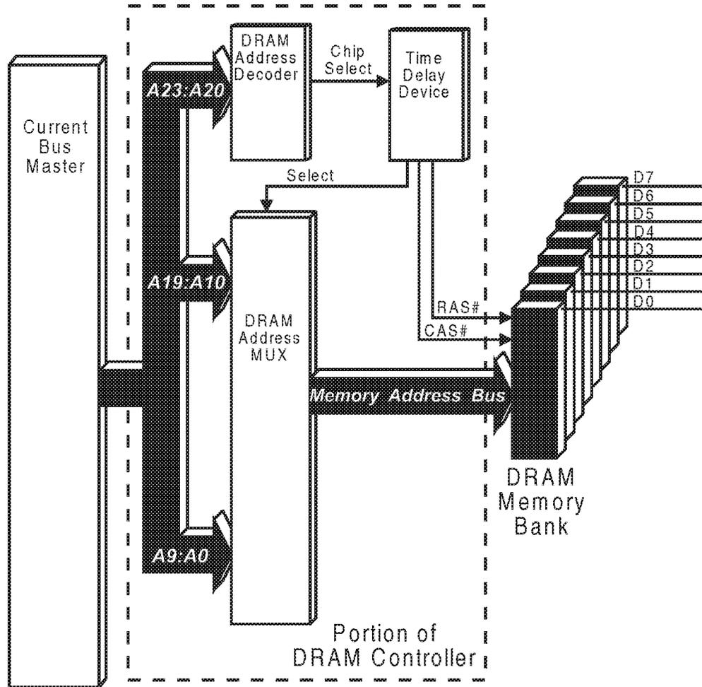
Figure 13-4. Block Diagram of DRAM Addressing Logic
