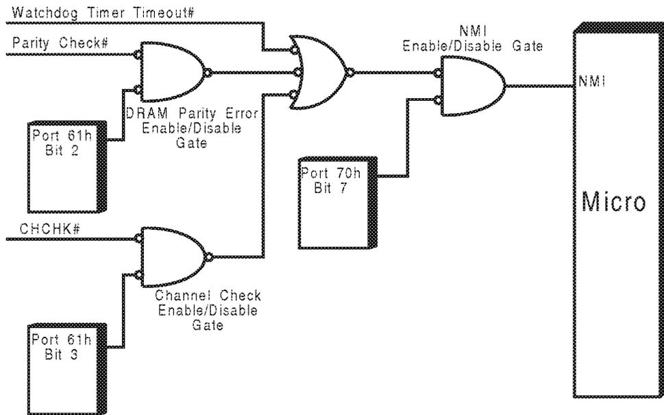
Figure 16-6. The Channel Check Logic
