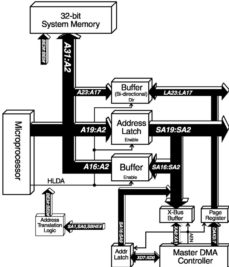
Figure 19-8. 16-bit Access to 32-bit Memory with DMA
