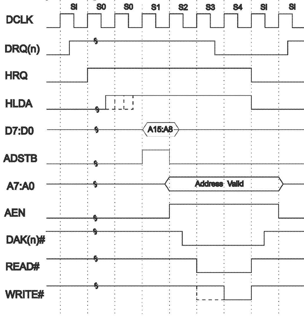
Figure 19-3. Single Transfer Mode Timing
