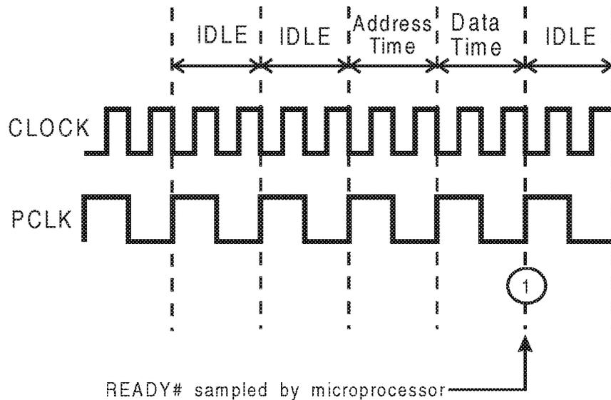
Figure 2-4. Bus Cycle Consisting of Address Time and Data Time
