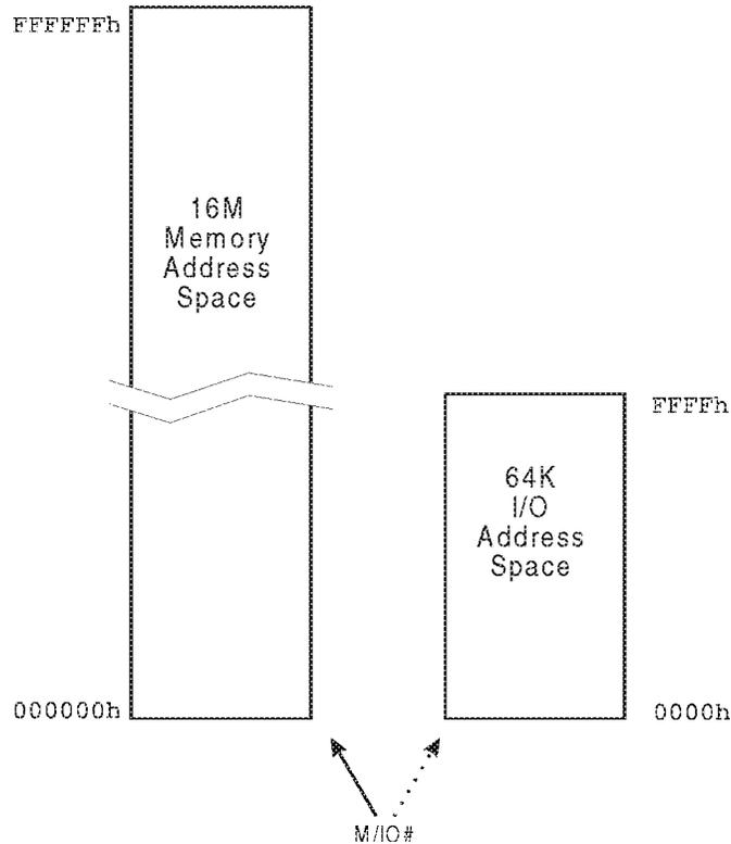
*Figure 3-4. 286 and 386SX Memory and I/O Address Space*
