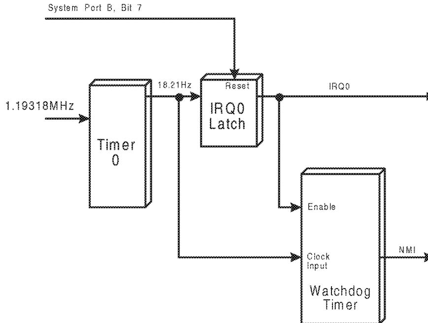
Figure 24-3. The Watchdog Timer and Associated Logic
