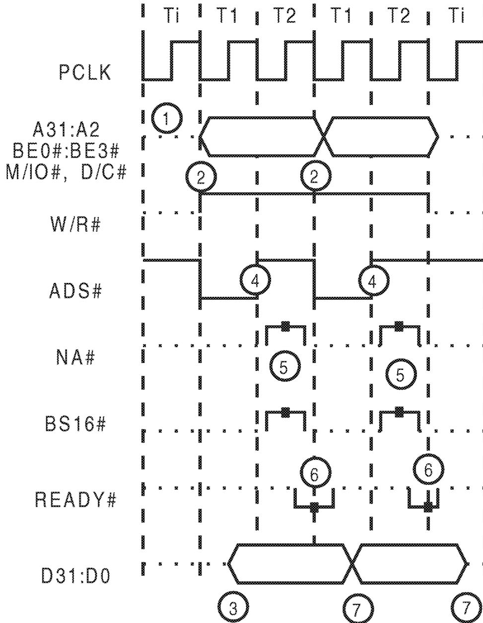
*Figure 12-2. Non-Pipelined Write Bus Cycle*
