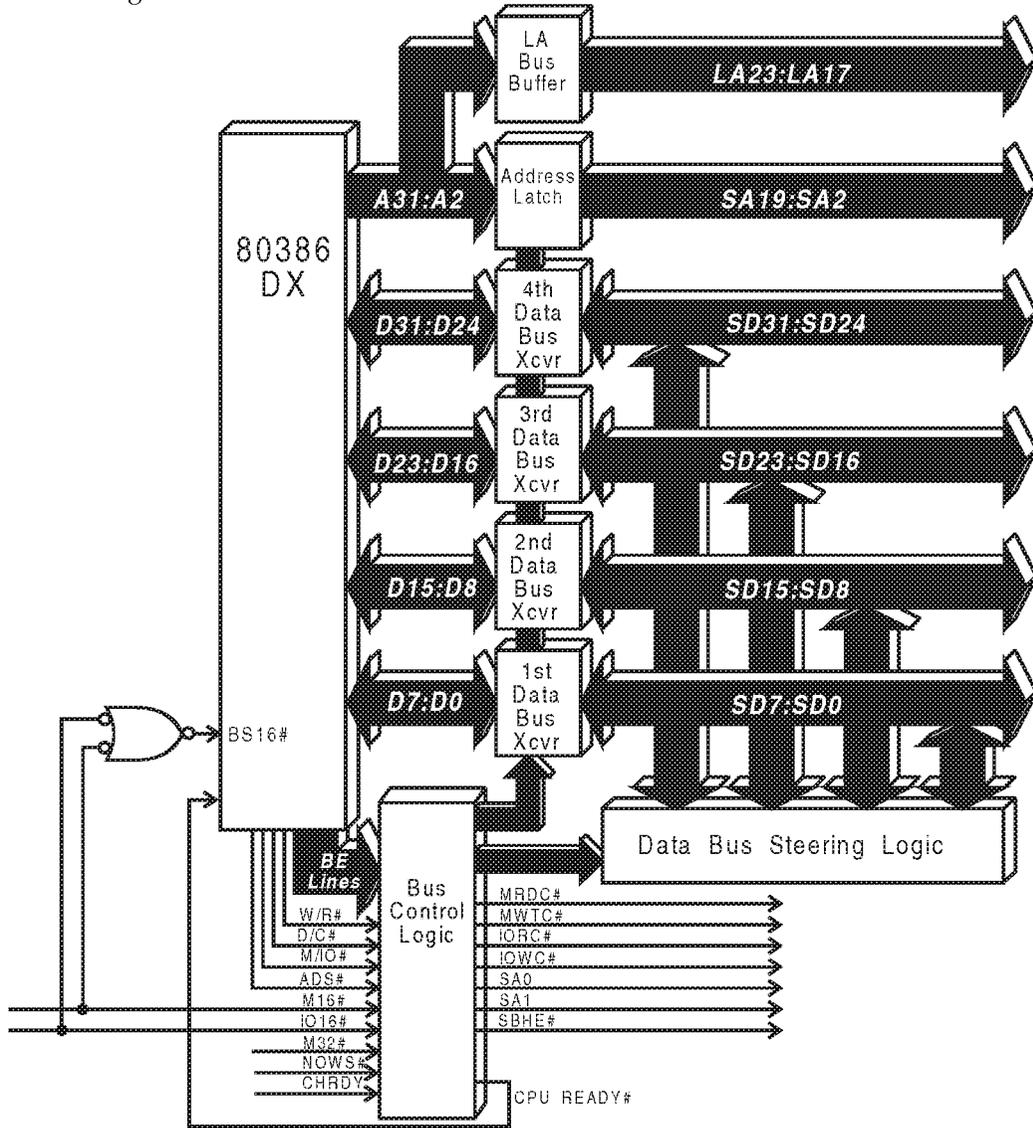
Figure 11-2. The 80386DX-Based Kernel with Dynamic Bus Sizing Implemented
