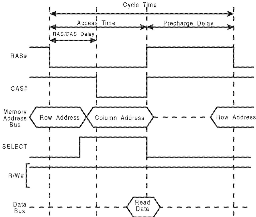
Figure 13-7. Pre-Charge Delay and Cycle Time
