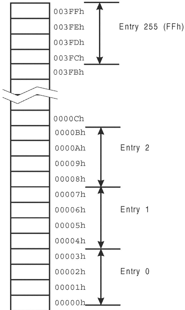
Figure 18-3. The Interrupt Table (in Real Mode)
