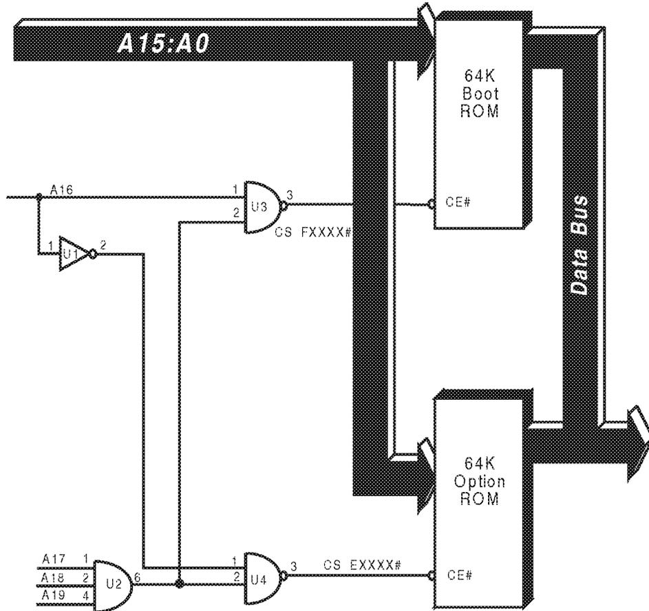
Figure 4-3. Example PC/XT ROM Address Decoder
