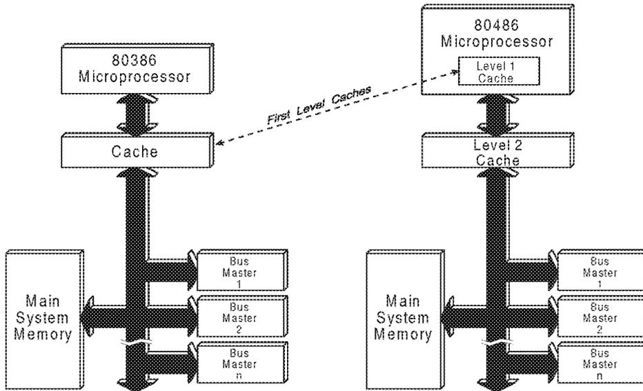
Figure 14-7. First- and Second-Level Caches
