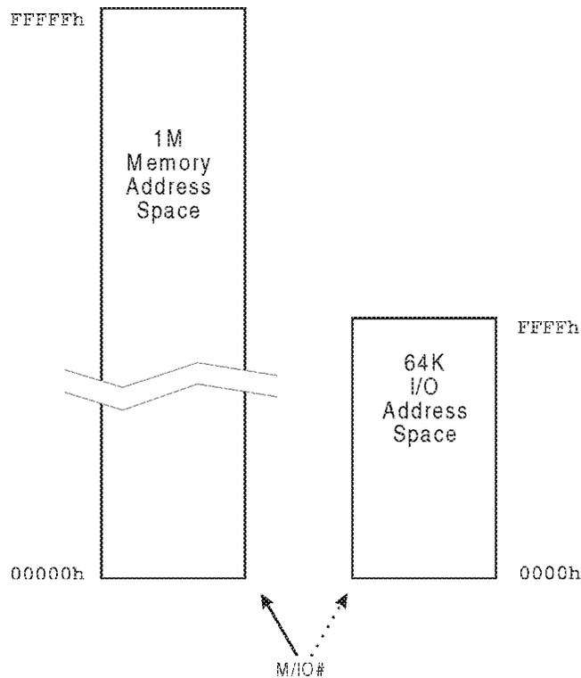
Figure 3-3. 8086 and 8088 Memory and I/O Address Space
