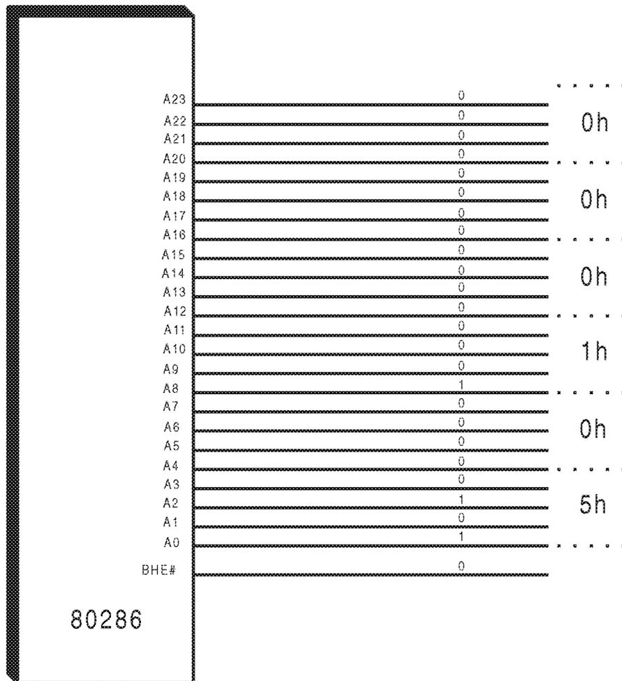
*Figure 1-3. The 80286 Address Bus*
