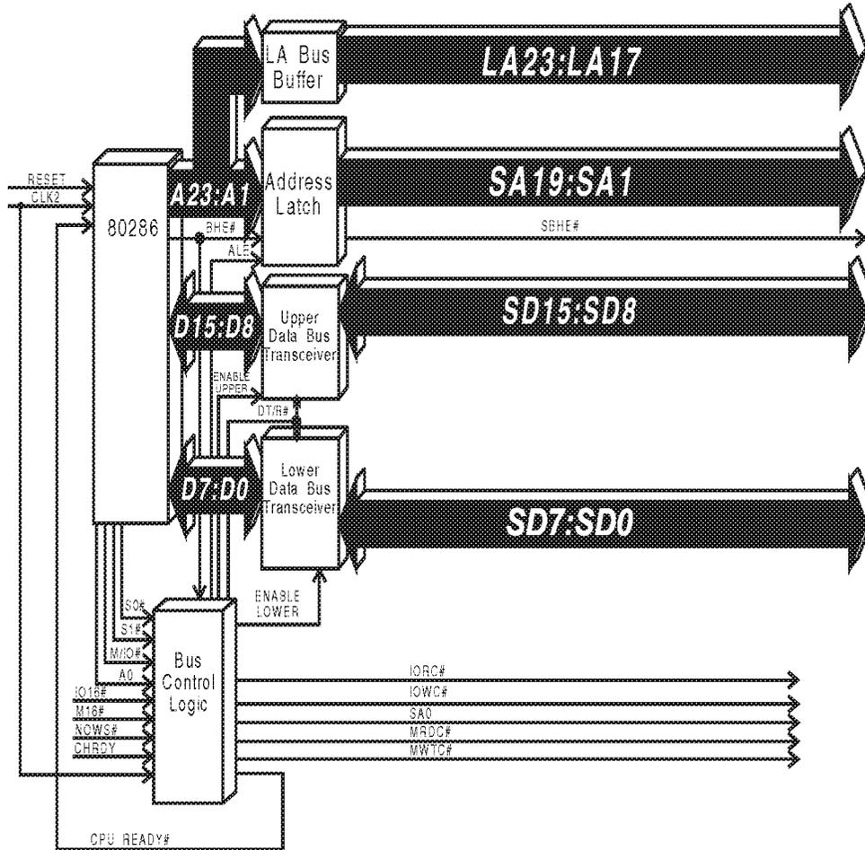
Figure 8-3. The Data Bus Transceivers
