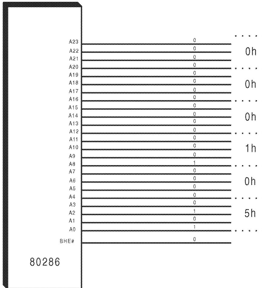
Figure 5-14. The 80286 Address Bus
