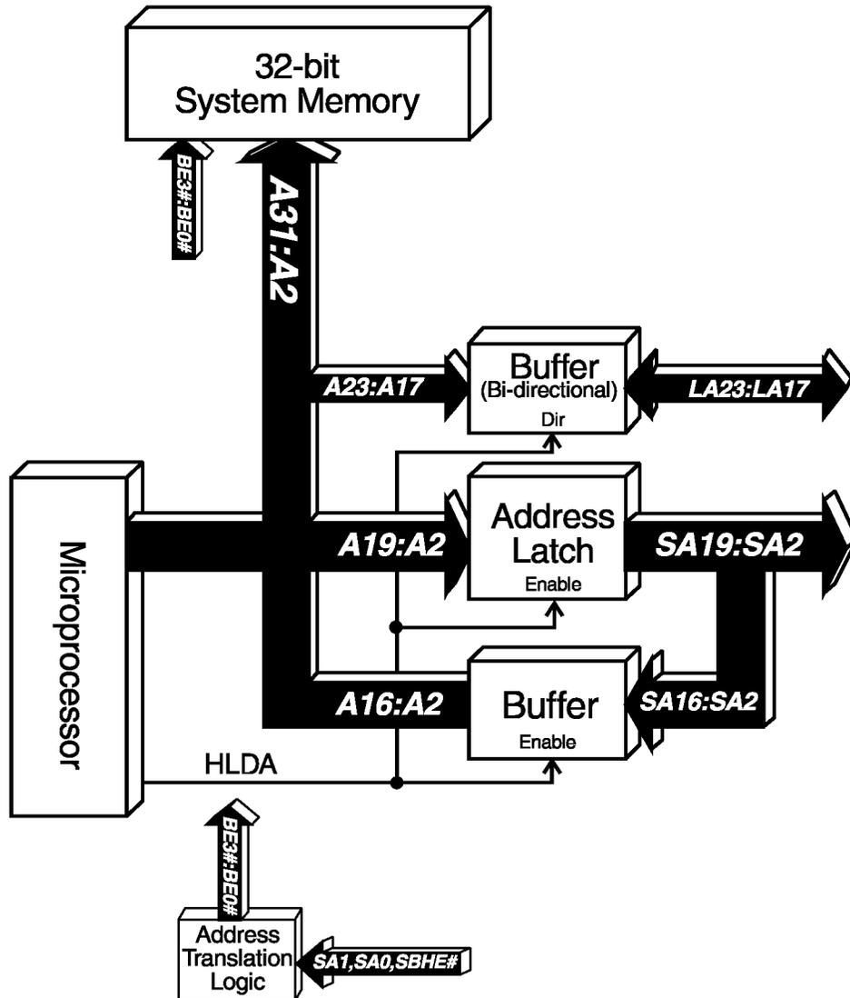
Figure 20-3. Addressing 32-bit Memory with ISA Bus Masters
