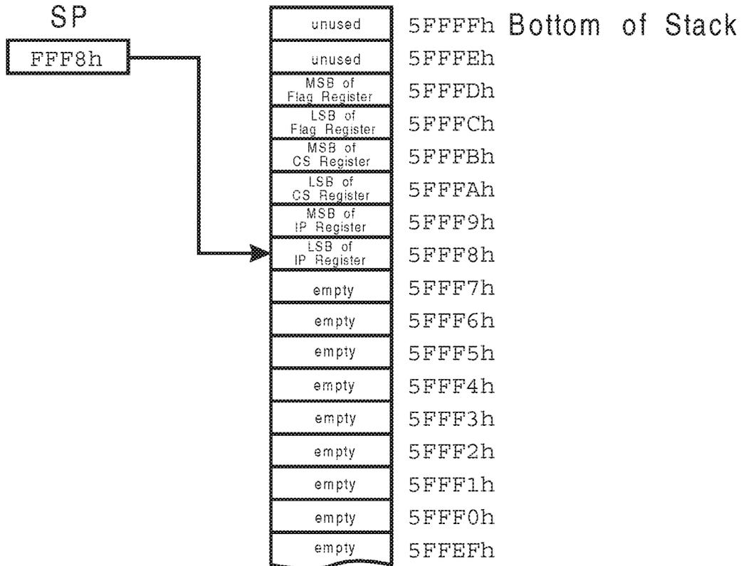
Figure 18-7. Stack After IP Register Push Operation
