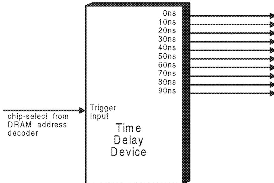
*Figure 13-3. The Time Delay Device*
