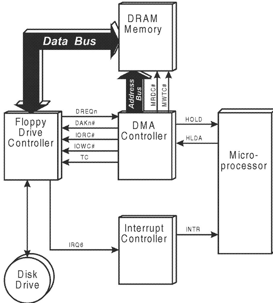
Figure 19-1. Example Disk/DMA Hardware System
