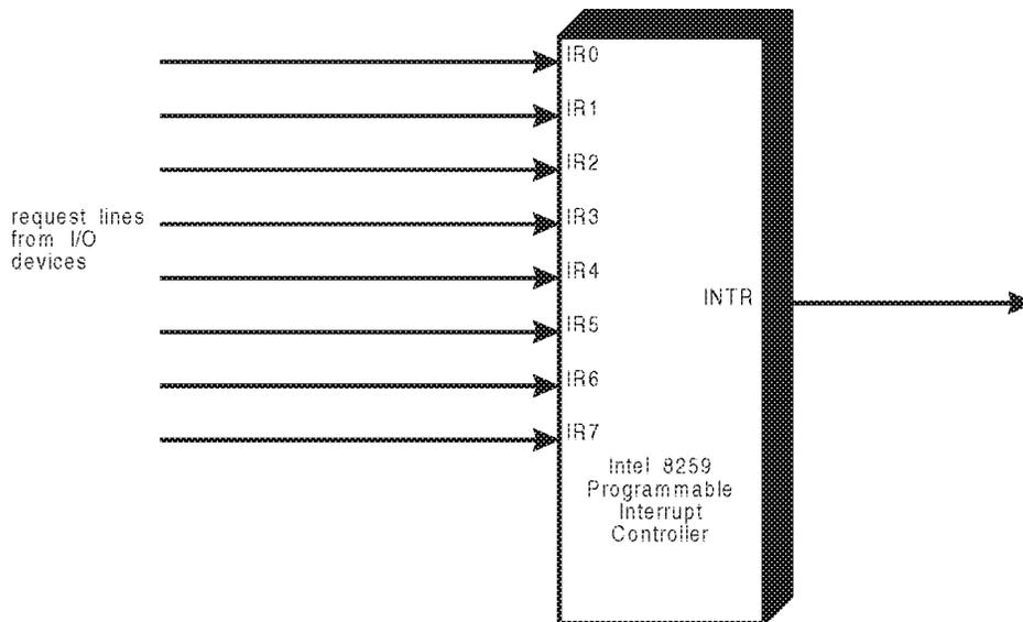
*Figure 18-2. The Intel 8259 Programmable Interrupt Controller (PIC)*
