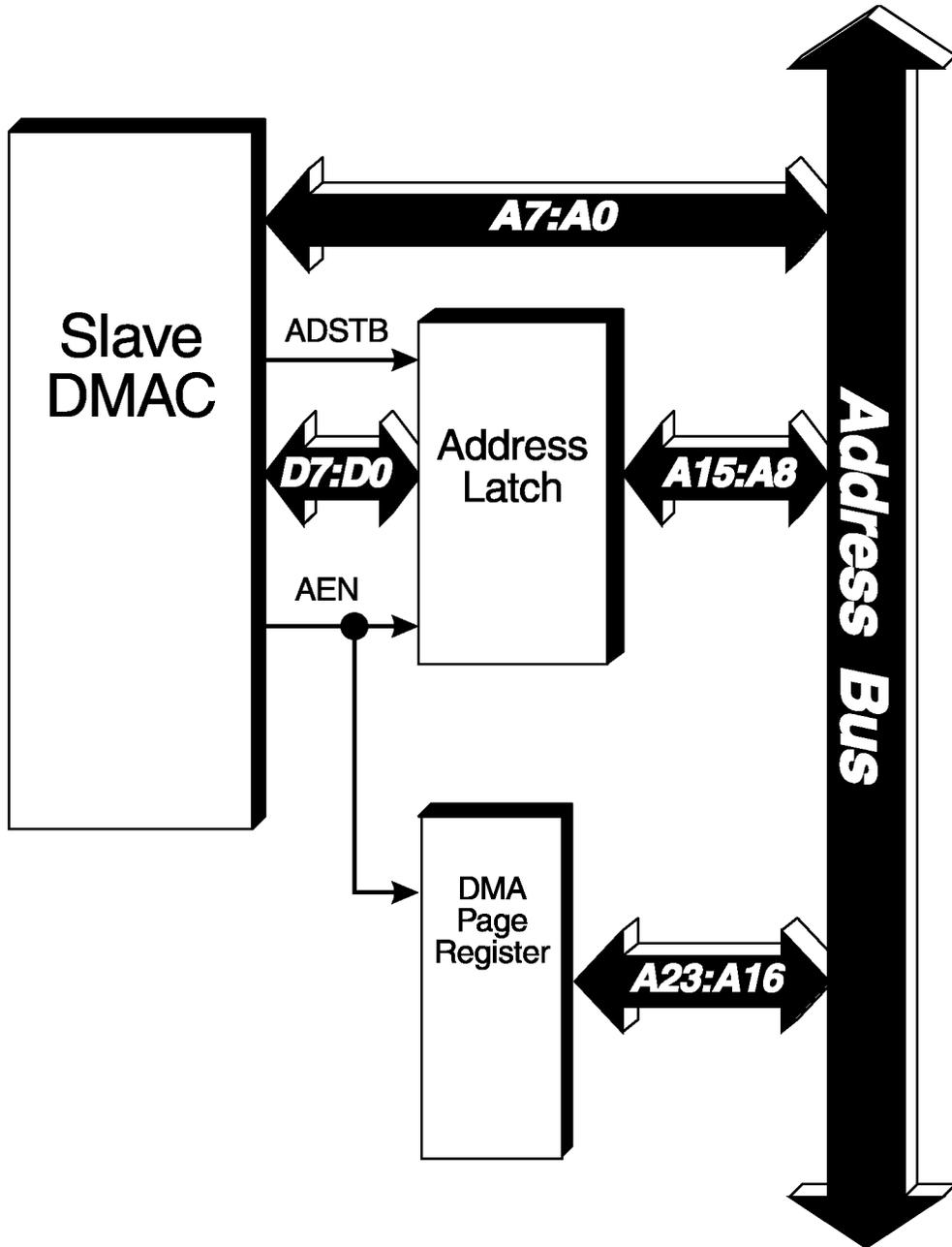
Figure 19-4. The Slave DMAC Memory Address Logic
