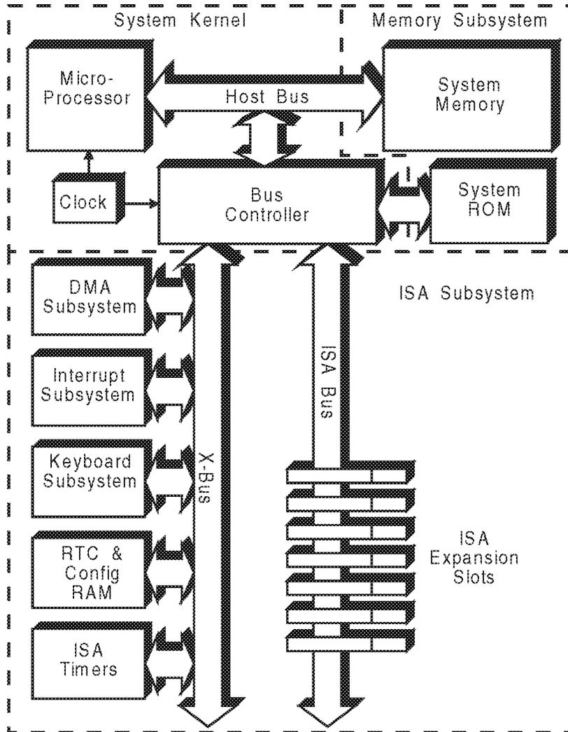
Figure 1. Simplified Block Diagram of Typical ISA System
