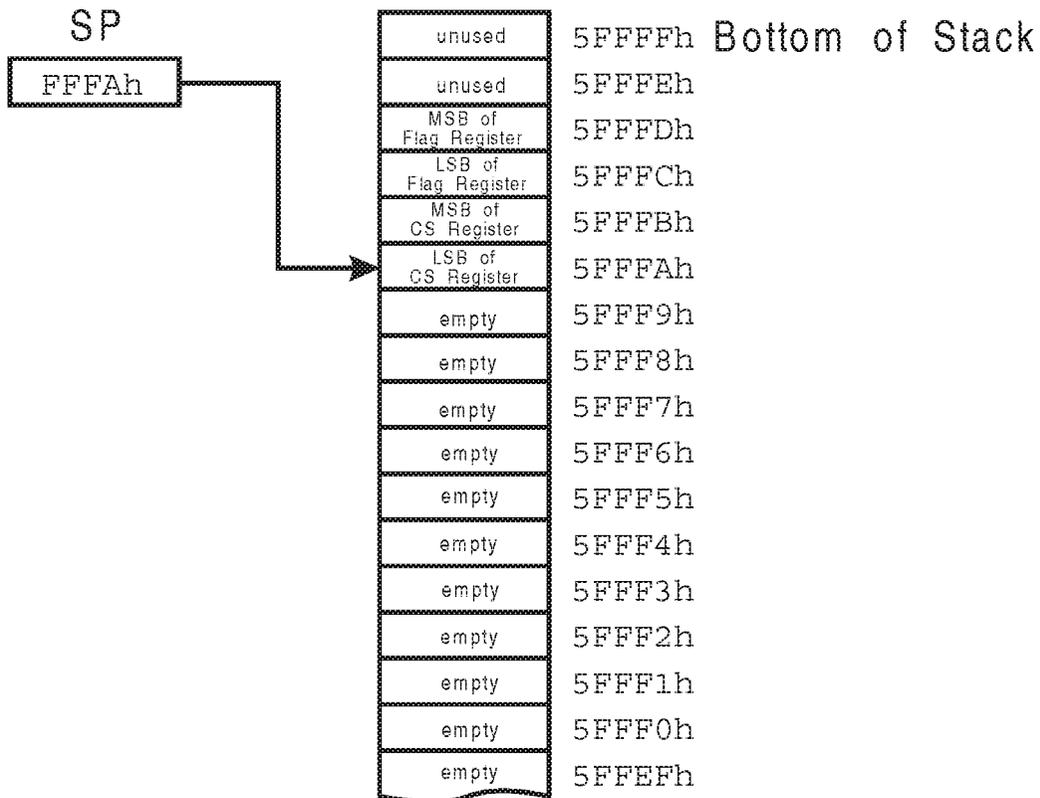
Figure 18-6. Stack After CS Register Push Operation
