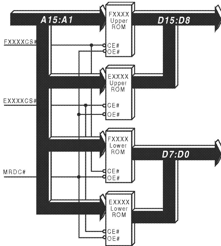
Figure 15-5. System Board ROM Configuration with 32KB ROMs
