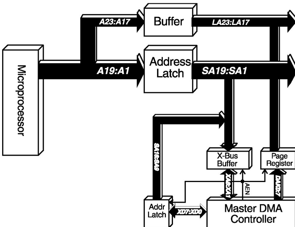
Figure 19-6. Master DMAC Addressing 16-bit ISA Memory
