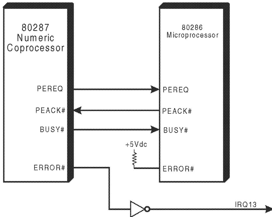
Figure 23-1. The 80287 Numeric Coprocessor
