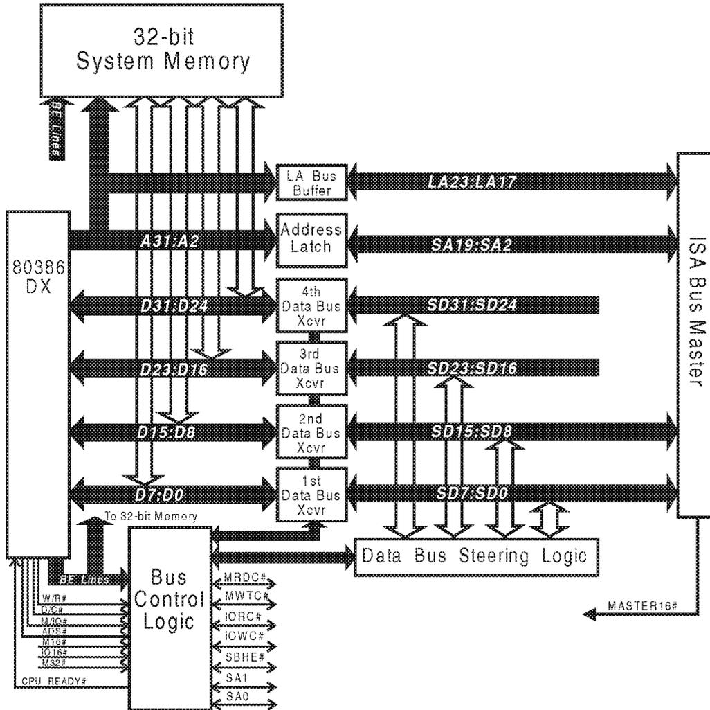
Figure 20-2. ISA Bus Master Addressing 32-bit System Memory
