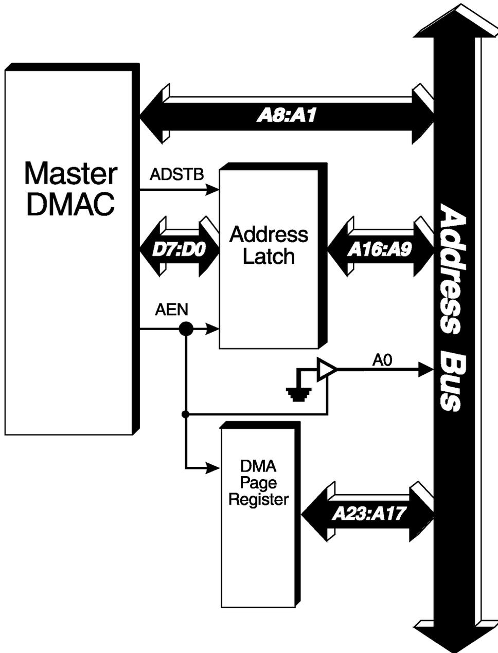
Figure 19-5. The Master DMAC Memory Address Logic
