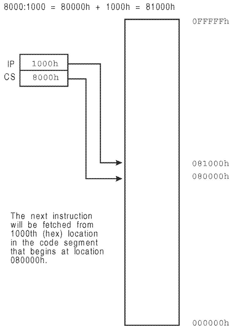
*Figure 5-8. CS and IP Registers*
