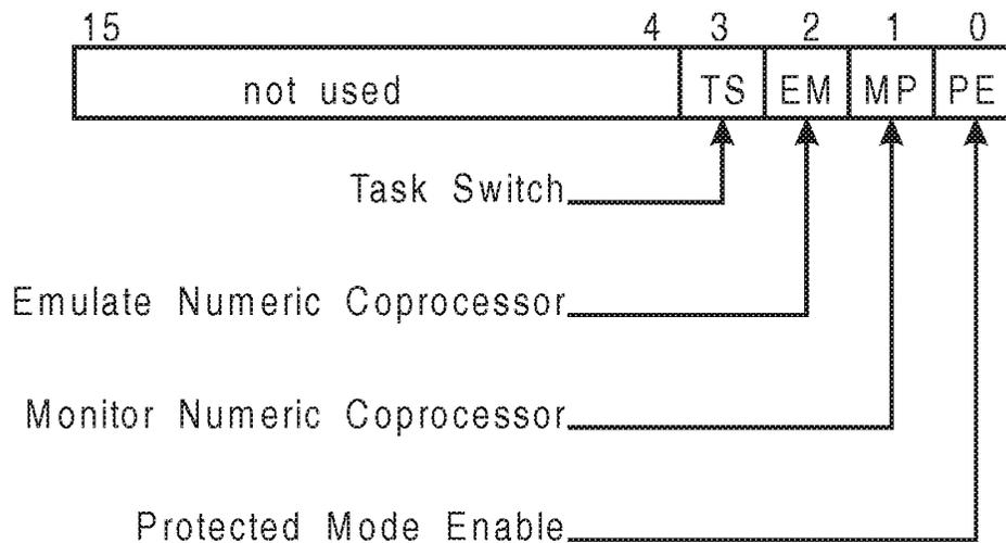
Figure 5-5. The 80286 Machine Status Word (MSW) Register
