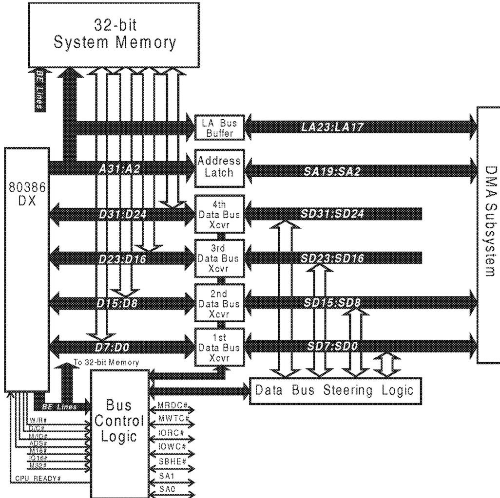
Figure 19-7. DMA (16-bit channel) Addressing 32-bit System Memory
