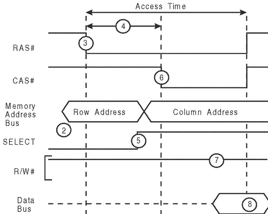
Figure 13-5. DRAM Addressing Timing Diagram
