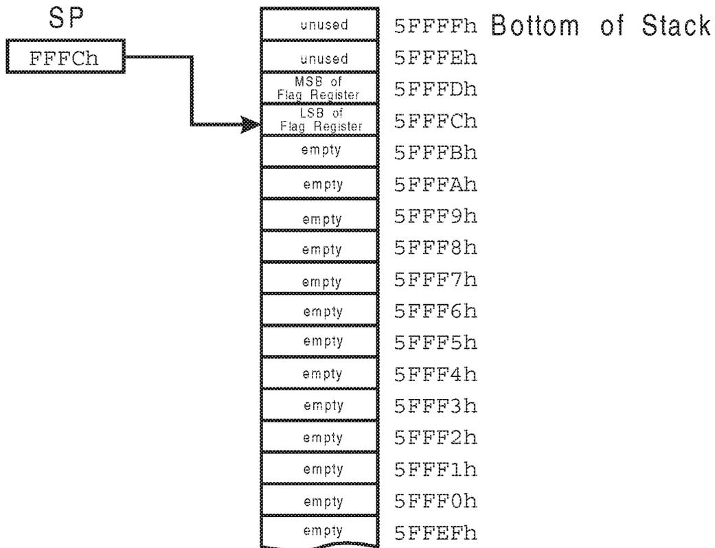
Figure 18-5. Stack After Flag Register Push Operation
