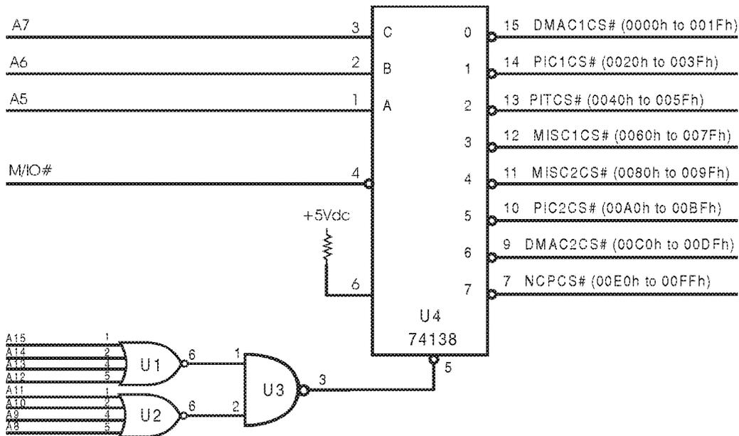
Figure 4-4. System Board I/O Address Decoder
