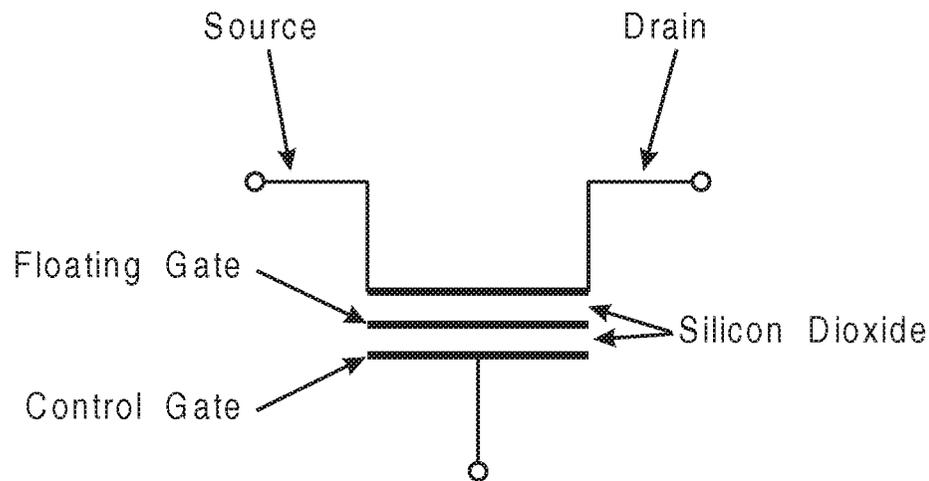
*Figure 15-3. The EPROM Bit Cell*
