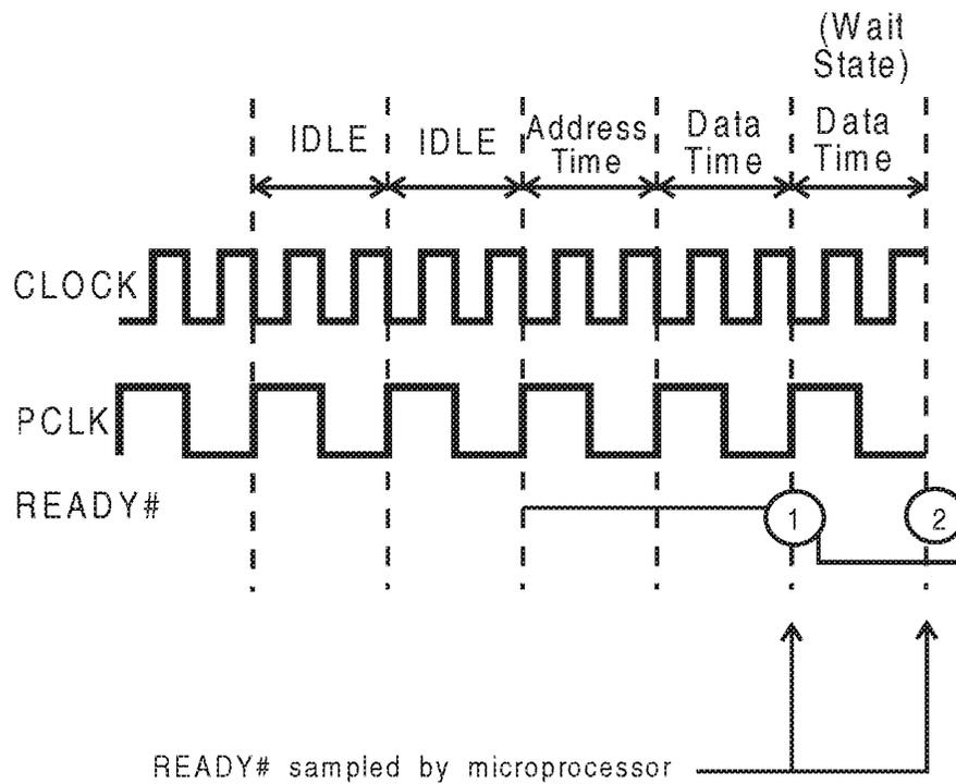
Figure 2-5. Bus Cycle with One Wait State Inserted
