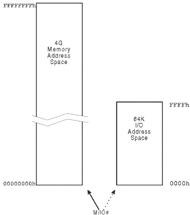
Figure 3-5. 386/486/Pentium Processor Memory and I/O Address Space
