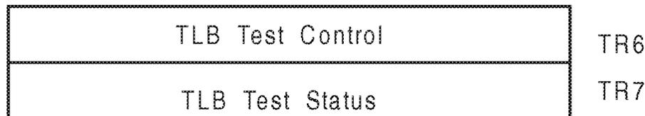
Figure 10-5. The 80386 Test Registers
