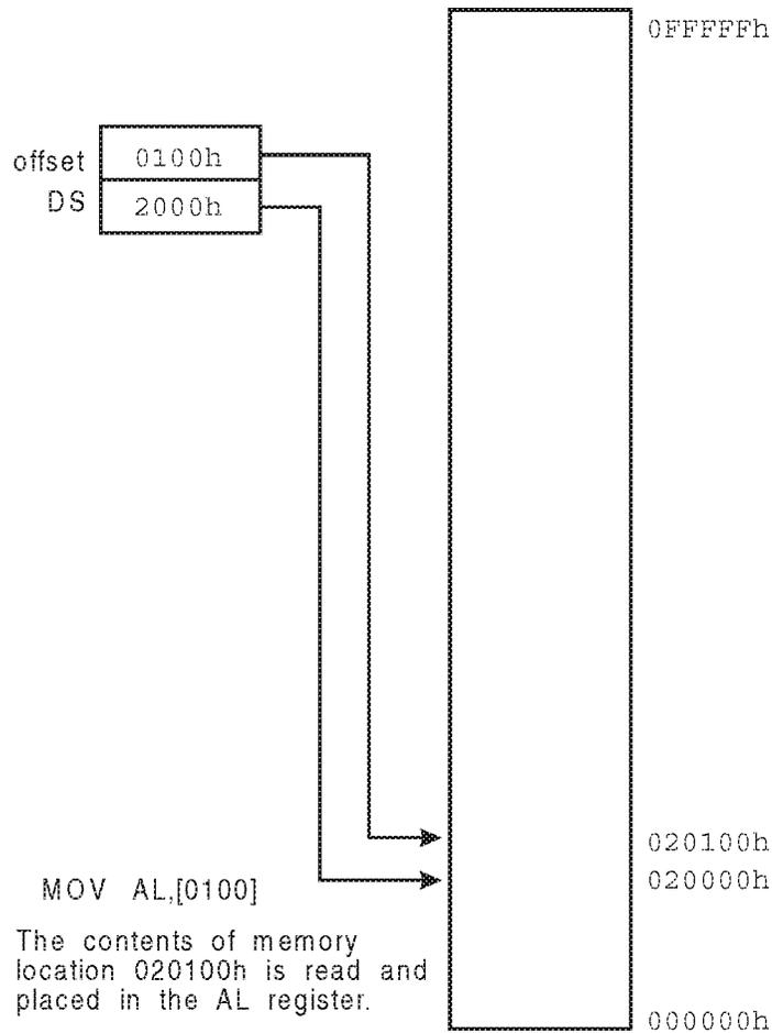
Figure 5-9. Illustration of Location within the Data Segment
