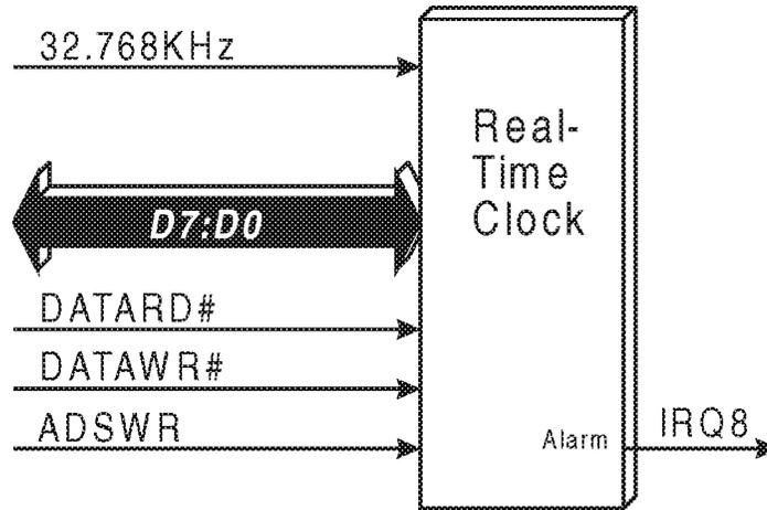
Figure 21-1. The RTC/Configuration RAM Chip
