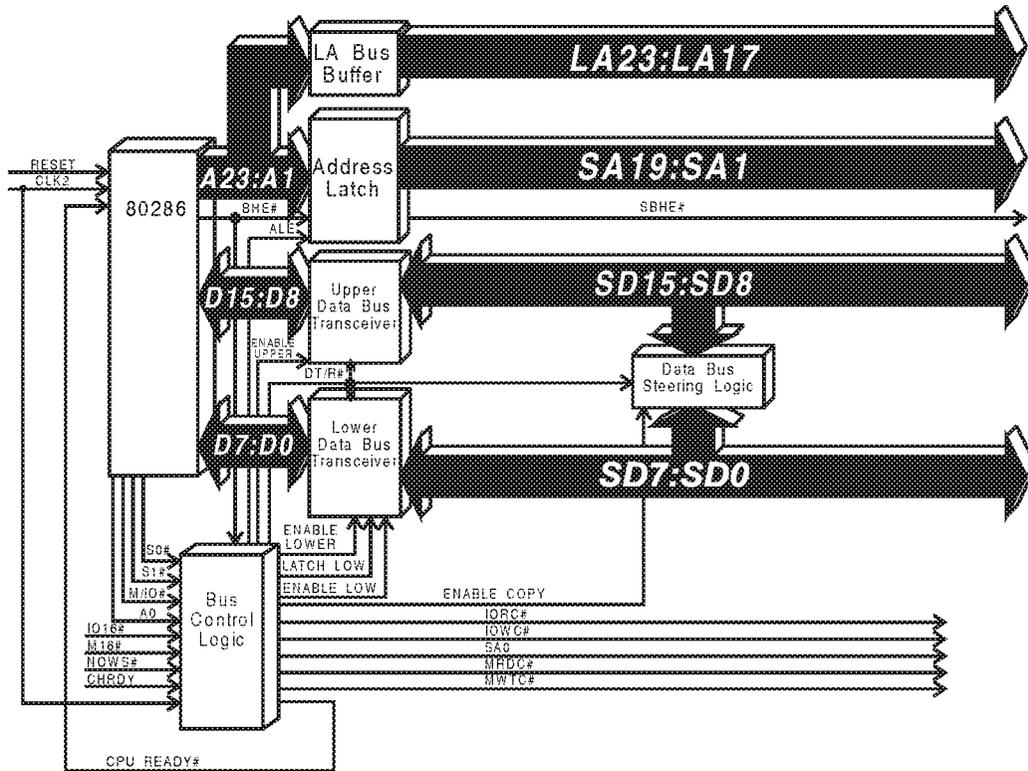
Figure 9-2. The 80286 System Engine
