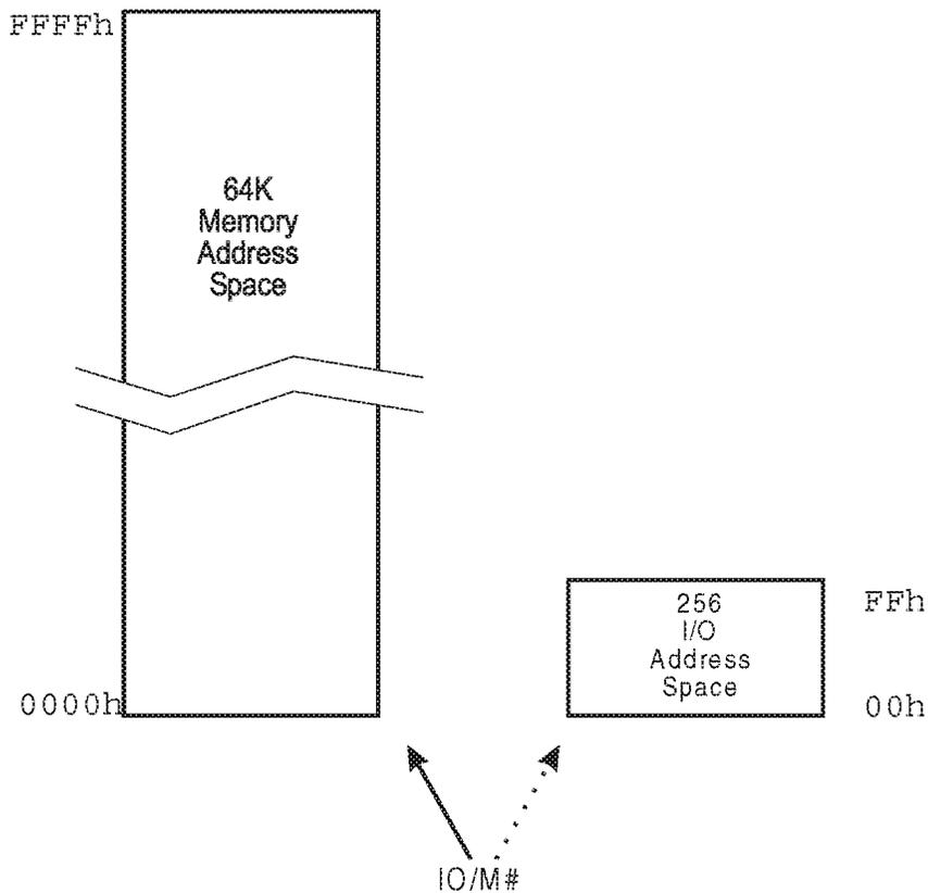
Figure 3-2. The 8085's Memory and I/O Address Spaces
