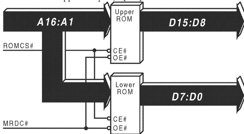
Figure 15-6. System Board ROM Configuration with 64KB ROMs
