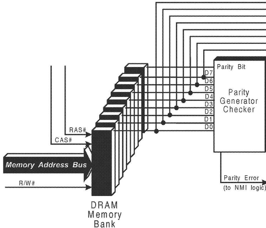
Figure 13-11. The System Board DRAM Parity Logic
