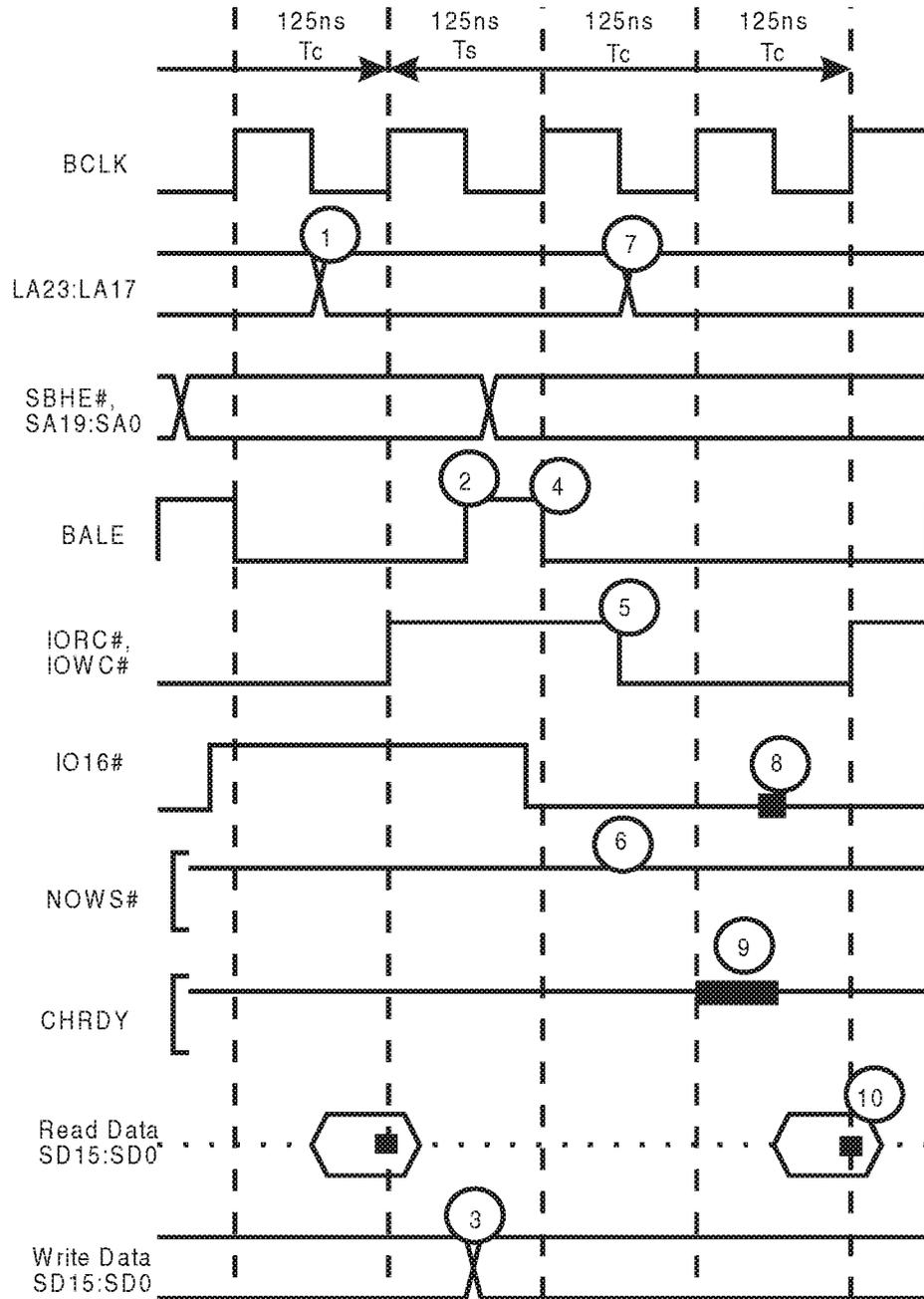
Figure 17-3. Standard Access to 16-bit I/O device
