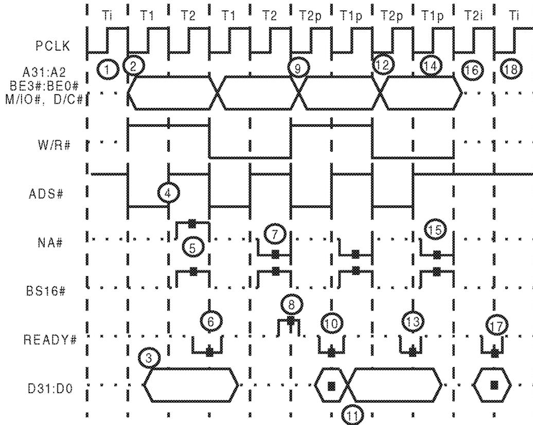
Figure 12-3. Transition from Non-Pipelined to Pipelined Operation
