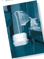
Notice how this cantilever beam deflects when loaded through the centroid (above) and through the shear center (below).
