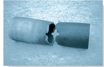
Failure of this steel pipe in tension occurred at its smallest cross-sectional area, which is through the hole. Notice how the material yielded around the fractured surface.
