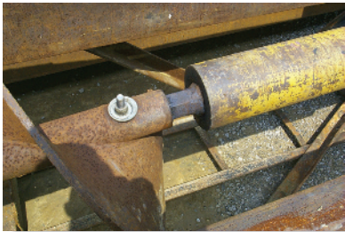
The shaft connected to the soil auger has a square cross section.
