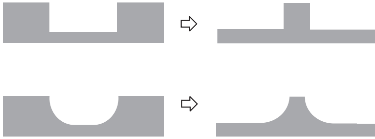
Figure 2.16 Examples of isolated positive features produced by regions of empty space.
