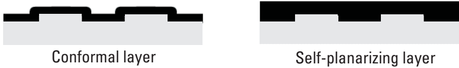
Figure 7.3 Self-planarizing layer compared to a conformal layer.
