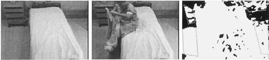
Figure 7: Experimental result on patient monitoring video WITHOUT illumination invariance function. The left panel shows a snapshot of the monitoring unit before the patient’s occupancy. The middle panel shows a sample video frame at the presence of patient. The right panel shows the detected CDM by the proposed method without concerning illumination variation. It is seen that the CDM was affected by the illumination change, for instance, the marked polygonal regions in the background area.
