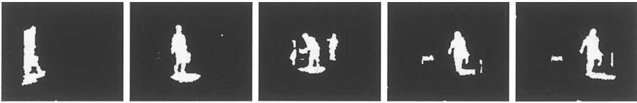
Figure 5: The detected CDM's from the sample frames of Hallway sequence, with the parameter values listed in 1. The white ("1-pixel") regions denote "there are significant changes between the test image (containing moving objects) and the reference image (containing merely background scene)". It is seen that the significant changes caused by the moving subjects and the suitcase being placed in the hallway were well identified.
