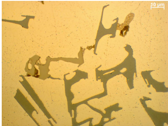
Fig. 5 Microstructure of the cast aluminium AlSi9Cu in its cast state
