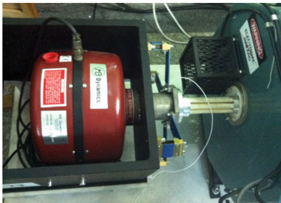
Fig. 2 Combined assembly with cryofurnace
