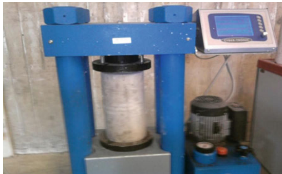
Photograph 1 Compression test set up
