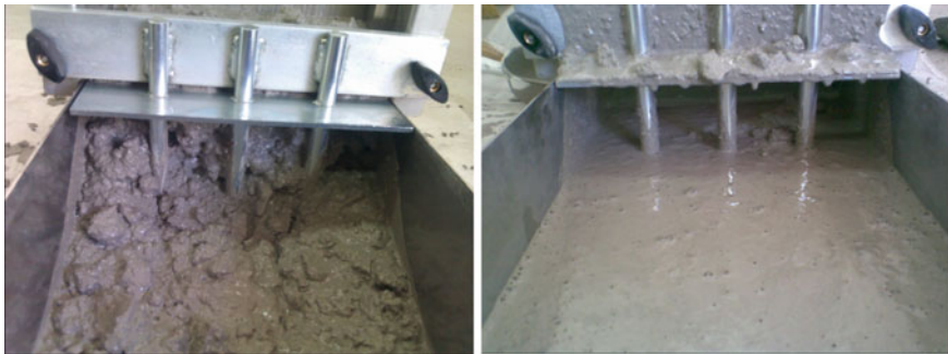
Fig. 8 Aggregate blocking on bars when the mixture C3 was tested (left) and water segregation without aggregate blocking when mixture C3S5 was tested (right)
