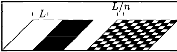
Fig. 3.9. The dissipation time of the magnetic field decreases as the spatial scales decrease
