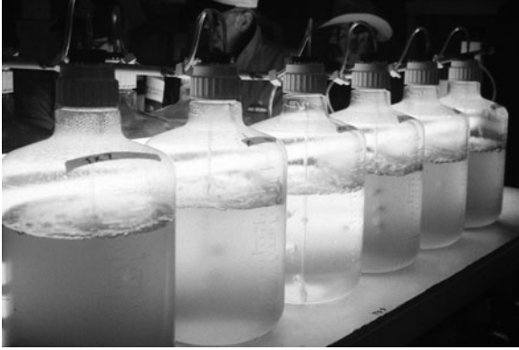
Fig. 2.19. Algal culture carboys. The carboy on the left has a dense concentration of cells and is nearly ready for harvest, while those to the right contain cultures in the early stages of growth.
