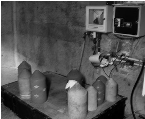
Fig. 2.36. The torpedo-shaped objects are called pigs, and are forced through water lines to scour out fouling organisms at the Monterey Bay Aquarium in Monterey, California, USA.
