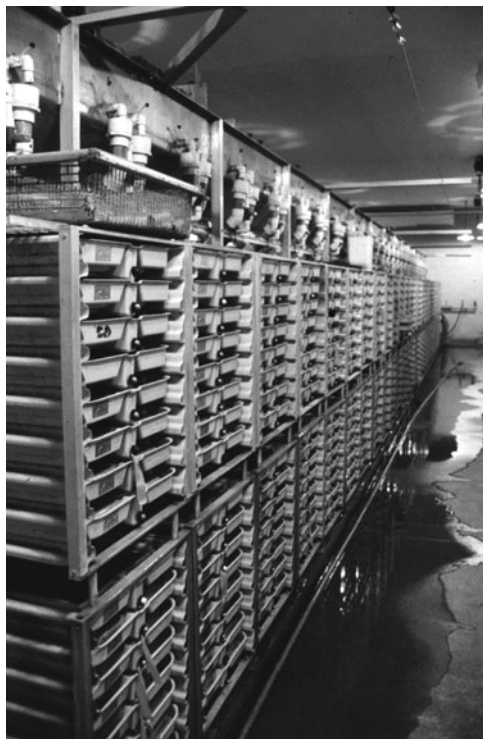
Fig. 3.12. A battery of Heath incubators used for hatching salmon eggs. The eggs are placed in drawers out of direct light. Oxygen-rich water is flowed into each stack of trays at the top and trickles down the stack, so the eggs are constantly submerged in high-quality water.
