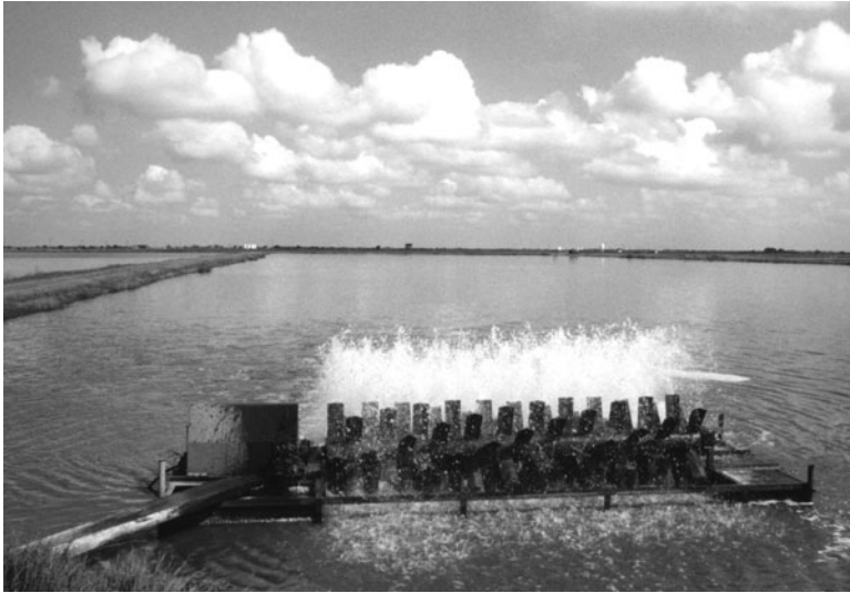
Fig. 3.3. A paddlewheel aerator in action.
