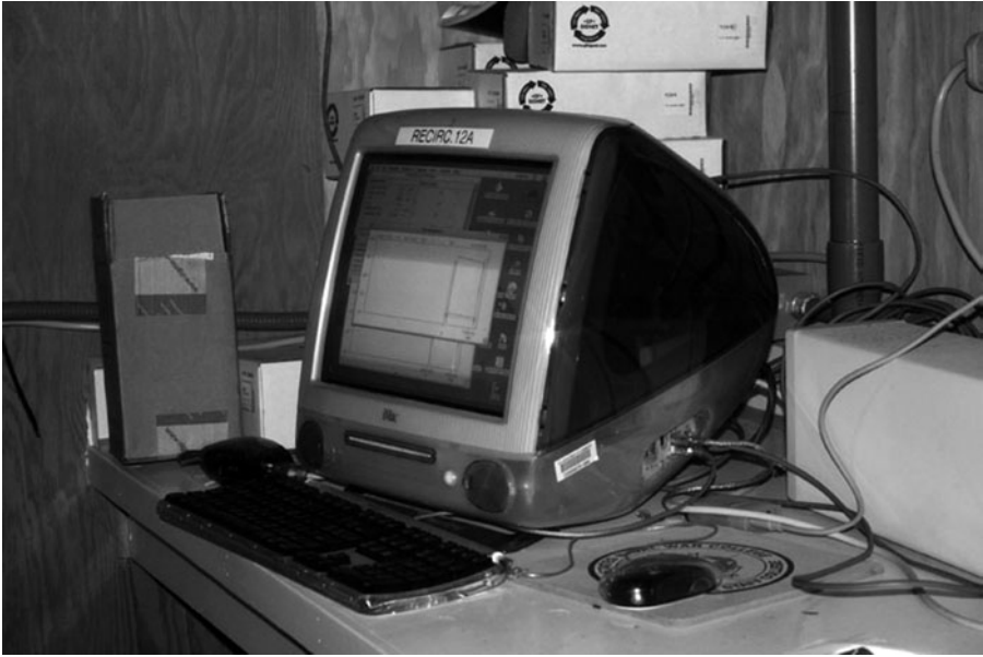
Fig. 1.1. Computers are often used to control water flow rates and collect data on water quality in modern aquaculture facilities.
