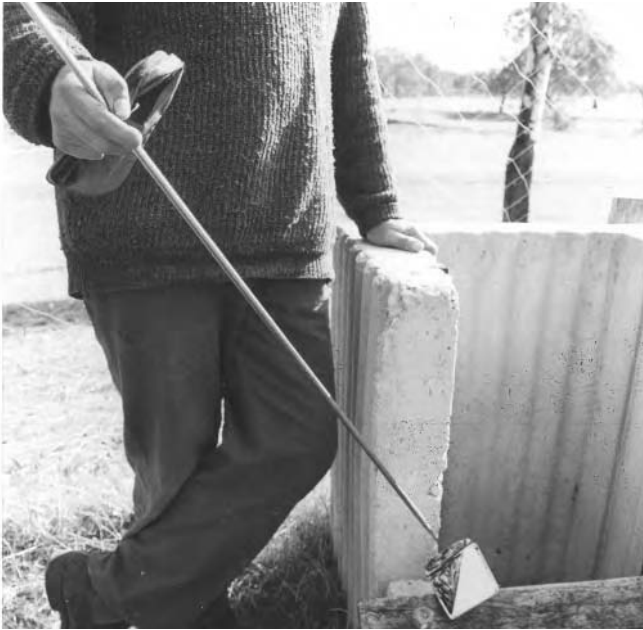
Figure 12.2. A simple farm-made Secchi disc.
