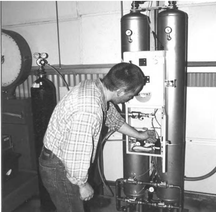
Figure 8.1. Oxygen can be raised to supersaturation levels in re-circulation systems by separating O_2 from the atmosphere and injecting it into the water used in the production tanks. Here an operator is shown adjusting the O_2 generator. An oxygen storage bottle can be seen in the background. The line going off to the right is taking pure oxygen to the pressure tank where it is mixed with the production water.
