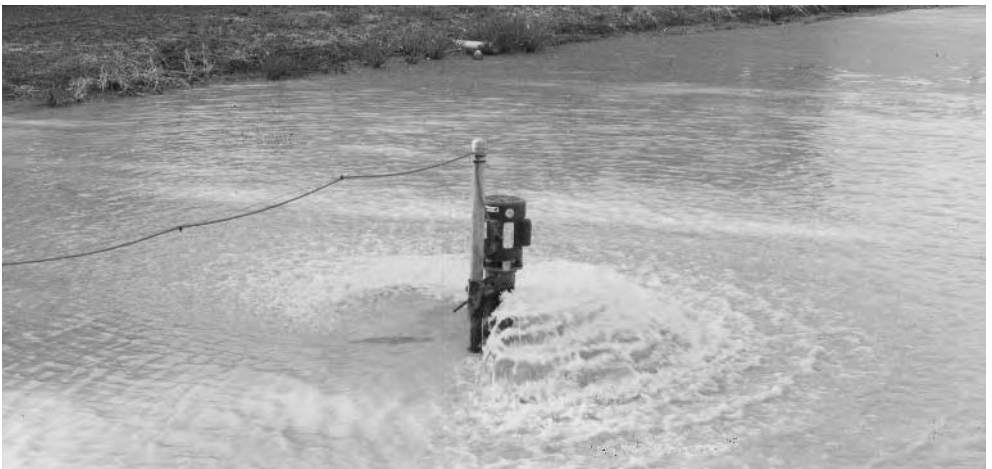
Figure 12.6. Simple farm-built devices are just as effective and will be a lot cheaper to build. However, a warning: it's not that water and electricity are bad mixers; the trouble is that they are very good mixers. Any electrical short that finds its way into the water will electrify the water which can be fatal to humans.
