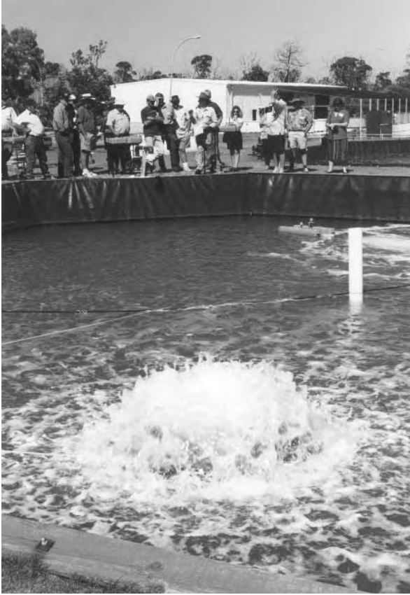
Figure 12.4. Aerator manufacturers compete for buyers' attention at an aquaculture conference and trade show in south-east Queensland. In the foreground can be seen a propeller-driven water lifter while in the background an air injector is at work.
