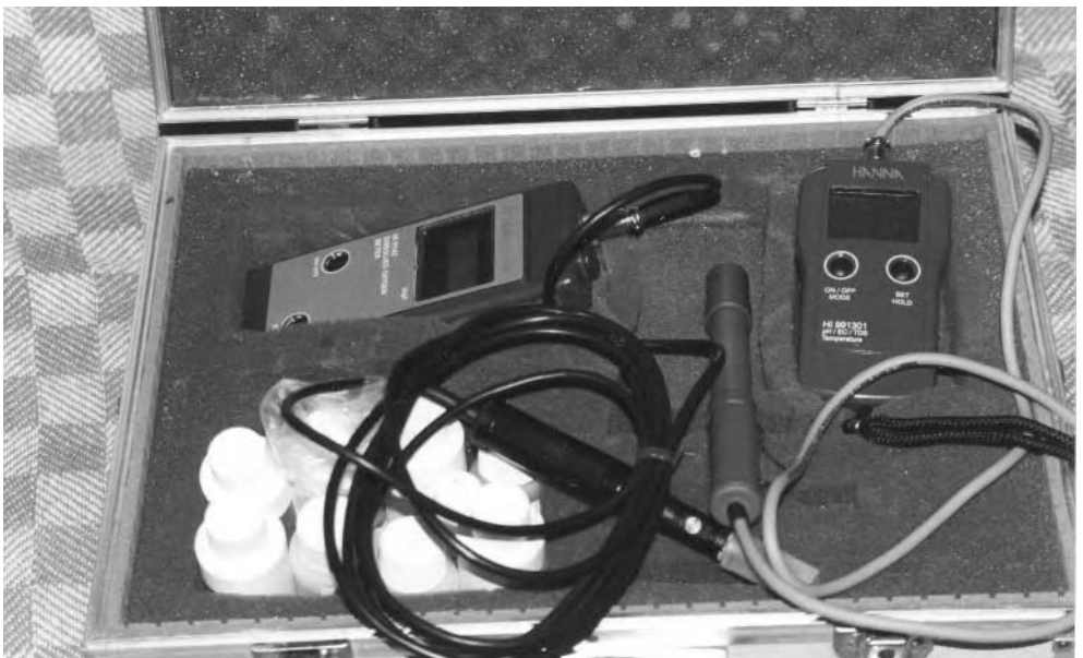
Figure 12.1. DO and pH meters are essential parameter measuring aids that will pay for themselves a thousand times the first time they save a crop.
