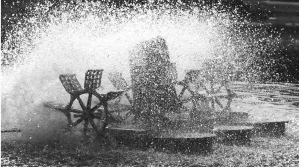
Figure 12.5. Paddlewheel aerators throw a continuous spray of small water particles into the air where the droplets interface with the atmosphere. This process allows the water to expel carbon dioxide and take on oxygen up to saturation level.
