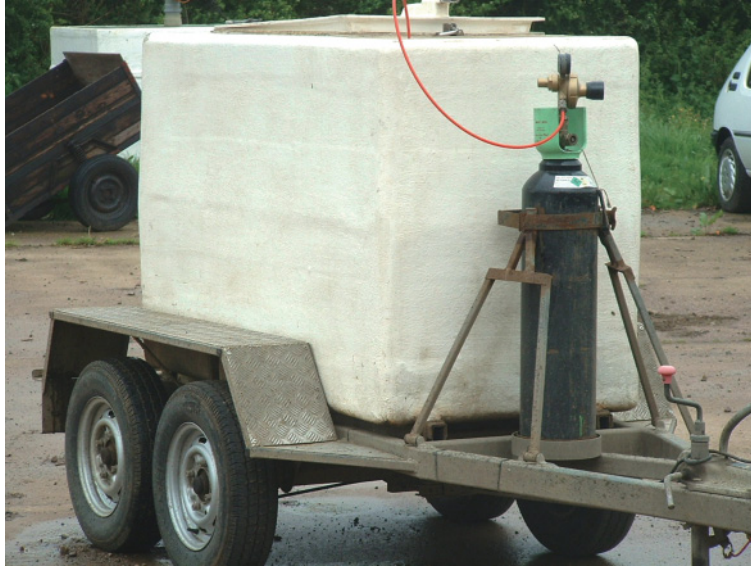
Figure 12.5 Simple closed system for the transport of live fish.
