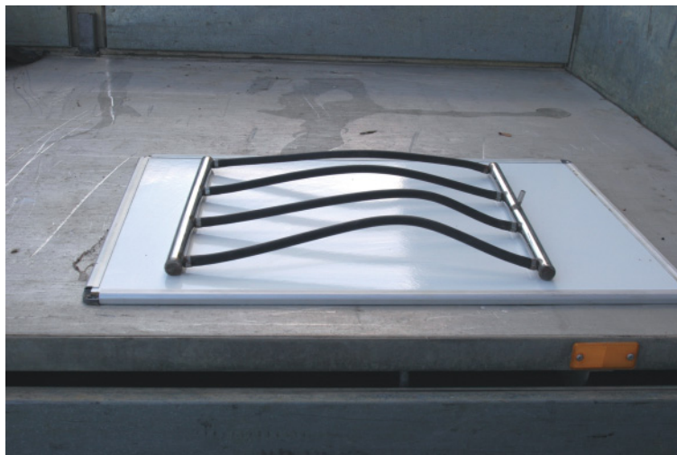
Figure 12.7 Leaky pipe diffuser.
