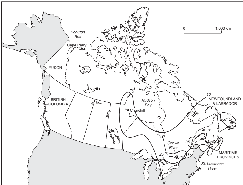
FIG. 6 Spatial distribution of climatological annual freezing rain hours in Canada. (From Stuart and Isaac [1999], reproduced here with authors' permission.)
