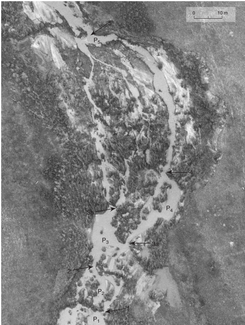
FIG. 16 Expanded view of Reach B. The major dams on this figure are labeled with numbers from 1 to 5, starting upstream. The pre-flood ponds are labeled in association with the dams as P1 through P5. Despite being just downstream of Reach A, the relatively dense woody vegetation associated with the numerous beaver ponds protected the floodplain. Although most of the beaver dams are breached, these breaches are small and would have been quickly repaired once the floodwaters receded a little further. Note that the flow resistance was so high in this bend from the presence of the mature willows that none of the geomorphic structures typical of bends are displayed at this location. The flow did not even erode the “cut” bank. There is some deposition of sand in the willow carr at the downstream end of the bend resulting from flow deceleration through the shrubs.
