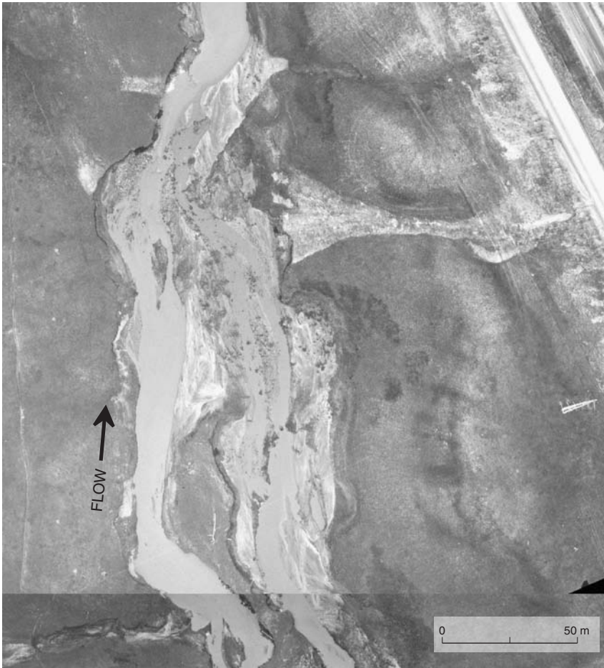
FIG. 19 Expanded view of Reach F showing the confluence of the larger unnamed tributary and Carpenter Creek. Gravel can be seen emanating from an eddy-caused cut in the bank at the center of the figure. Upstream of this location there is evidence of only sand on the bottom of the channel. Similarly, there is only sand in the channel of Carpenter Creek upstream of the confluence. This reach of the unnamed tributary has fully unraveled, but the gravel has prevented it from evolving a flood-related hydraulic geometry. Also, the gravel has disrupted the flood-related hydraulic geometry of Carpenter Creek for a short distance downstream of the confluence. The notches in the banks of both creeks are a result of recirculation zones and that the fluid mechanics of the confluence was complex.
