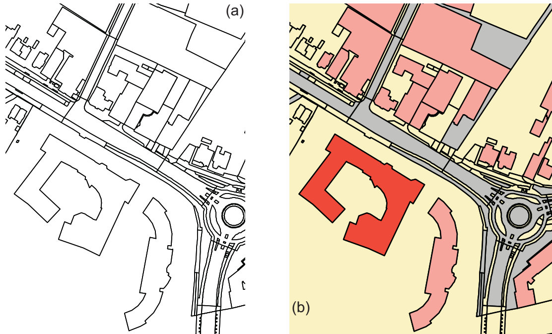
Figure 6.22: Visual hierarchy and the location of the ITC building: (a) hierarchy not applied; (b) hierarchy applied
