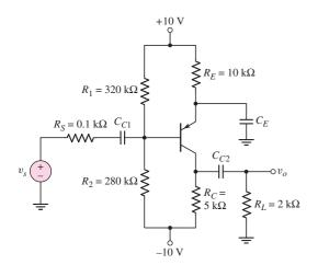
**Figure 7.30** Circuit with two coupling capacitors and an emitter bypass capacitor
