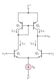
Figure 14.18 Basic bipolar diff-amp with active load
