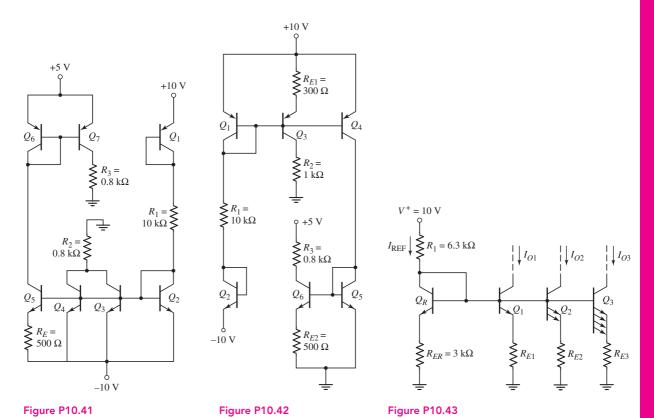
\*D10.43 Consider the circuit in Figure P10.43. The transistor parameters are:  $\beta = \infty$ ,  $V_A = \infty$ , and  $V_{BE} = 0.7$  V. Design the circuit such that the B–E voltages of  $Q_1$ ,  $Q_2$ , and  $Q_3$  are identical to that of  $Q_R$ . What are the values of  $I_{O1}$ ,  $I_{O2}$ , and  $I_{O3}$ ?
