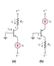
Figure 5.11 Common-base circuit configuration with constant current source biasing: (a) an npn transistor and (b) a pnp transistor
