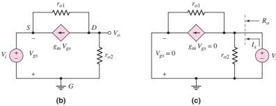
Figure 4.48 (a) CMOS common-gate amplifier, (b) small-signal equivalent circuit, and (c) small-signal equivalent circuit for determining the output resistance
