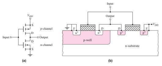
Figure 16.22 Simplified cross section, CMOS inverter
