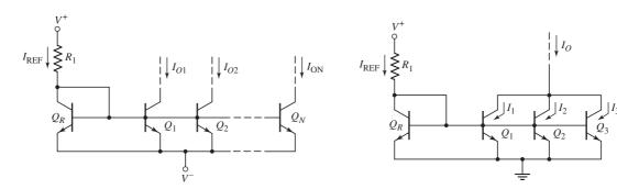
Figure 10.12 Multitransistor current mirror
