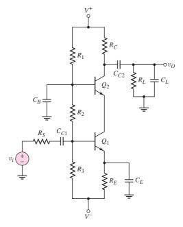
Figure 7.65 Cascode circuit
