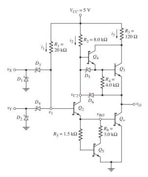
Figure 17.34 Low-power Schottky TTL NAND logic circuit
