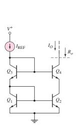
Figure 11.41 Bipolar cascode constant-current source
