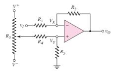
Figure 14.20 Offset voltage compensation circuit for inverting amplifier
