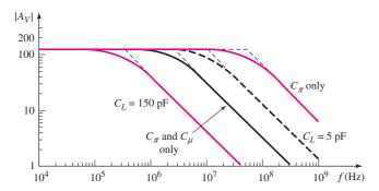
Figure 7.59 PSpice analysis results for common-emitter amplifier
