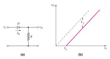
Figure 2.33 Diode and resistor in series: (a) circuit and (b) voltage transfer characteristics
