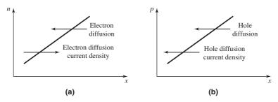
Figure 1.9 (a) Assumed electron concentration versus distance in a semiconductor, and the resulting electron diffusion and electron diffusion current density, (b) assumed hole concentration versus distance in a semiconductor, and the resulting hole diffusion and hole diffusion current density
