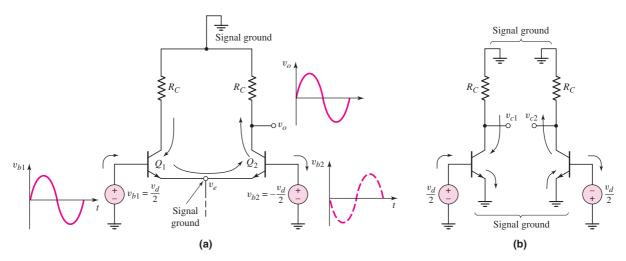
Figure 11.12 (a) Equivalent ac circuit, diff-amp with applied sinusoidal differential-mode input signal, and resulting signal current directions and (b) differential-mode half-circuits
