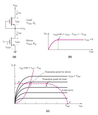
Figure 16.7 (a) NMOS inverter with depletion load, (b) current–voltage characteristic of depletion load, and (c) driver transistor characteristics and load curve
