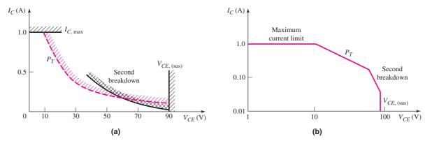
Figure 8.3 The safe operating area of a bipolar transistor plotted on: (a) linear scales and (b) logarithmic scales
