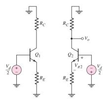
Figure 11.18 Differential half-circuits with emitter degeneration
