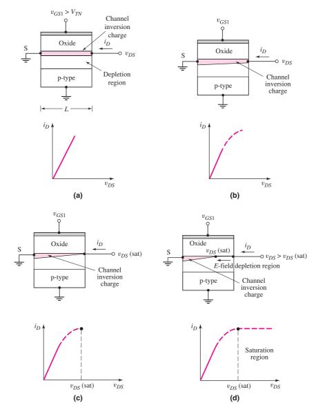
Figure 3.9 Cross section and  $i_D$  versus  $v_{DS}$  curve for an n-channel enhancement-mode MOSFET when  $v_{GS} > V_{TN}$  for (a) a small  $v_{DS}$  value, (b) a larger  $v_{DS}$  value but for  $v_{DS} < v_{DS}(\text{sat})$ , (c)  $v_{DS} = v_{DS}(\text{sat})$ , and (d)  $v_{DS} > v_{DS}(\text{sat})$
