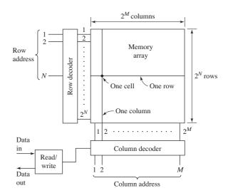
Figure 16.71 Basic random access memory architecture
