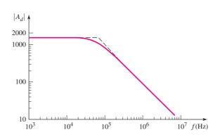
Figure 11.58 PSpice results for frequency response of diff-amp with active load and single-sided input
