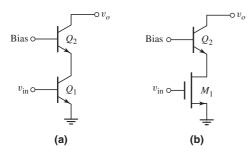
Figure 11.40 (a) Bipolar cascode configuration and (b) BiCMOS cascode configuration
