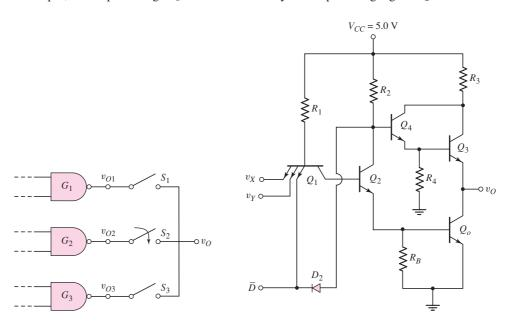
Figure 17.28 Circuit symbolically showing tristate output
