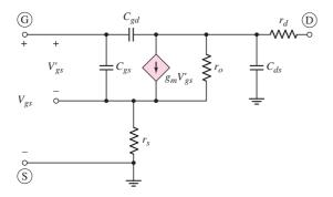
Figure 7.50 Equivalent circuit of the n-channel common-source MOSFET
