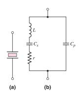
Figure 15.22 (a) Piezoelectric crystal circuit symbol and (b) piezoelectric crystal equivalent circuit
