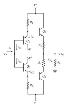
Figure 8.34 Class-AB output stage with input buffer transistors
