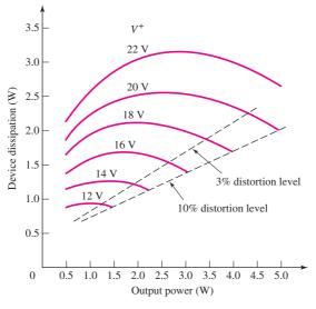
Figure 15.44 LM380 power amplifier characteristics
