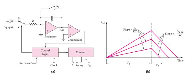
Figure 16.95 (a) Block diagram and (b) timing diagram of a dual-slope A/D converter
