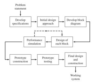
Figure PR2.3 Flowchart of the design process
