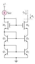
Figure 11.42 BiCMOS double cascode constant-current source
