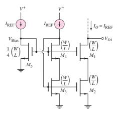
Figure 10.21 A wide-swing MOSFET cascode current mirror
