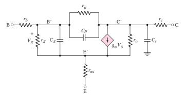
Figure 7.37 Hybrid- $\pi$  equivalent circuit
