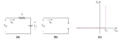
Figure 1.31 The diode piecewise equivalent circuit (a) in the "on" condition when  $V_D \ge V_{\gamma}$ , (b) in the "off" condition when  $V_D < V_{\gamma}$ , and (c) piecewise linear approximation when  $r_f = 0$ . When  $r_f = 0$ , the voltage across the diode is a constant at  $V_D = V_{\gamma}$  when the diode is conducting.
