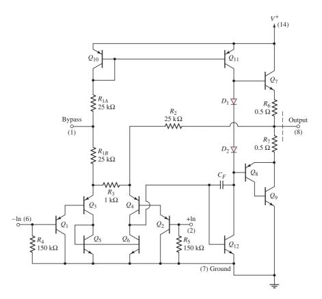
Figure 15.42 The LM380 power amplifier
