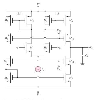
Figure 13.19 CMOS cascode current-mirror op-amp
