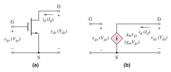
Figure 4.5 (a) Common-source NMOS transistor with small-signal parameters and (b) simplified small-signal equivalent circuit for NMOS transistor
