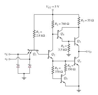
Figure 17.33 Schottky TTL NAND logic circuit
