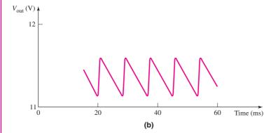
**Figure 2.12** (a) PSpice circuit schematic of diode bridge circuit with an RC filter; (b) Steady-state output voltage of PSpice analysis of diode bridge circuit for a 60 Hz input sine wave with a peak value of 13.4 V
