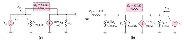
Figure 12.40 Small-signal equivalent circuits of the circuit in Figure 12.37(a) for calculating (a) input resistance and (b) output resistance
