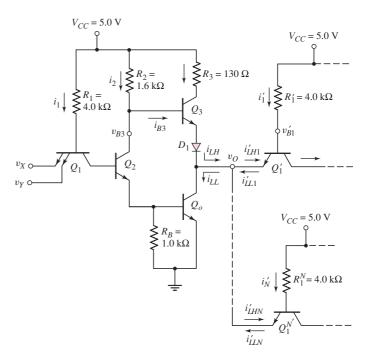
Figure 17.25 TTL circuit with totem-pole output stage
