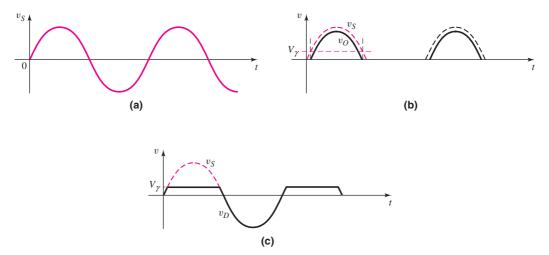
Figure 2.3 Signals of the half-wave rectifier circuit: (a) sinusoidal input voltage, (b) rectified output voltage, and (c) diode voltage
