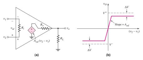
Figure 9.7 (a) Equivalent circuit of the op-amp and (b) simplified voltage transfer characteristic
