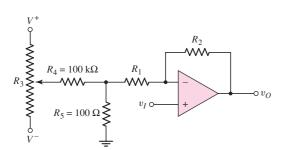
Figure 14.21 Offset voltage compensation circuit for noninverting amplifier
