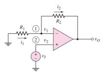
Figure 9.15 Noninverting op-amp circuit
