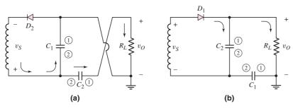
Figure 2.15 Equivalent circuit of the voltage doubler circuit: (a) negative input cycle and (b) positive input cycle
