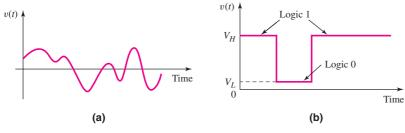
Figure PR1.2 Graphs of analog and digital signals: (a) analog signal versus time and (b) digital signal versus time
