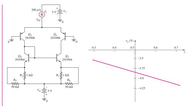
**Figure 14.23** Circuit used in the computer simulation analysis for Example 14.12
