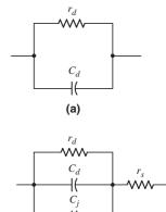
Figure 1.38 Small-signal equivalent circuit of the diode: (a) simplified version and (b) complete circuit
