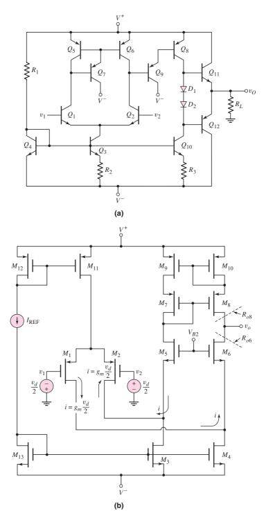
Figure 14.1 (a) Simple all-bipolar op-amp circuit; (b) all-CMOS folded cascode op-amp circuit
