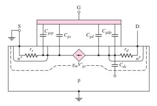
Figure 7.49 Inherent resistances and capacitances in the n-channel MOSFET structure
