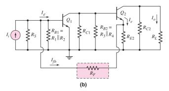
Figure 12.24 (a) Example of a discrete transistor shunt–series feedback circuit and (b) ac equivalent circuit
