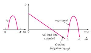
Figure 8.27 Effective ac load line of a class-C amplifier
