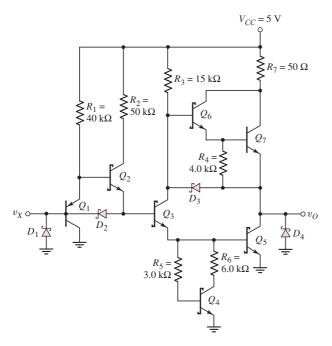
Figure 17.35 Advanced low-power Schottky (ALS) inverter gate
