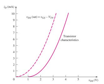
Figure 3.35 Current-voltage characteristic of an enhancement load device
