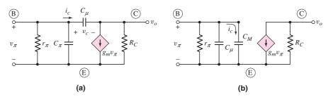
Figure 7.47 (a) Hybrid- $\pi$  equivalent circuit of a bipolar transistor with a load resistor  $R_C$  connected to the output. (b) Equivalent circuit with the Miller capacitance.
