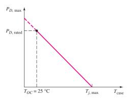
Figure 8.12 A power derating curve
