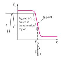
Figure 10.34 Voltage transfer characteristic of MOSFET circuit with active load
