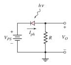
Figure 2.44 A photodiode circuit. The diode is reverse biased
