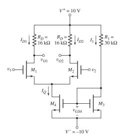
Figure 11.20 MOSFET differential amplifier for Example 11.8
