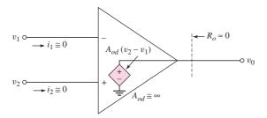
Figure 9.6 Parameters of the ideal op-amp
