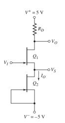
Figure 10.24 The dc equivalent circuit of simple JFET amplifier biased with JFET current source
