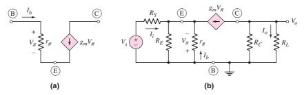
Figure 6.60 (a) Simplified hybrid- $\pi$  model of the npn transistor and (b) small-signal equivalent circuit of the common-base circuit
