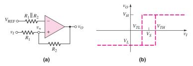
Figure 15.31 (a) Noninverting Schmitt trigger circuit with applied reference voltage and (b) voltage transfer characteristics
