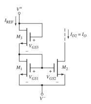
Figure 10.17 MOSFET current source
