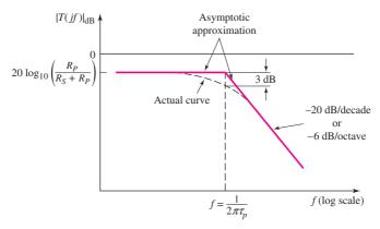
Figure 7.8 Bode plot of the voltage transfer function magnitude for the circuit in Figure 7.3
