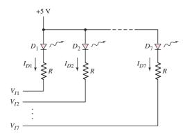
Figure 2.46 Control circuit for the seven-segment LED display
