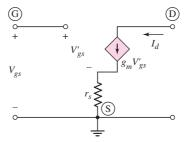
Figure 7.51 Simplified low-frequency equivalent circuit of the n-channel common-source MOSFET including source resistance  $r_s$  but not resistance  $r_o$
