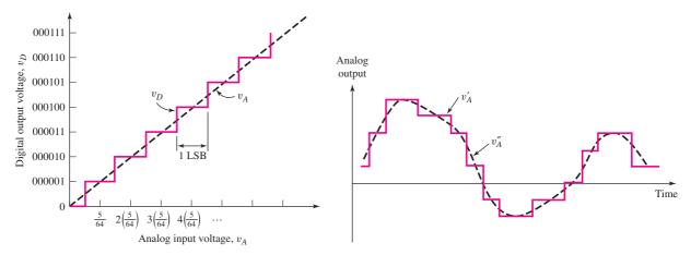
Figure 16.88 Digital output versus analog input for a 6-bit A/D converter
