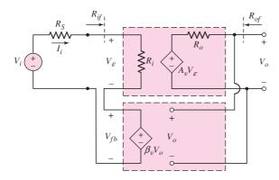
Figure 12.6 Ideal series-shunt feedback topology
