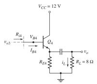
Figure 6.78 Output stage (emitter-follower) for design application
