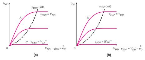
Figure 16.23 Current-voltage characteristics, (a) NMOS transistor and (b) PMOS transistor
