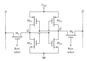
Figure 16.75 A CMOS static RAM cell
