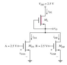
Figure 16.12 Two-input NMOS NOR logic gate for Example 16.5
