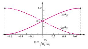
Figure 11.21 Normalized dc transfer characteristics, MOSFET differential amplifier
