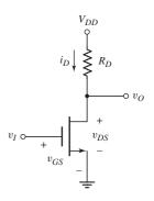
Figure 3.45 NMOS inverter circuit
