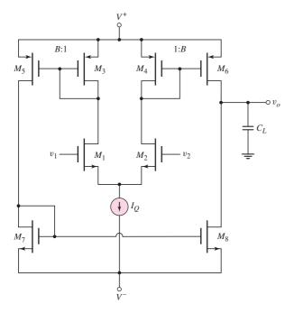
Figure 13.18 CMOS current-mirror op-amp
