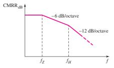
**Figure 11.54** Frequency response of common-mode rejection ratio
