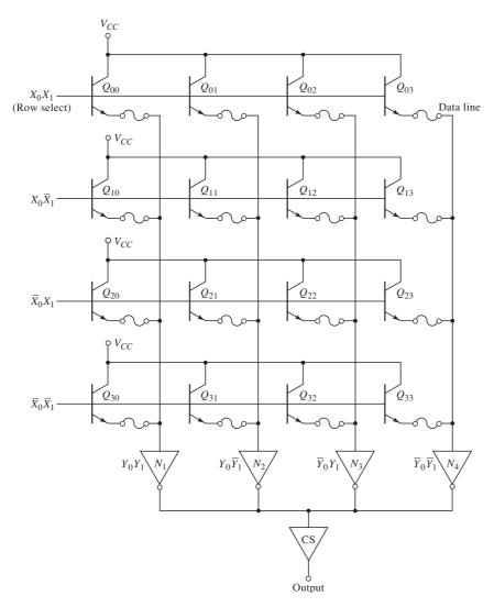
Figure 16.84 A bipolar fuse-linked user-programmable ROM
