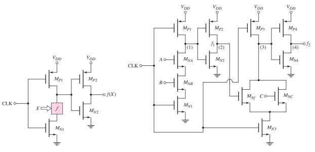
Figure 16.45 Generalized CMOS clocked logic circuit
