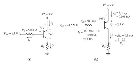
Figure 5.22 Circuit for Example 5.4; (a) circuit and (b) circuit showing current and voltage values
