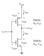
Figure 16.21 CMOS inverter
