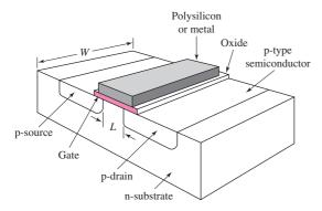
Figure 16.20 Simplified cross section of p-channel MOSFET
