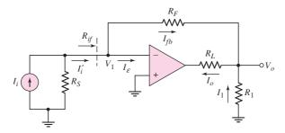
Figure 12.20 Example of an op-amp shunt-series feedback circuit
