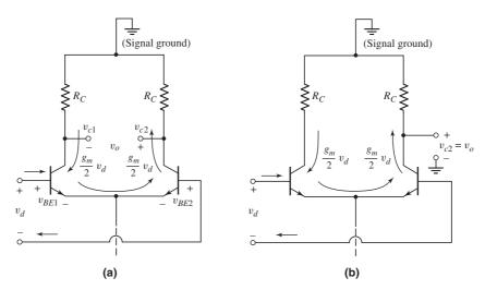
Figure 11.8 (a) Equivalent ac circuit, diff-amp with differential-mode input signal and two-sided output voltage and (b) ac equivalent circuit with one-sided output
