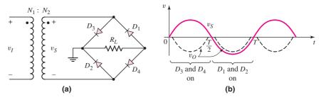
**Figure 2.7** (a) Full-wave bridge rectifier circuit to produce negative output voltages. (b) Input and output waveforms.
