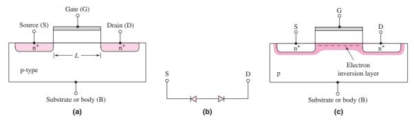
Figure 3.6 (a) Cross section of the n-channel MOSFET prior to the formation of an electron inversion layer, (b) equivalent back-to-back diodes between source and drain when the transistor is in cutoff, and (c) cross section after the formation of an electron inversion layer
