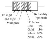
**Figure C.1** Color-band notation of low-power carbon-composition resistors
