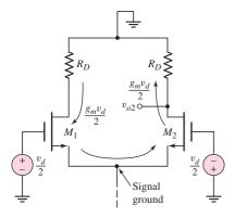
Figure 11.22 AC equivalent circuit, MOSFET differential amplifier
