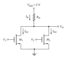
Figure 3.46 A two-input NMOS NOR logic gate
