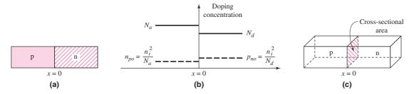
Figure 1.10 (a) The pn junction: (a) simplified one-dimensional geometry, (b) doping profile of an ideal uniformly doped pn junction, and (c) three-dimensional representation showing the cross-sectional area
