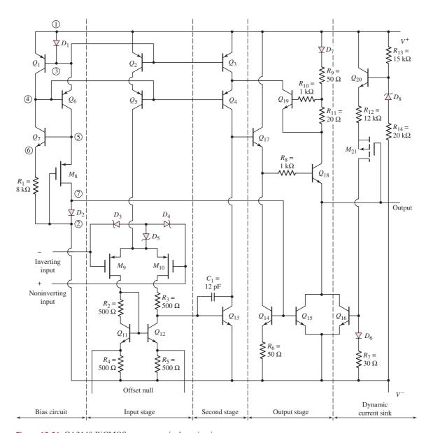
Figure 13.21 CA3140 BiCMOS op-amp equivalent circuit
