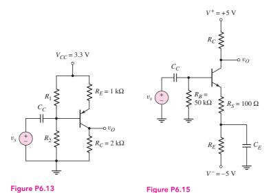
D6.15 For the circuit in Figure P6.15, the transistor parameters are  $\beta = 100$  and  $V_A = \infty$ . Design the circuit such that  $I_{CQ} = 0.25$  mA and  $V_{CEQ} = 3$  V.
