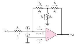
Figure 9.12 Inverting op-amp with T-network
