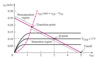
Figure 3.31 Transistor characteristics,  $v_{DS}$ (sat) curve, load line, and Q-point for the NMOS common-source circuit in Figure 3.25(b)
