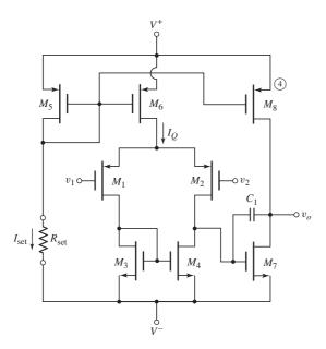
Figure 13.14 MC14573 CMOS op-amp equivalent circuit
