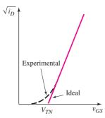
Figure 3.23 Plot of  $\sqrt{i_D}$  versus  $v_{GS}$  for a MOSFET biased in the saturation region showing subthreshold conduction. Experimentally, a subthreshold current exists even for  $v_{GS} < V_{TN}$ .
