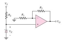
Figure 9.41 Simple op-amp voltage reference circuit
