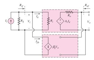
Figure 12.14 Ideal shunt-shunt feedback topology
