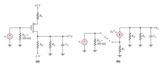
Figure 7.25 (a) MOSFET common-source circuit with a load capacitor and (b) small-signal equivalent circuit
