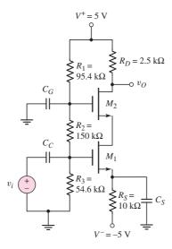
Figure 4.51 NMOS cascode circuit
