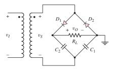
Figure 2.14 A voltage doubler circuit
