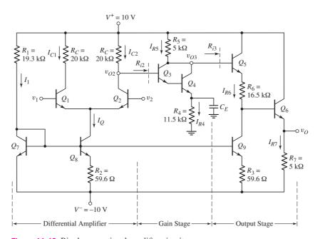
Figure 11.49 Bipolar operational amplifier circuit
