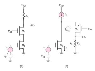
Figure 13.16 (a) Classical cascode stage. (b) folded-cascode stage
