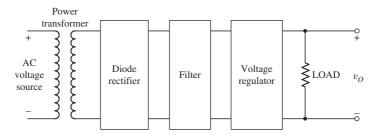
**Figure 2.1** Diagram of an electronic power supply. The circuits that characterize each block diagram are considered in this chapter.
