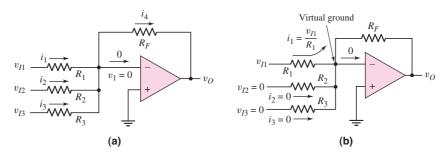
Figure 9.14 (a) Summing op-amp amplifier circuit and (b) currents and voltages in the summing amplifier
