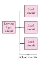
**Figure 16.17** Logic circuit driving *N* load circuits
