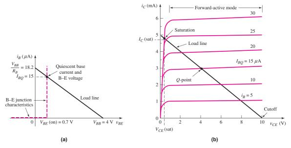
Figure 5.23 (a) Base–emitter junction piecewise linear i–v characteristics and the input load line, and (b) common-emitter transistor characteristics and the collector–emitter load line showing the Q-point for the circuit shown in Example 5.3 (Figure 5.20)
