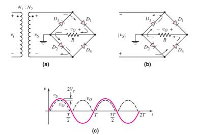
Figure 2.6 A full-wave bridge rectifier: (a) circuit showing the current direction for a positive input cycle, (b) current direction for a negative input cycle, and (c) input and output voltage waveforms
