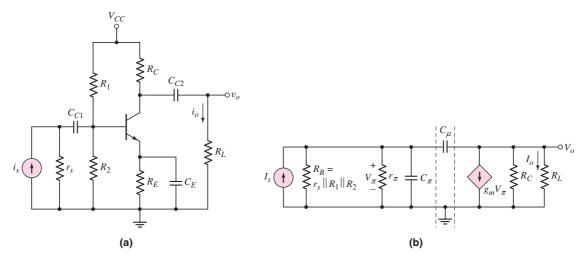
Figure 7.41 (a) Common-emitter circuit with current source input; (b) small-signal equivalent circuit with simplified hybrid- $\pi$  model
