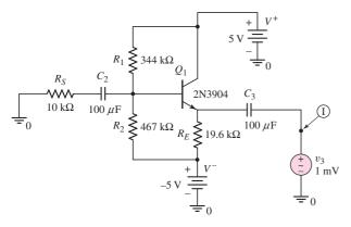
Figure 6.56 PSpice circuit schematic for Example 6.14
