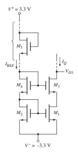
Figure 10.42 MOSFET cascode current source circuit for design application
