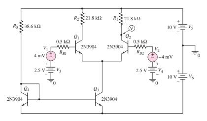
Figure 11.11 Circuit used in the computer simulation of Design Example 11.4
