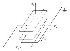
Figure 11.10 Experimental arrangement for measuring Hall voltage
