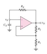
Figure 15.35 Schmitt trigger oscillator
