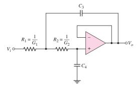
Figure 15.6 General two-pole low-pass filter
