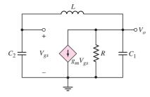
Figure 15.20 Small-signal equivalent circuit, MOSFET Colpitts oscillator
