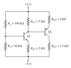
Figure 5.61 A multistage transistor circuit
