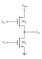
Figure 3.41 Example of CMOS inverter
