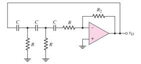
Figure 15.16 Phase-shift oscillator circuit
