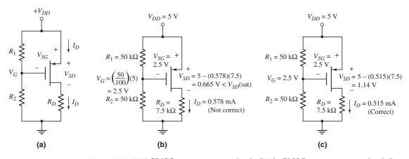
Figure 3.26 (a) A PMOS common-source circuit, (b) the PMOS common-source circuit for Example 3.4 showing current and voltage values when the saturation-region bias assumption is incorrect, and (c) the circuit for Example 3.4 showing current and voltage values when the nonsaturation-region bias assumption is correct
