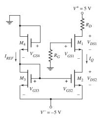
Figure 3.50 Implementation of a MOSFET constant-current source
