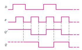
Figure 16.66 CMOS master-slave D flip-flop
