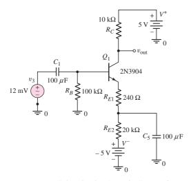
Figure 6.37 PSpice circuit schematic diagram for Example 6.7
