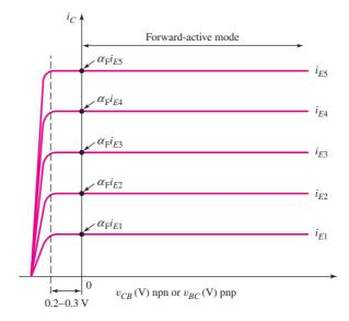
Figure 5.12 Transistor current-voltage characteristics of the common-base circuit
