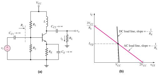
Figure 8.28 (a) Inductively coupled class-A amplifier and (b) dc and ac load lines
