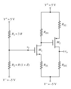
Figure 4.60 Two-stage MOSFET amplifier for design application
