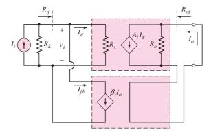
Figure 12.9 Ideal shunt-series feedback topology
