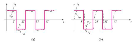
Figure 7.20 Steady-state output response for a square-wave input response for (a) circuit in Figure 7.16 (coupling capacitor) and a large time constant, and (b) circuit in Figure 7.18 (load capacitor) and a short time constant
