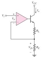
Figure 12.27 Example of an op-amp series–series feedback circuit
