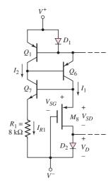
Figure 13.22 Bias circuit, CA3140 BiCMOS op-amp
