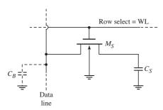
Figure 16.81 One-transistor dynamic RAM cell
