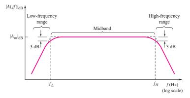
Figure 7.1 Amplifier gain versus frequency
