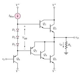
Figure 8.36 Class-AB output stage with Darlington pairs
