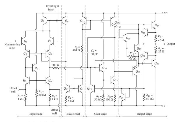
Figure 13.3 Equivalent circuit, 741 op-amp
