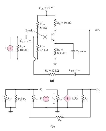
Figure 12.44 (a) Feedback circuit prior to breaking the loop and (b) small-signal equivalent circuit after breaking the loop
