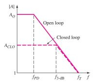
Figure 14.10 Bode plot, open-loop and closed-loop gain magnitude
