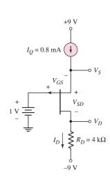
Figure 3.63 A p-channel JFET circuit biased with a constant-current source
