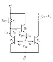
Figure 10.5 Basic three-transistor current source
