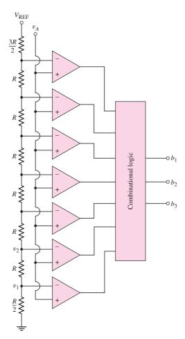
Figure 16.93 A 3-bit flash or parallel A/D converter
