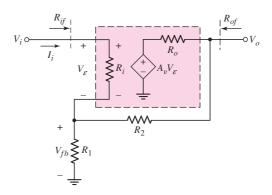
Figure 12.17 Equivalent circuit, op-amp series—shunt feedback configuration
