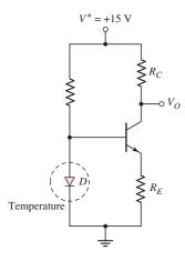
Figure 5.64 Design application circuit to measure output voltage of diode versus temperature
