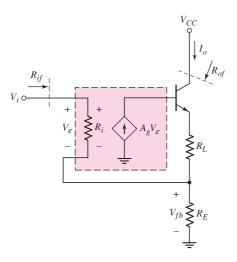
Figure 12.28 Equivalent circuit, op-amp series-series feedback configuration
