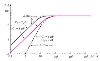
Figure 7.31 PSpice results for each coupling capacitor, and the combined effect for the circuit in Figure 7.30 ( $C_E \rightarrow \infty$ )
