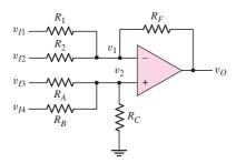
Figure 9.40 Generalized op-amp summing amplifier
