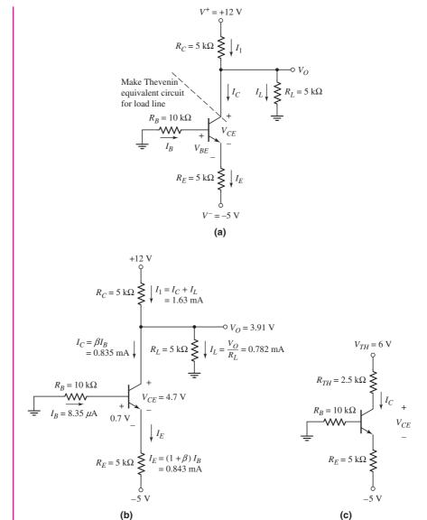
Figure 5.38 Circuit for Example 5.10: (a) circuit; (b) circuit showing current and voltage values; and (c) Thevenin equivalent circuit
