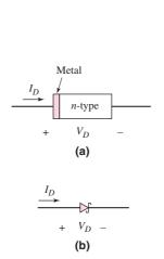
Figure 1.41 Schottky barrier diode: (a) simplified geometry and (b) circuit symbol
