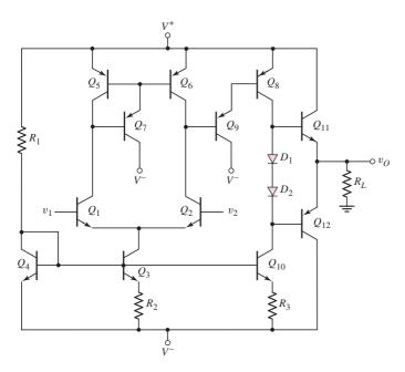
Figure 13.2 A simple bipolar operational amplifier
