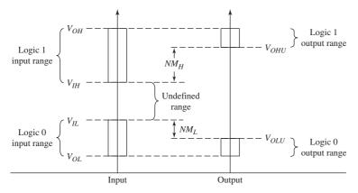
Figure PR3.5 Voltage ranges representing logic 1 and logic 0, and definition of noise margins
