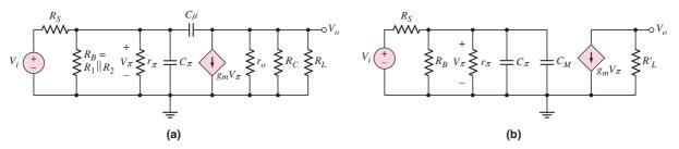
Figure 7.57 (a) High-frequency equivalent circuit of common-emitter amplifier; (b) high-frequency equivalent circuit of common-emitter amplifier, including the Miller capacitance
