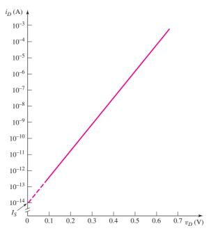
Figure 1.18 Ideal forward-biased I-V characteristics of a pn junction diode, with the current plotted an a log scale for  $I_S = 10^{-14}$  A and n = 1. The diode current increases approximately one order of magnitude for every 60-mV increase in diode voltage.
