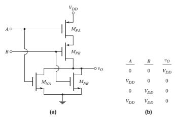
Figure 16.33 (a) Two-input CMOS NOR logic circuit and (b) truth table
