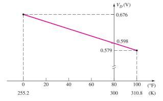
Figure 1.48 Diode voltage versus temperature
