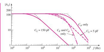
Figure 7.67 PSpice analysis results for cascode circuit
