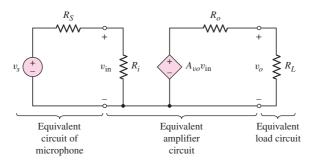
Figure 6.25 Equivalent preamplifier circuit
