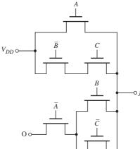
Figure 16.55 NMOS pass logic network with complementary function in parallel
