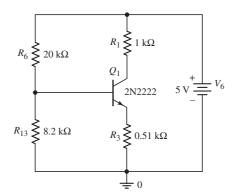
Figure 5.56 PSpice circuit schematic for Design Example 5.16
