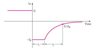
Figure 1.25 Current characteristics versus time during diode switching
