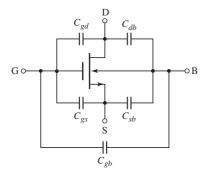
Figure 16.2 n-channel MOSFET and device capacitances
