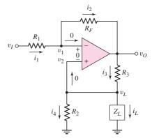
Figure 9.21 Simple voltage-to-current converter
