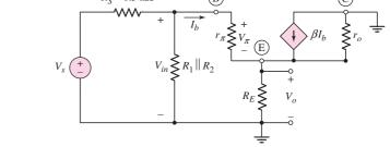
Figure 6.49 Emitter-follower circuit. Output signal is at the emitter terminal with respect to ground.
