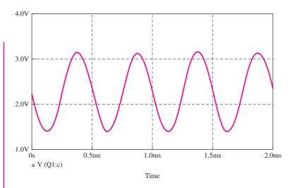
Figure 5.49 Output signal from the circuit shown in Figure 5.48 for input signals of  $V_{BB}=1.3 \text{ V}$  and  $\Delta v_I=0.2 \sin \omega t$  (V)
