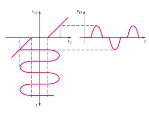
**Figure 8.21** Crossover distortion of basic complementary push–pull output stage
