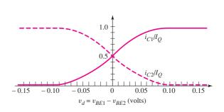
Figure 17.2 Normalized dc transfer characteristics, BJT differential amplifier
