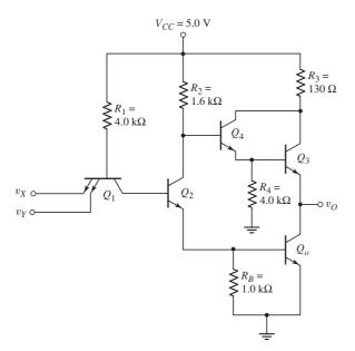
Figure 17.27 TTL circuit with modified totem-pole output stage
