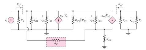
Figure 12.25 Small-signal equivalent circuit of circuit in Figure 12.24(a)
