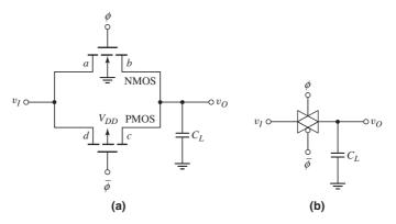
Figure 16.56 (a) CMOS transmission gate and (b) simplified circuit symbol
