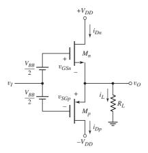
Figure 8.26 MOSFET class-AB output stage
