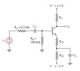
Figure 6.36 A bipolar circuit with an emitter resistor and an emitter bypass capacitor
