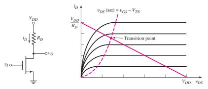
Figure 16.3 (a) NMOS inverter with resistor load and (b) transistor characteristics and load line
