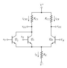
Figure 17.3 Basic two-input ECL OR/NOR logic circuit
