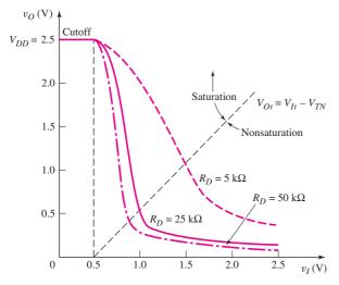
Figure 16.4 Voltage transfer characteristics of NMOS inverter with resistive load, using parameters from Example 16.1 and for the three resistor values.
