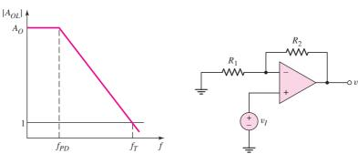
**Figure 14.8** Bode plot, open-loop gain magnitude
