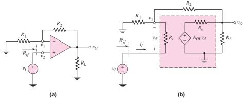
Figure 14.5 (a) Noninverting amplifier and (b) noninverting amplifier equivalent circuit, for calculating closed-loop input resistance
