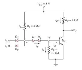
Figure 17.20 Basic diode-transistor logic gate
