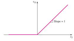
Figure 9.34 Voltage transfer characteristics of precision half-wave rectifier
