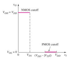
Figure 16.24 CMOS inverter output voltage for input voltage in either high state or low state
