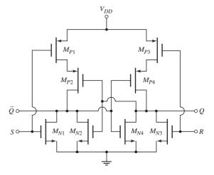
Figure 16.64 CMOS R-S flip-flop
