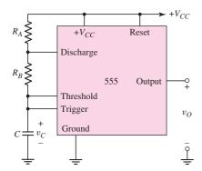
Figure 15.41 Astable multivibrator 555 circuit
