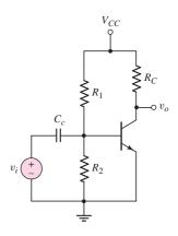
Figure 10.28 Bipolar common-emitter circuit
