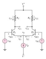
Figure 11.2 Basic BJT differential-pair configuration
