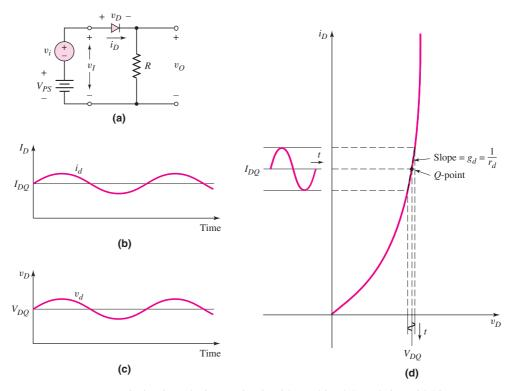
Figure 1.35 AC circuit analysis: (a) circuit with combined dc and sinusoidal input voltages, (b) sinusoidal diode current superimposed on the quiescent current, (c) sinusoidal diode voltage superimposed on the quiescent value, and (d) forward-biased diode I-V characteristics with a sinusoidal current and voltage superimposed on the quiescent values
