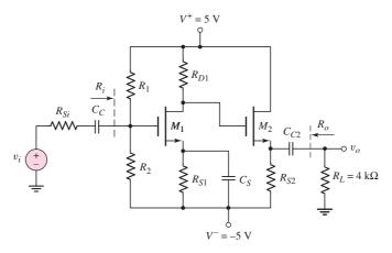
Figure 3.52 Common-source amplifier in cascade with source follower
