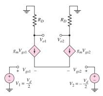
Figure 11.26 Small-signal equivalent circuit, JFET differential amplifier
