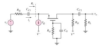
Figure 4.32 Common-gate circuit
