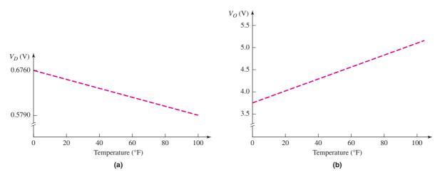
Figure 3.70 (a) Diode voltage versus temperature and (b) circuit output voltage versus temperature
