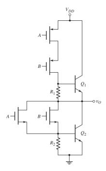
Figure 17.37 Two-input BiCMOS NOR circuit
