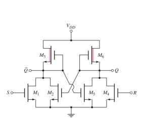
Figure 16.63 NMOS R-S flip-flop
