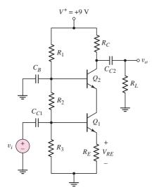
Figure 5.63 A bipolar cascode circuit for Example 5.20
