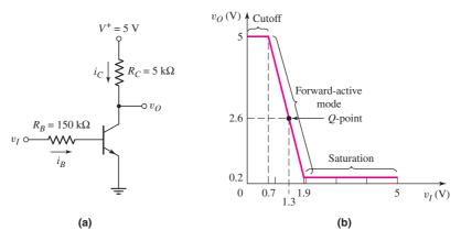
Figure 5.48 (a) A bipolar inverter used as an amplifier; (b) the inverter voltage transfer characteristics
