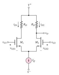
Figure 11.19 Basic MOSFET differential pair configuration
