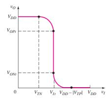
Figure 16.26 Complete voltage transfer characteristics, CMOS inverter
