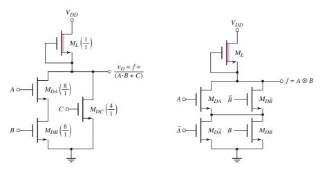
Figure 16.15 NMOS logic circuit example
