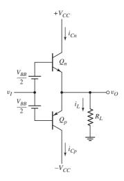
Figure 8.24 Bipolar class-AB output stage
