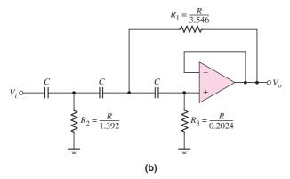
Figure 15.9 (a) Three-pole low-pass Butterworth filter and (b) three-pole high-pass Butterworth filter
