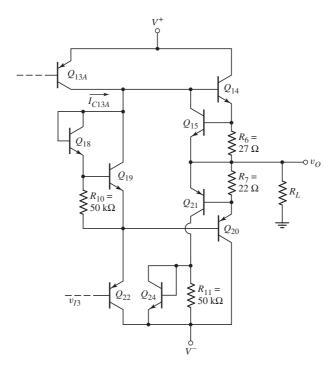
Figure 13.9 Output stage, 741 op-amp with short-circuit protection devices
