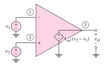
Figure 9.2 Ideal op-amp equivalent circuit
