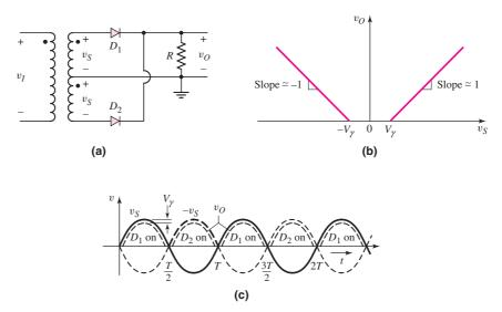
Figure 2.5 Full-wave rectifier: (a) circuit with center-tapped transformer, (b) voltage transfer characteristics, and (c) input and output waveforms
