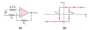
Figure 15.29 (a) Noninverting Schmitt trigger circuit and (b) voltage transfer characteristics
