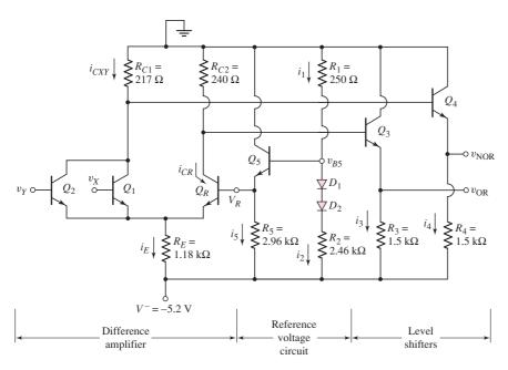
Figure 17.5 Basic ECL logic gate with reference circuit
