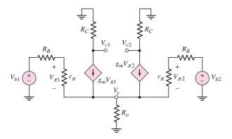
Figure 11.9 Small-signal equivalent circuit, bipolar differential amplifier
