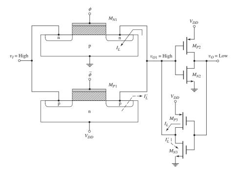
Figure 16.65 CMOS D-type flip-flop
