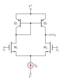
Figure 11.44 Basic BiCMOS differential amplifier
