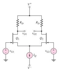
Figure 11.25 Basic JFET differential pair configuration
