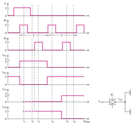
Figure 16.61 NMOS shift register voltages at various times
