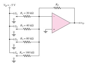
Figure 16.90 A 4-bit weighted-resistor D/A converter
