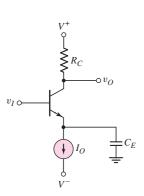
Figure 10.1 Bipolar circuit with ideal current-source biasing
