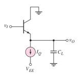
Figure 17.18 Emitterfollower stage with load capacitance
