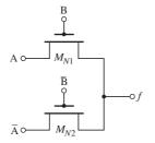
Figure 16.52 Simple NMOS pass logic network
