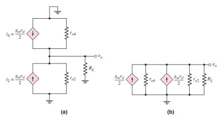
Figure 11.31 (a) Small-signal equivalent circuit BJT differential amplifier with active load and (b) rearrangement of small-signal equivalent circuit
