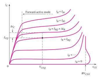
Figure 5.18 Common-emitter characteristics showing breakdown effects
