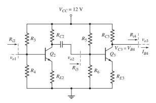
Figure 6.79 Gain stage (two-stage common-emitter amplifier) for design application
