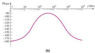
Figure 7.29 PSpice analysis results for the circuit with an emitter bypass capacitor: (a) voltage gain magnitude response and (b) phase response
