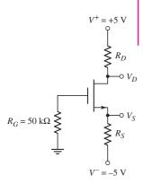
Figure 3.27 Circuit configuration for Example 3.5
