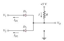
Figure 2.42 A two-input diode AND logic circuit
