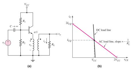
Figure 8.30 (a) Transformer-coupled emitter-follower amplifier and (b) dc and ac load lines
