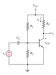
Figure 6.73 Simple common-emitter amplifier for power calculations
