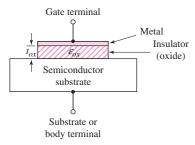
Figure 3.1 The basic MOS capacitor structure
