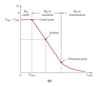
**Figure 4.39** (a) NMOS amplifier with enhancement load device; (b) driver transistor characteristics and enhancement load curve with transition point; and (c) voltage transfer characteristics of NMOS amplifier with enhancement load device
