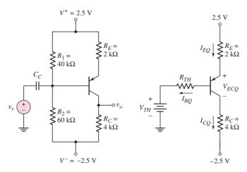
Figure 6.32 (a) pnp transistor circuit for Example 6.6 and (b) Thevenin equivalent circuit for Example 6.6
