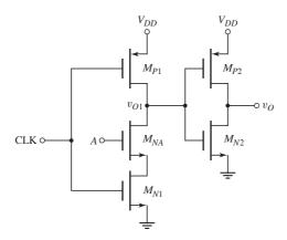
Figure 16.43 Simple clocked CMOS logic circuit
