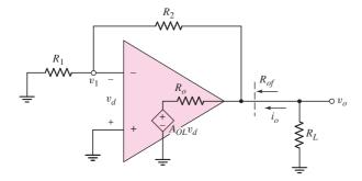
Figure 14.6 Equivalent circuit for calculating closed-loop output resistance
