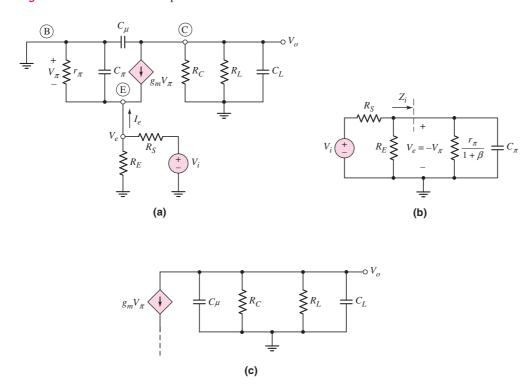
Figure 7.62 (a) High-frequency common-base equivalent circuit, (b) equivalent input circuit, and (c) equivalent output circuit
