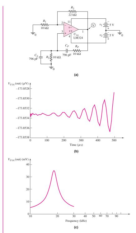
Figure 15.18 (a) Circuit used in the computer simulation for Example 15.5, (b) output voltage versus time, and (c) output voltage versus input frequency
