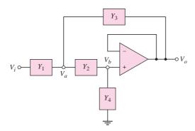
Figure 15.5 General two-pole active filter
