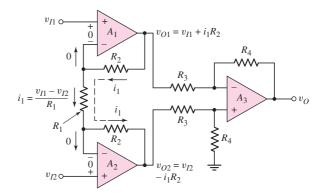
Figure 9.26 Instrumentation amplifier
