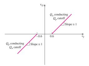
Figure 8.20 Voltage transfer characteristics of basic complementary push–pull output stage
