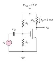
Figure 4.17 Common-source NMOS transistor circuit
