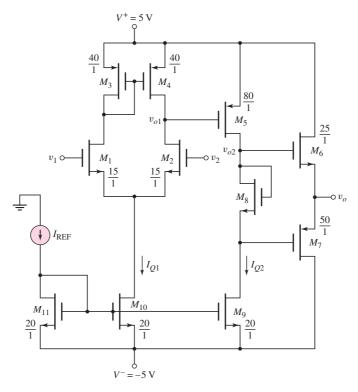
Figure 13.15 A three-stage CMOS operational amplifier
