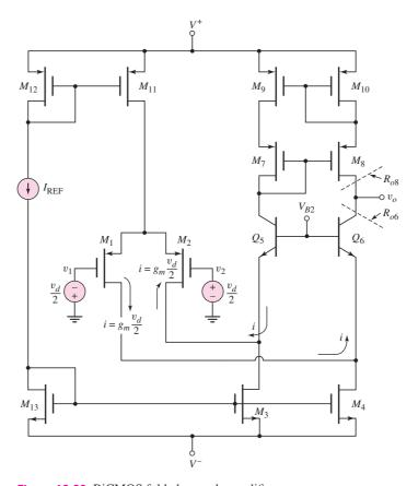
Figure 13.20 BiCMOS folded cascode amplifier
