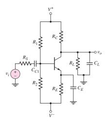
Figure 7.56 Common-emitter amplifier
