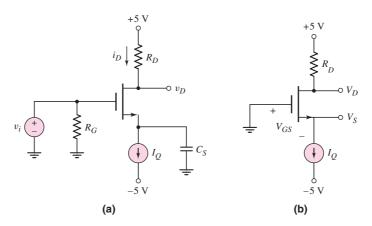
Figure 3.32 (a) NMOS common-source circuit biased with a constant-current source and (b) equivalent dc circuit
