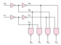
Figure 16.72 Simplified decoder with two-bit input
