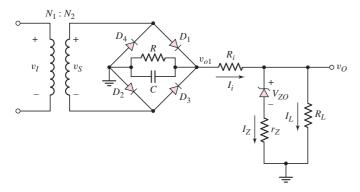
Figure 2.48 DC power supply circuit for design application
