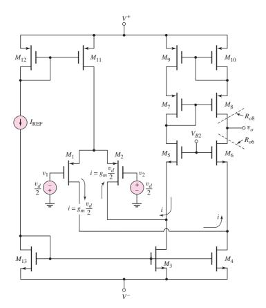
Figure 13.17 CMOS folded cascode amplifier
