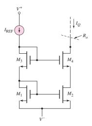
Figure 11.24 MOSFET cascode current source
