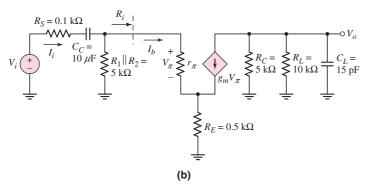
Figure 7.26 (a) Circuit with both a coupling and a load capacitor and (b) small-signal equivalent circuit
