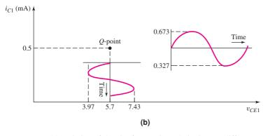
Figure 11.4 (a) Variation of Q-point for transistor  $Q_1$  in the BJT diff-amp as the common-mode input voltage varies from +5 to -9.3 V; (b) change in collector current and collector–emitter voltage versus time for transistor  $Q_1$  in the BJT diff-amp when a sinusoidal 18 mV differential voltage is applied
