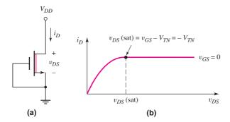
Figure 3.38 (a) Depletion-mode NMOS device with the gate connected to the source and (b) current–voltage characteristics
