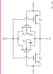
16.76 What is the logic function implemented by the circuit in Figure P16.76?
