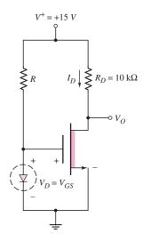
Figure 3.69 Design application circuit to measure output voltage of diode versus temperature
