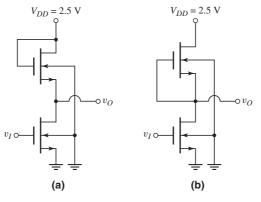
Figure 16.9 NMOS inverters, showing substrate connections to ground potential: (a) enhancement-load inverter and (b) depletion-load inverter
