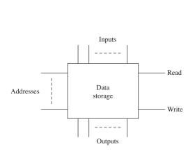
Figure 16.70 Schematic of a basic memory configuration
