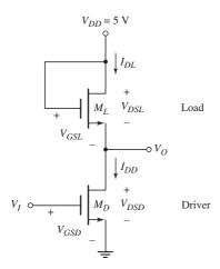
Figure 3.36 Circuit with enhancement-load device and NMOS driver
