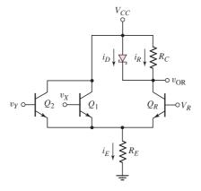
Figure 17.10 Modified ECL logic gate with Schottky diode
