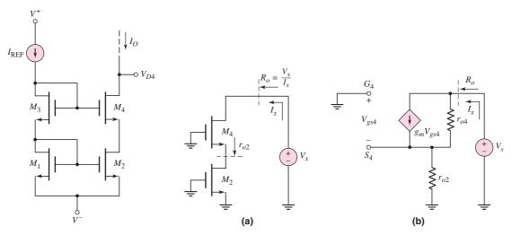
Figure 10.18 MOSFET cascode current mirror
