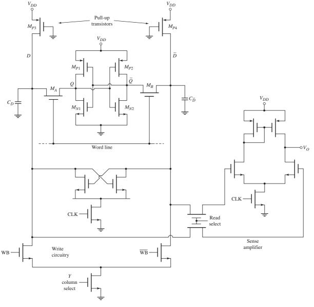
Figure 16.79 Complete circuit diagram of a CMOS RAM cell with write and read circuitry
