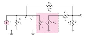
Figure 12.21 Equivalent circuit, op-amp shunt-series feedback configuration
