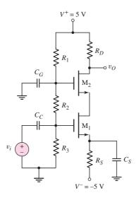
Figure 3.53 NMOS cascode circuit
