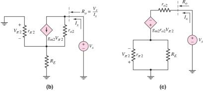
Figure 10.11 (a) Small-signal equivalent circuit for determining output resistance of Widlar current source, (b) simplified equivalent circuit for determining output resistance, and (c) equivalent circuit after a Norton transformation
