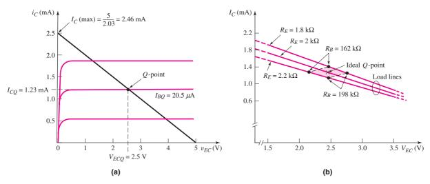
Figure 5.37 (a) Load line and *Q*-point value for the ideal designed circuit shown in Figure 5.36 used in Example 5.9; (b) load lines and *Q*-point values for the extreme tolerance values of resistors
