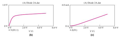
Figure 1.34 (a) PSpice circuit schematic, (b) diode voltage, and (c) diode current for Example 1.10
