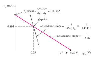
Figure 6.44 Plots of dc and ac load lines for Example 6.9
