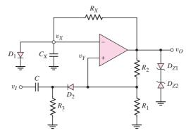
Figure 15.37 Schmitt trigger monostable multivibrator
