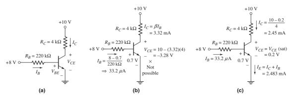
Figure 5.24 Circuit for Example 5.5: (a) circuit; (b) circuit showing current and voltage values, assuming the transistor is biased in the forward-active mode (an incorrect assumption); and (c) circuit showing current and voltage values, assuming the transistor is biased in the saturation mode (correct assumption)
