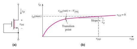
Flgure 4.42 (a) NMOS depletion-mode transistor with gate and source connected in a load device configuration and (b) current–voltage characteristic of NMOS depletion load transistor
