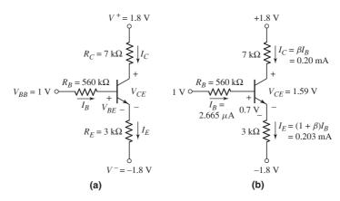
Figure 5.30 Circuit for Example 5.7: (a) circuit and (b) circuit showing current and voltage values
