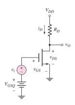
Figure 4.1 NMOS commonsource circuit with timevarying signal source in series with gate dc source
