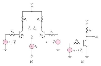
Figure 11.50 (a) BJT differential amplifier with differential-mode input signal and (b) equivalent common-emitter half-circuit of differential amplifier
