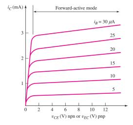
Figure 5.13 Transistor current-voltage characteristics of the common-emitter circuit
