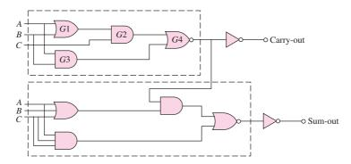
Figure 16.68 Gate configuration of the one-bit full adder
