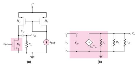
Figure 10.40 (a) Simple MOSFET amplifier with active load and load resistance and (b) small-signal equivalent circuit
