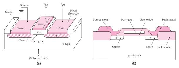
Figure 3.5 (a) Schematic diagram of an n-channel enhancement-mode MOSFET and (b) an n-channel MOSFET, showing the field oxide and polysilicon gate
