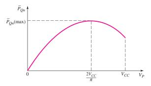
Figure 8.23 Average power dissipation in each transistor versus peak output voltage for class-B output stage
