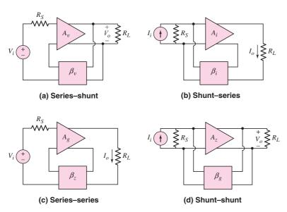
Figure 12.5 Basic feedback connections
