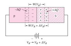
Figure 1.14 Increase in space-charge width with an increase in reverse bias voltage from  $V_R$  to  $V_R + \Delta V_R$ . Creation of additional charges  $+\Delta Q$  and  $-\Delta Q$  leads to a junction capacitance.
