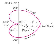
Figure 12.54 Nyquist plot, loop gain for two-stage amplifier
