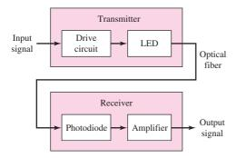
Figure 1.40 Basic elements in an optical transmission system
