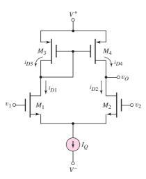
Figure 11.32 MOSFET differential amplifier with active load
