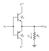
Figure 8.19 Basic complementary push–pull output stage
