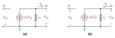
Figure 4.11 Small signal equivalent circuit of a p-channel MOSFET showing (a) the conventional voltage polarities and current directions and (b) the case when the voltage polarities and current directions are reversed.
