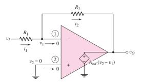
Figure 9.9 Inverting op-amp equivalent circuit
