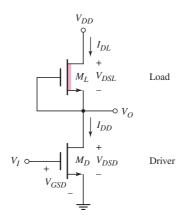
Figure 3.39 Circuit with depletion-load device and NMOS driver
