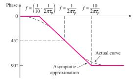
Figure 7.9 Bode plot of the voltage transfer function phase for the circuit in Figure 7.3
