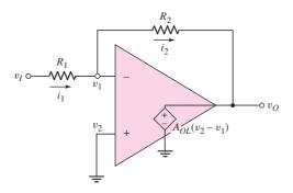
Figure 14.2 Equivalent circuit, inverting amplifier with finite open-loop gain
