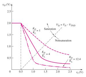
Figure 16.6 Voltage transfer characteristics of NMOS inverter with saturated load, using parameters from Example 16.2 and for three aspect ratios.
