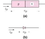
Figure 1.19 The basic pn junction diode: (a) simplified geometry and (b) circuit symbol, and conventional current direction and voltage polarity
