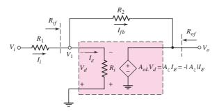
Figure 12.34 Equivalent circuit, op-amp shunt-shunt feedback configuration
