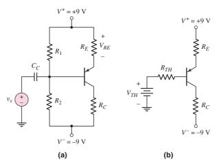
Figure 5.57 (a) Circuit for Example 5.17 and (b) Thevenin equivalent circuit
