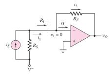
Figure 9.20 Current-to-voltage converter
