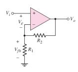
Figure 12.16 Example of an op-amp series—shunt feedback circuit
