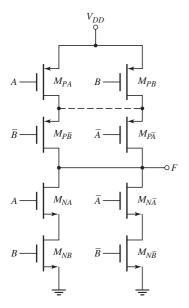
Figure 16.41 A CMOS static exclusive-OR logic gate
