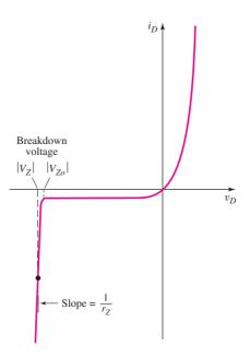
Figure 1.43 Diode *I–V* characteristics showing breakdown effects
