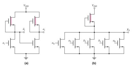
Figure 16.73 (a) Input buffer-inverter pair; (b) five-input NOR logic address decoder
