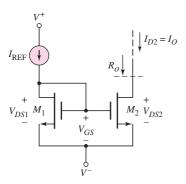
Figure 10.16 Basic two-transistor MOSFET current source
