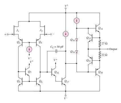
Figure 13.24 Equivalent circuit, LH0022/42/52 series hybrid JFET op-amp
