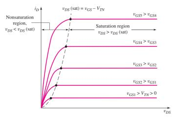
Figure 3.10 Family of  $i_D$  versus  $v_{DS}$  curves for an n-channel enhancement-mode MOSFET. Note that the  $v_{DS}$ (sat) voltage is a single point on each of the curves. This point denotes the transition between the nonsaturation region and the saturation region
