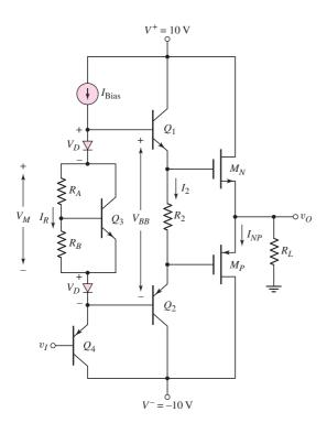
Figure 8.38 Output stage for design application
