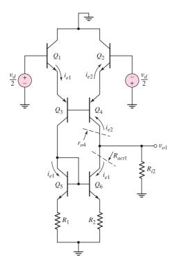
Figure 13.10 Simplified ac equivalent circuit of input stage of 741 op-amp
