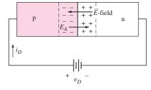
Figure 1.15 A pn junction with an applied forward-bias voltage showing the direction of the electric field induced by  $V_D$  and the direction of the original space-charge electric field. The two electric fields are in opposite directions resulting in a smaller net electric field and a smaller barrier between the p- and n-regions. The net electric field is always from the n- to the p-region.
