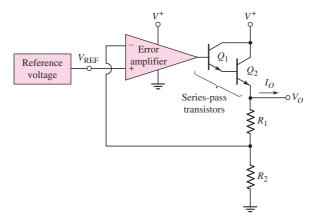
Figure 15.49 Basic series-pass voltage regulator
