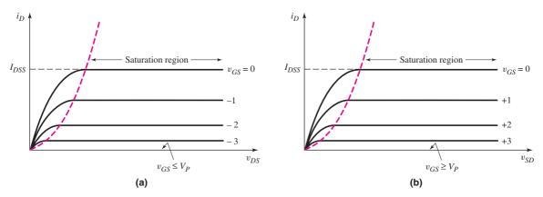
Figure 3.60 Current-voltage characteristics for: (a) n-channel JFET and (b) p-channel JFET
