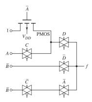
Figure 16.59 CMOS pass logic network
