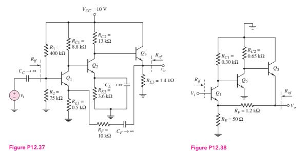
\*12.38 The circuit shown in Figure P12.38 is an ac equivalent circuit of a feedback amplifier. The transistor parameters are  $h_{FE} = 100$  and  $V_A = \infty$ . The quiescent collector currents are  $I_{C1} = 14.3$  mA,  $I_{C2} = 4.62$  mA, and  $I_{C3} = 4.62$  mA, and  $I_{C3} = 4.62$  mA, and  $I_{C3} = 4.62$  mA.
