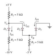
Figure 2.40 Diode circuit for Example 2.11
