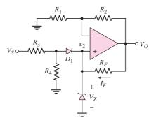
Figure 9.42 Op-amp voltage reference circuit
