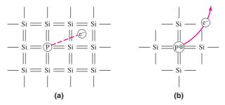
Figure 1.6 (a) Two-dimensional representation of a silicon lattice doped with a phosphorus atom showing the fifth phosphorus valence electron, (b) the resulting positively charged phosphorus ion after the fifth valence electron has moved into the conduction band
