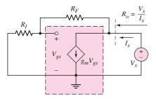
Figure 9.5 Equivalent circuit determining output resistance
