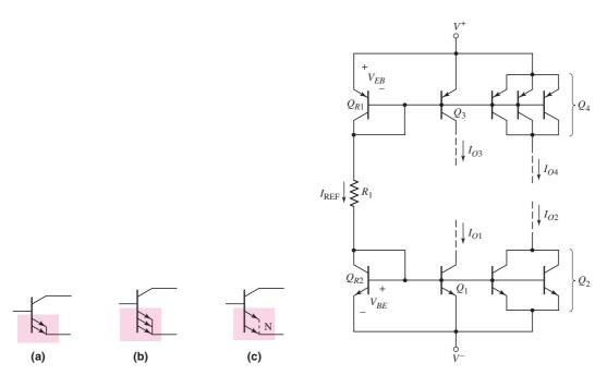
**Figure 10.14** Equivalent circuit symbols (a) two transistors in parallel, (b) three transistors in parallel, and (c) *N* transistors in parallel
