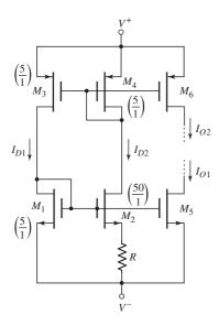
Figure 10.22 Bias-independent MOSFET current mirror
