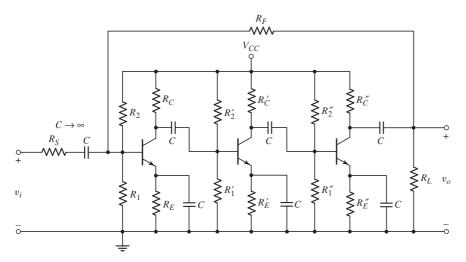
Figure 12.41 Example of multistage shunt-shunt feedback circuit
