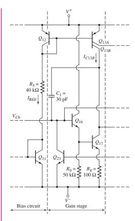
Figure 13.7 Reference circuit and gain stage, 741 op-amp
