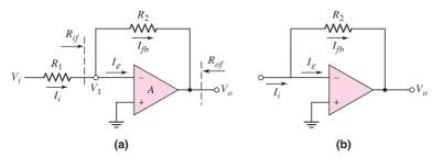
Figure 12.33 (a) The basic inverting op-amp circuit and (b) the circuit showing the shunt input connection
