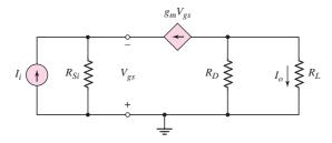
Flgure 4.34 Small-signal equivalent circuit of common-gate amplifier with a Norton equivalent signal source
