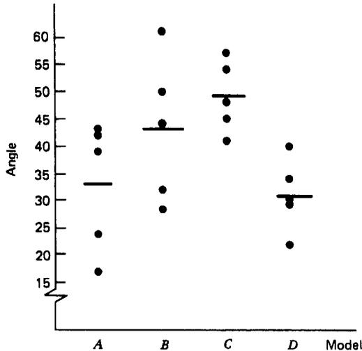
FIGURE 10.4. Angles of deflection for four types of chain saws.
